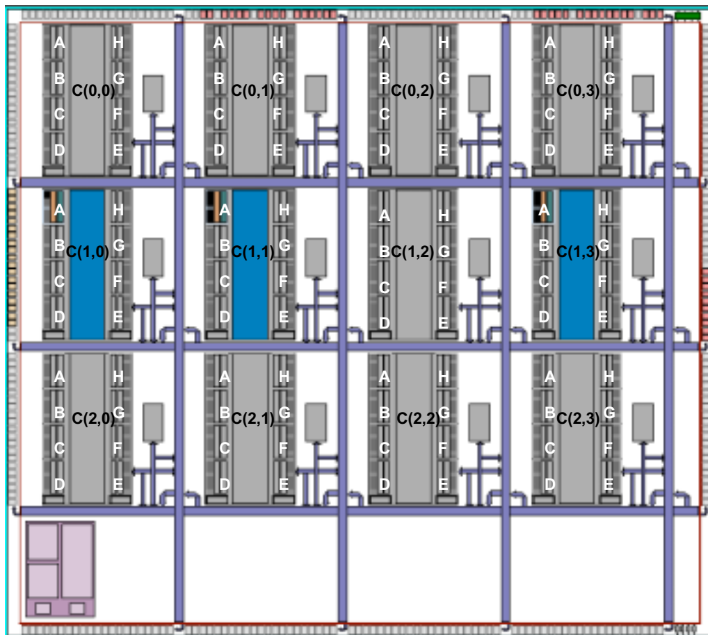
Figure 7. PSI2G100(S) logic block clusters and logic array block labels.
