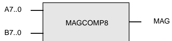
Figure 16. Block Diagram of an 8-Bit Magnitude Compare
