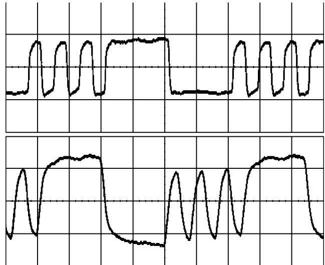
Figure 40. Thèvenin Bias, Direct-Coupled, with 93Ω Cable
