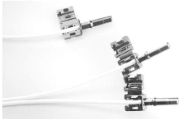
Figure 10. Fibers Inserted Into Connector Ferrules
