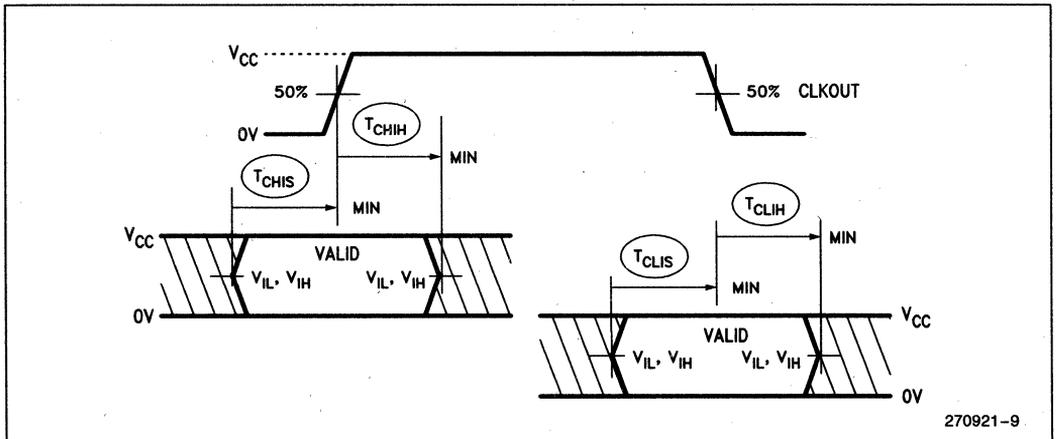
Figure 7. Input Setup and Hold
