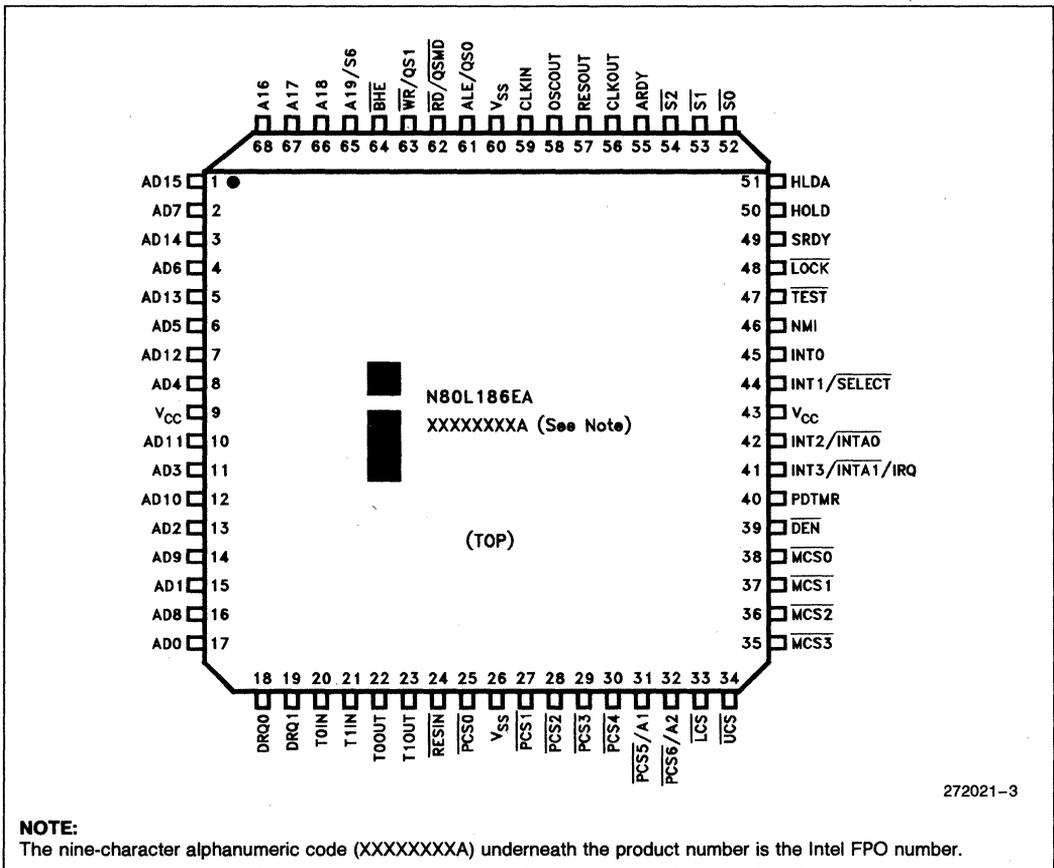
Figure 2. 68-Lead PLCC Pinout Diagram
