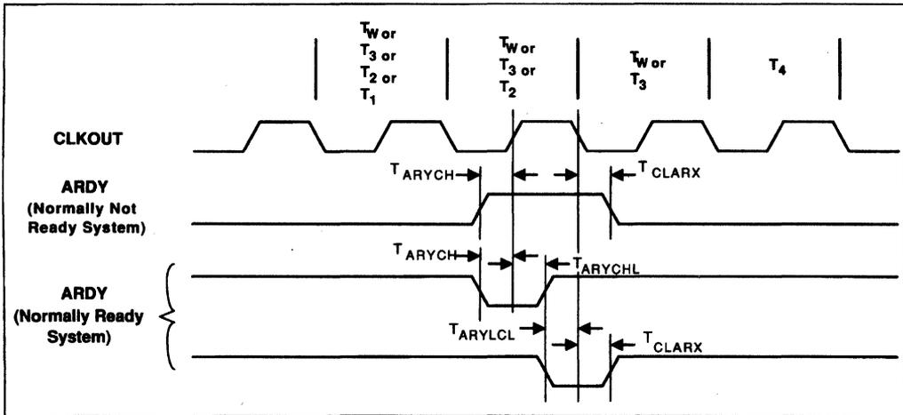
PERIPHERAL AND QUEUE STATUS WAVEFORMS
