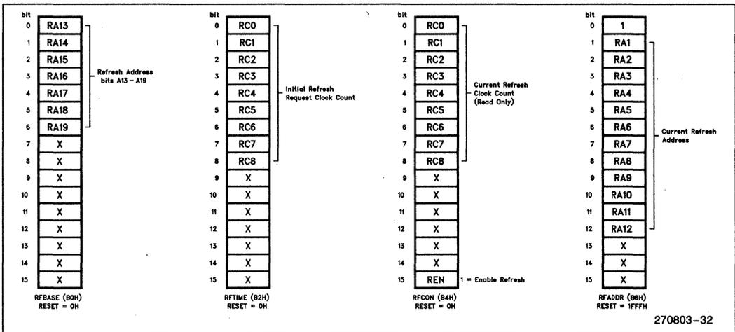
Figure 30. Refresh Control Unit Registers
