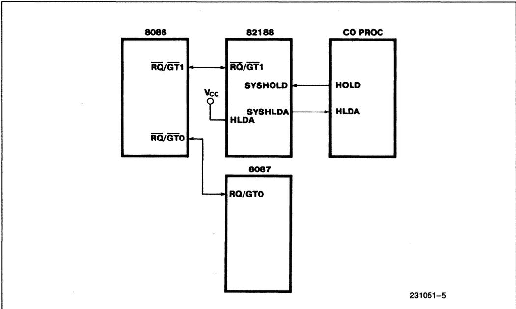
Figure 5. Bus Exchange Signal Connections (8086 Mode)
