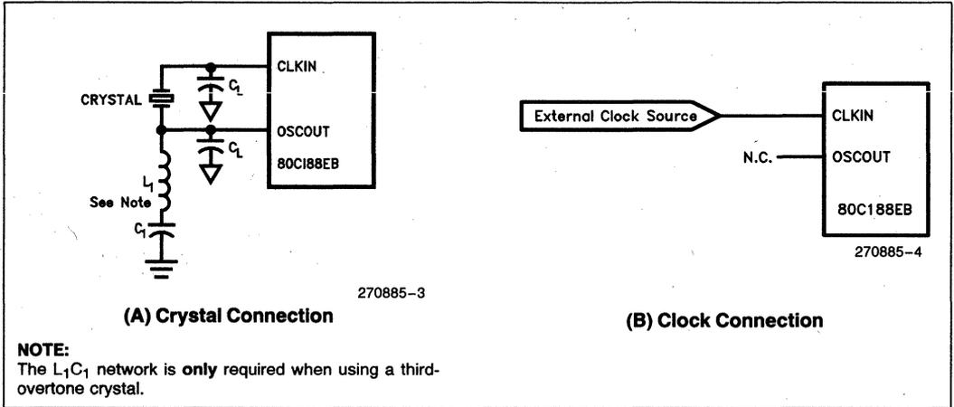
Figure 2. 80C188EB Clock Configurations
