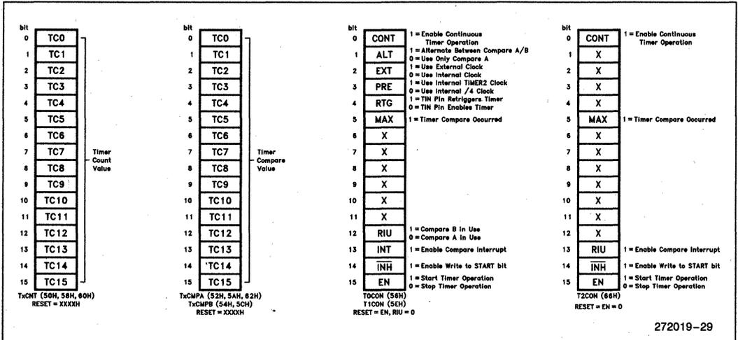
Figure 26. Timer Control Unit Registers
