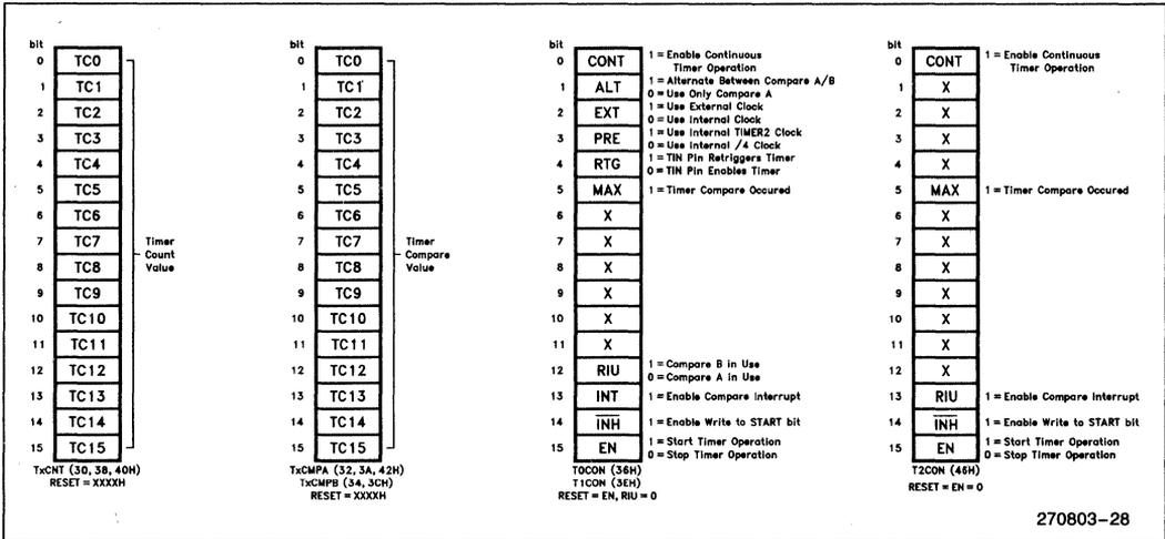
Figure 26. Timer Control Unit Registers
