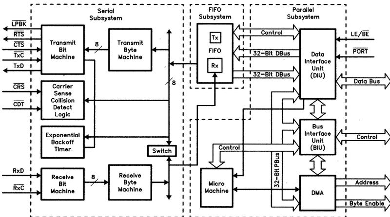
Figure 1. 82596DX/SX Block Diagram
