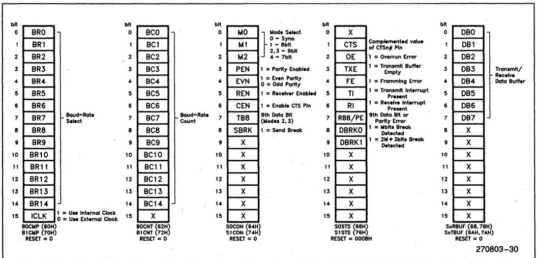
Figure 28. Serial Communications Unit Registers
