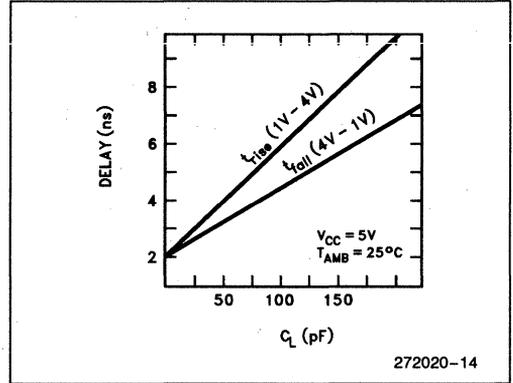
Figure 13. Typical Rise and Fall Variations Versus Load Capacitance
