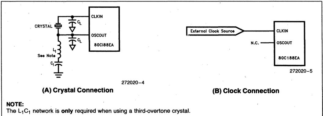
**Figure 2. 80C188EA Clock Configurations**
