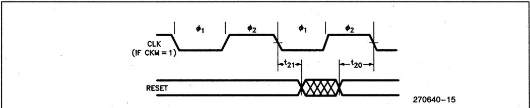
**CLK,  $\overline{\text{NPRD}}$ ,  $\overline{\text{NPWR}}$  TIMING (CKM = 1)**
