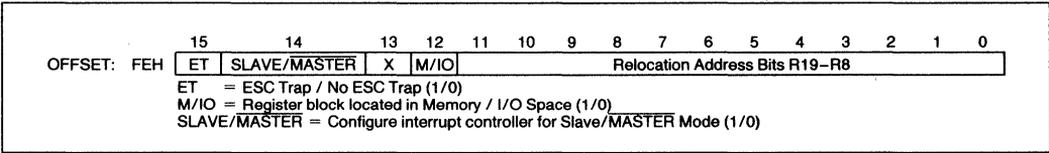
Figure 9. Relocation Register
