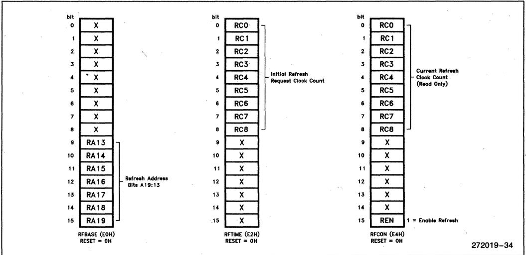
Figure 29. Refresh Control Unit Registers
