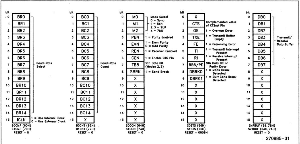
Figure 28. Serial Communications Unit Registers
