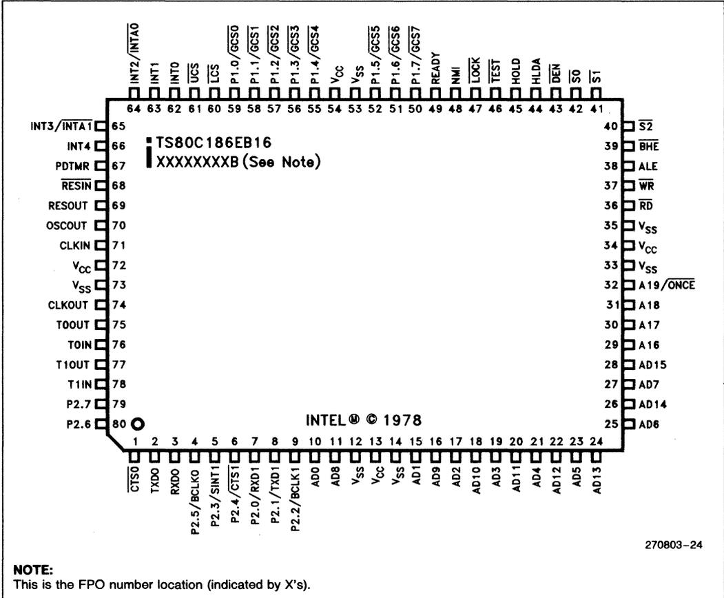
Figure 6. Quad Flat Pack Pinout Diagram
