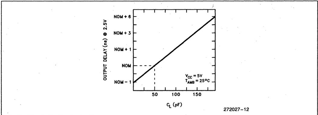
Figure 13. Typical Output Delay Variations versus Load Capacitance
