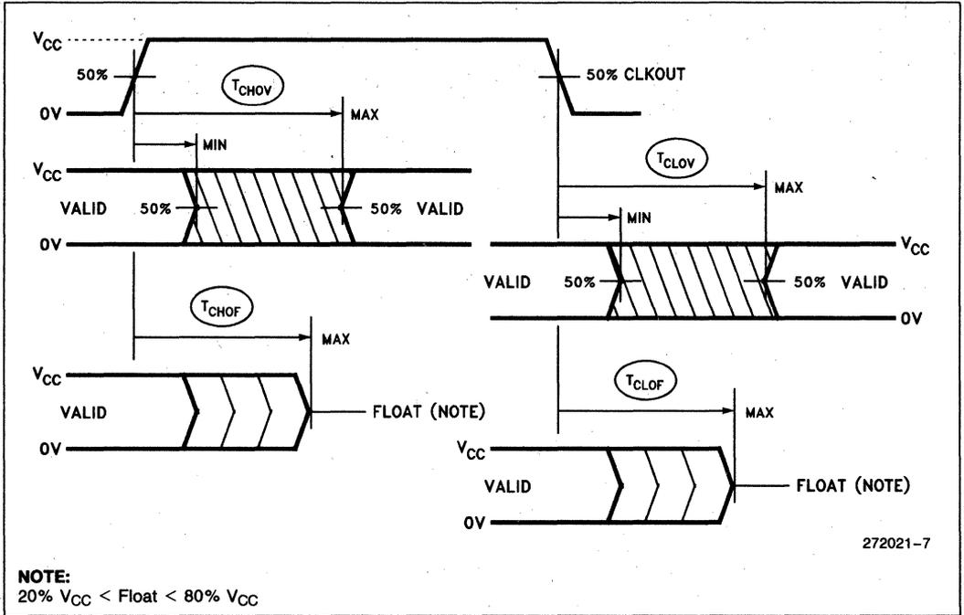
Figure 6. Output Delay and Float Waveform
