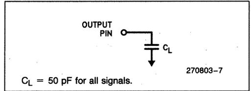
**Figure 7. AC Test Load**
