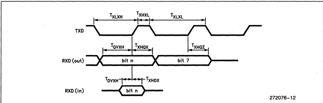
Figure 12. Serial Port Mode 0 Waveform
