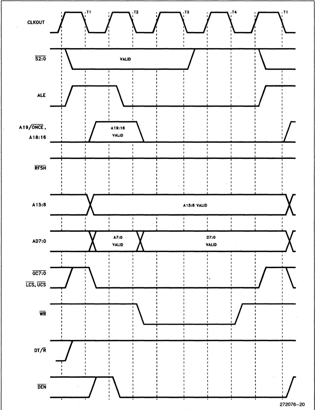
Figure 18. Memory Write and I/O Write Cycle Waveform
