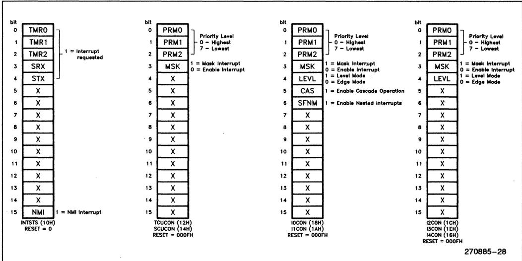
Figure 25. Interrupt Control Unit Registers
