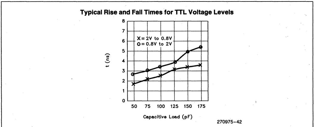
Figure 17. TTL Level Slew Rates for Output Buffers
