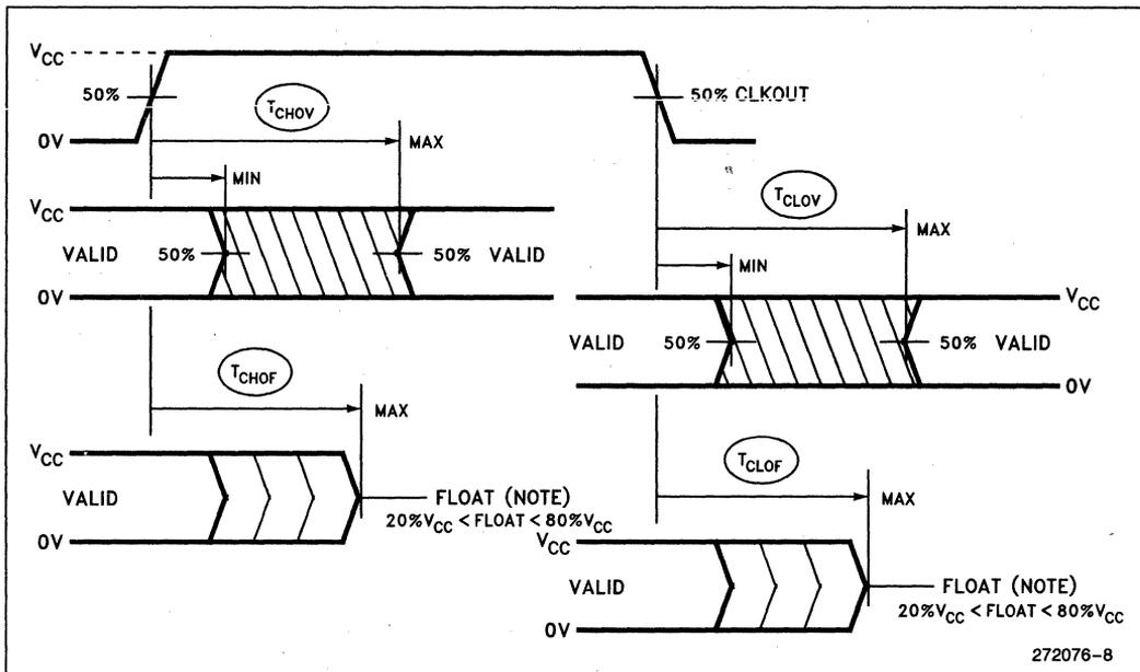
Figure 8. Output Delay and Float Waveforms
