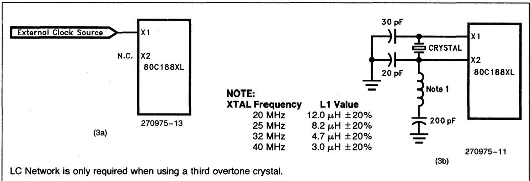
**Figure 3. 80C188XL Oscillator Configurations (see text)**
