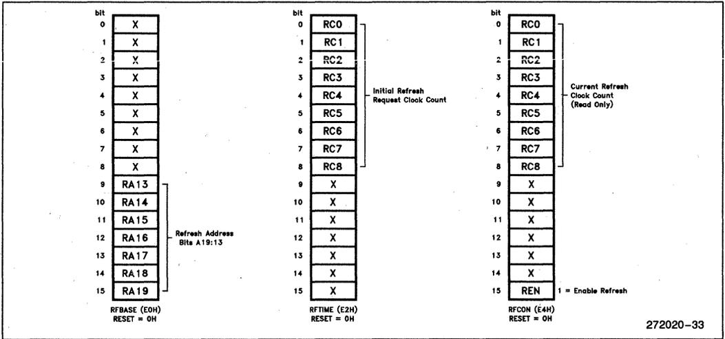
Figure 29. Refresh Control Unit Registers
