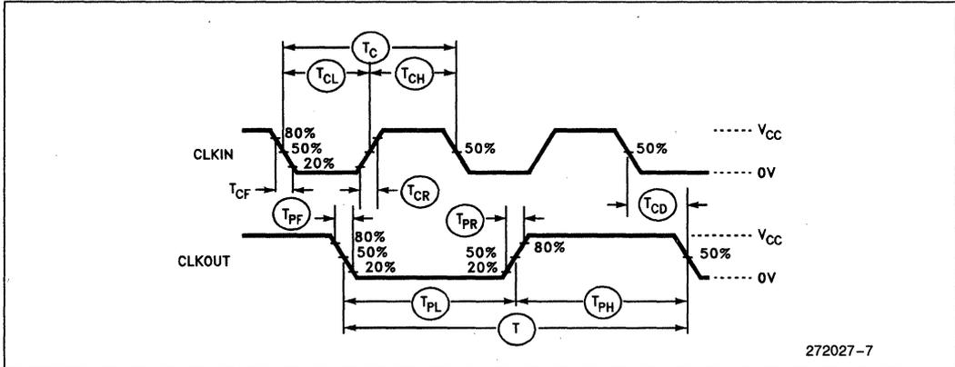
**Figure 7. Input and Output Clock Waveforms**
