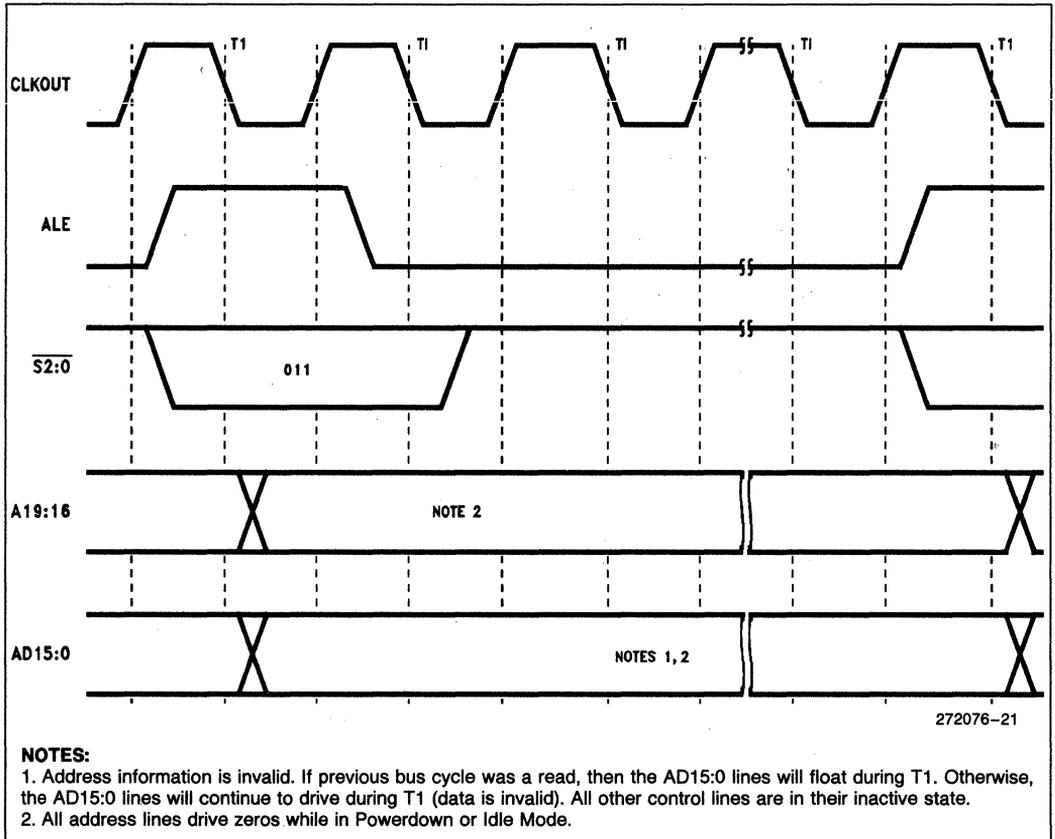
Figure 19. Halt Cycle Waveform
