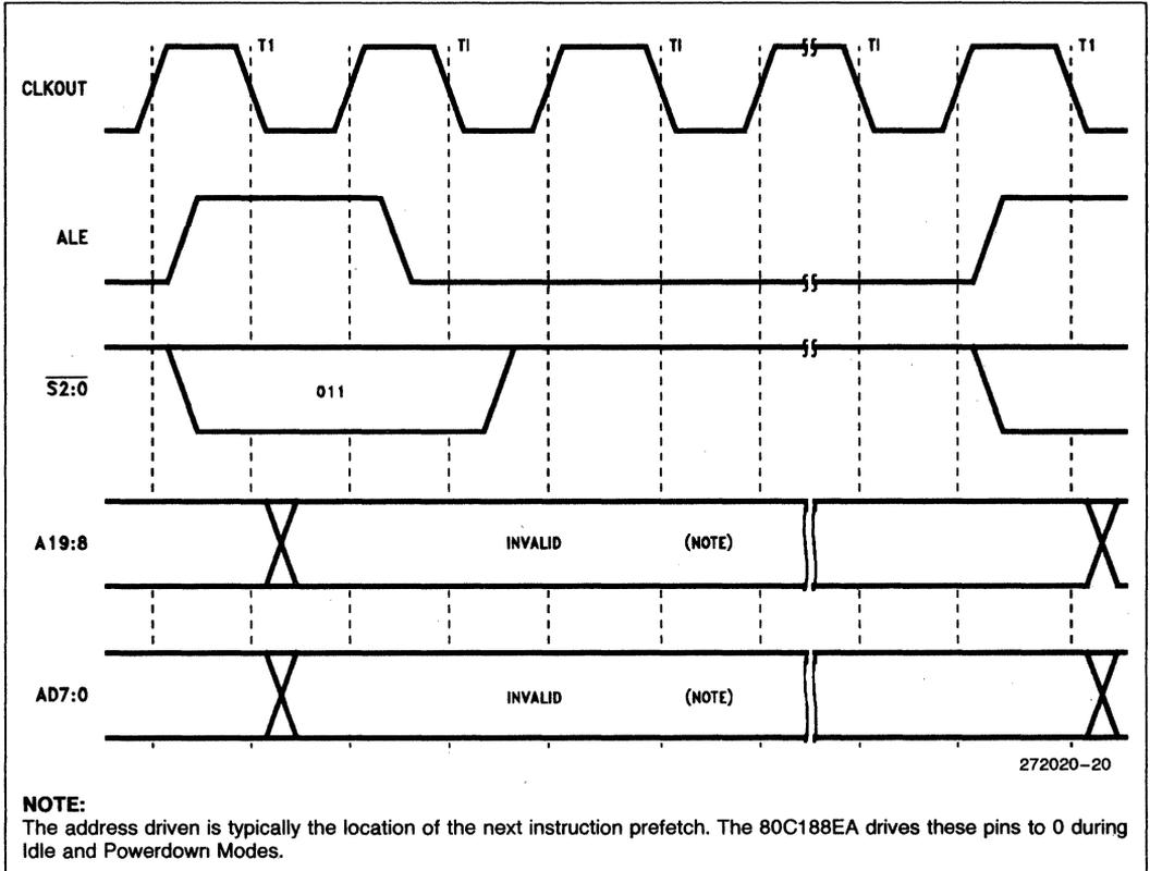
Figure 18. Halt Cycle Waveform
