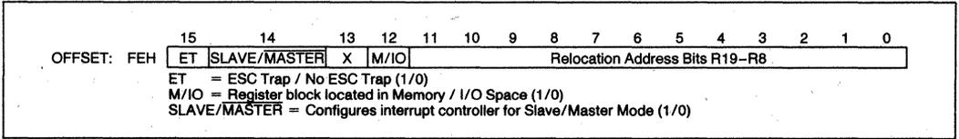
Figure 9. Relocation Register
