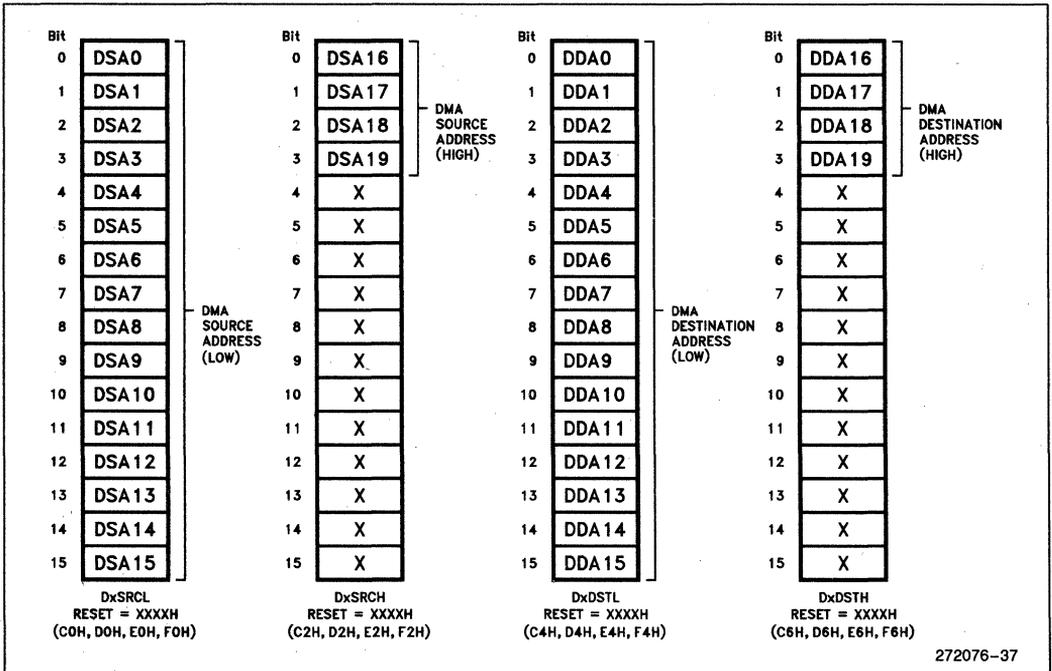
Figure 35. DMA Unit Registers
