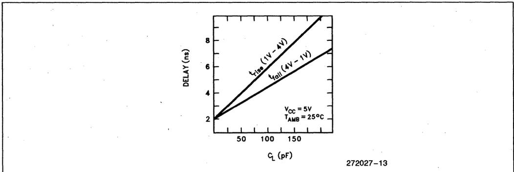
Figure 14. Typical Rise and Fall Variations versus Load Capacitance
