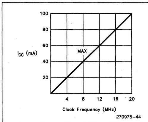
**Figure 4. I<sub>CC</sub> vs Frequency**
