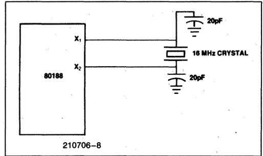
Figure 8. Recommended 8 MHz 80188 Crystal Configuration
