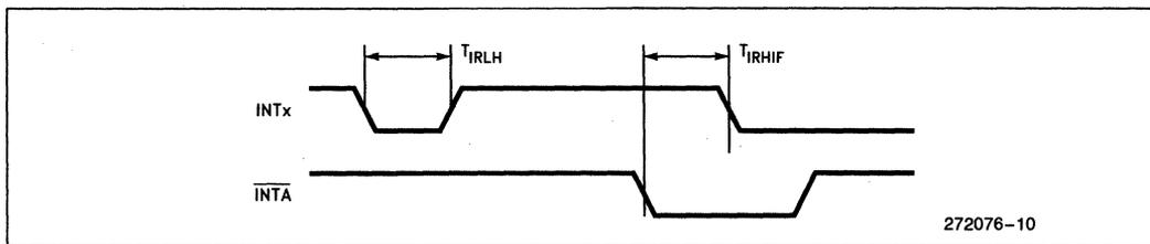
Figure 10. Relative Interrupt Signal Timings
