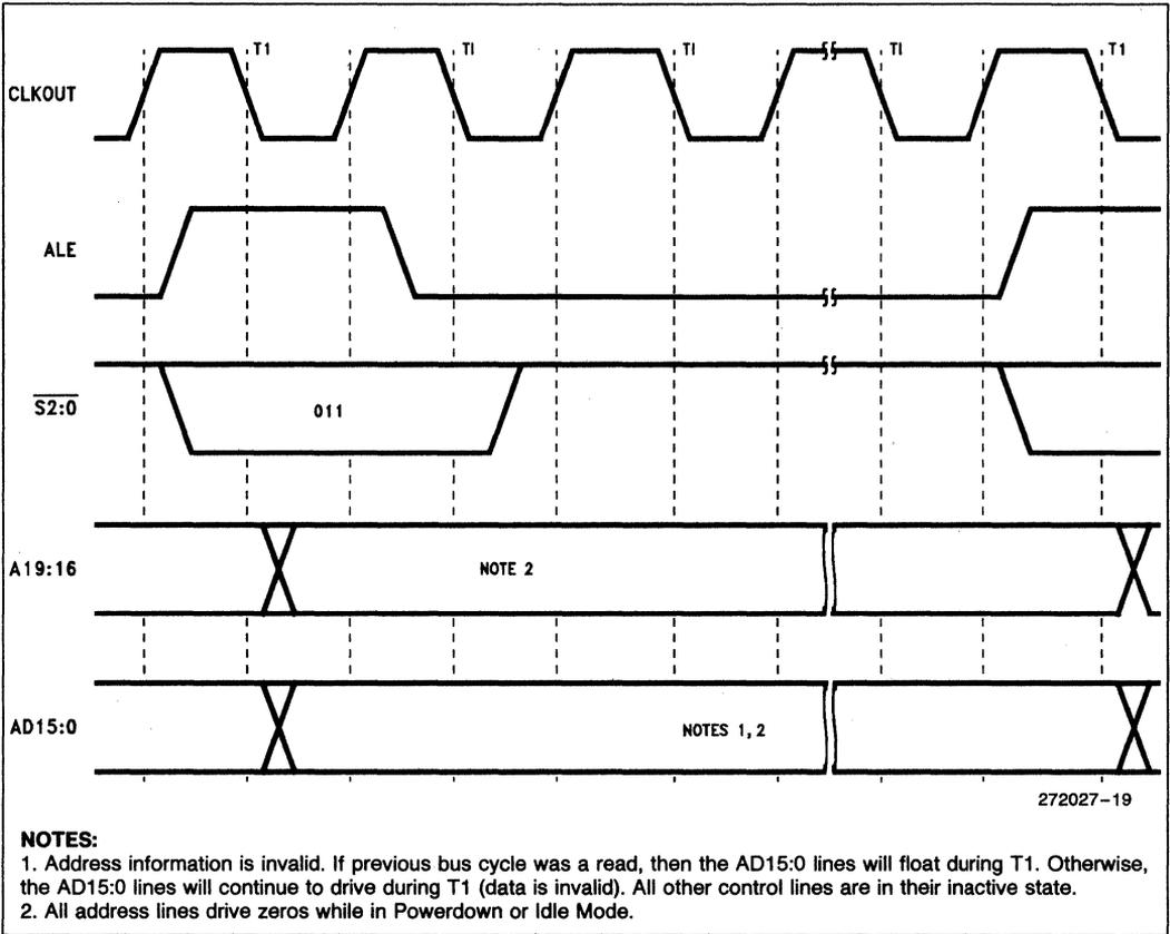
Figure 19. Halt Cycle Waveform
