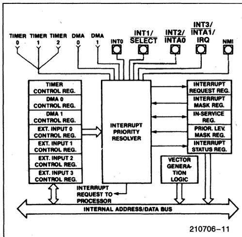
Figure 21. Interrupt Controller Block Diagram
