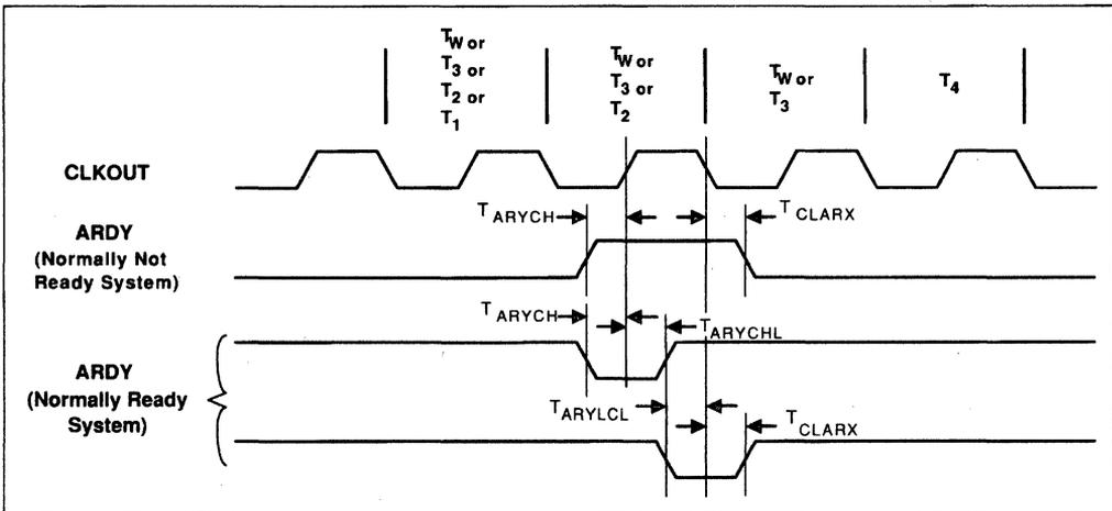
**PERIPHERAL AND QUEUE STATUS WAVEFORMS**
