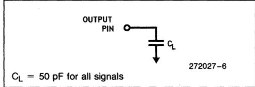
**Figure 6. AC Test Load**
