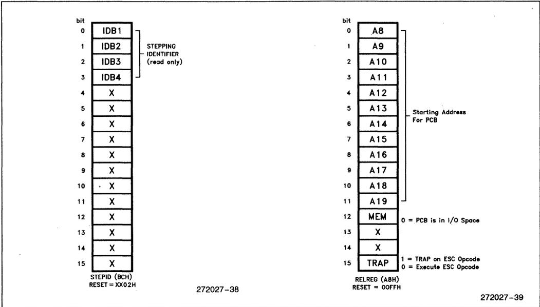
Figure 37. Relocation and Stepping Identifier Registers
