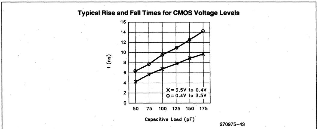
Figure 18. CMOS Level Slew Rates for Output Buffers
