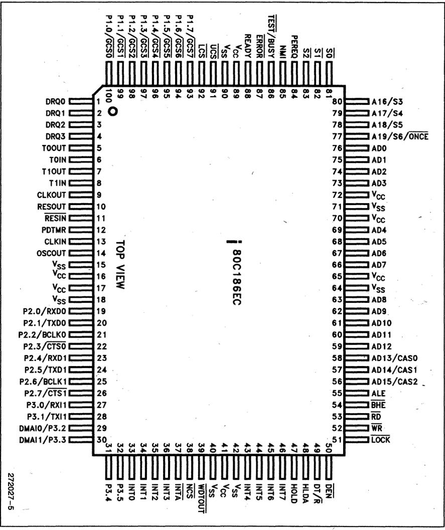
Figure 5. Quad Flat Pack (EIAJ) Pinout Diagram
