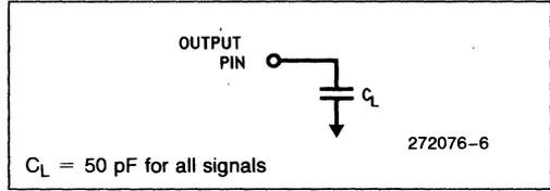
Figure 6. AC Test Load
