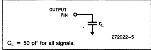
**Figure 4. AC Test Load**
