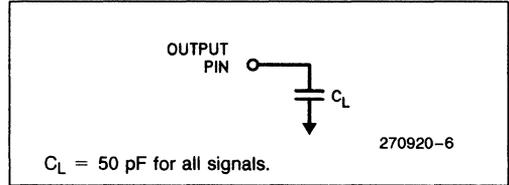
**Figure 4. AC Test Load**
