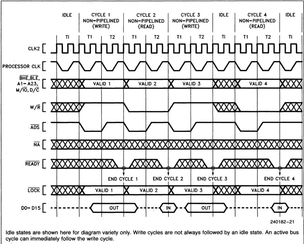
Figure 4.6. Various Non-Pipelined Bus Cycles (Zero Wait States)
