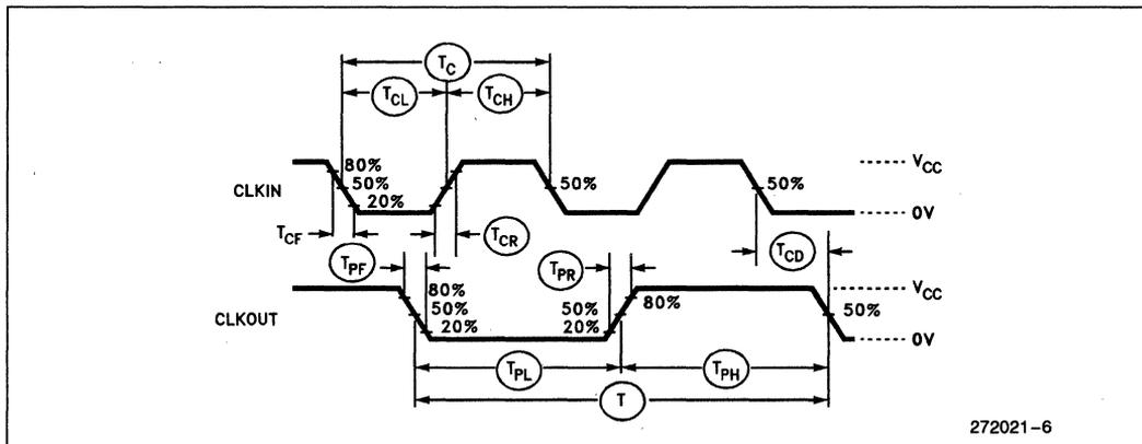
**Figure 5. Input and Output Clock Waveform**
