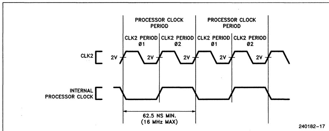
Figure 4.2. CLK2 Signal and Internal Processor Clock
