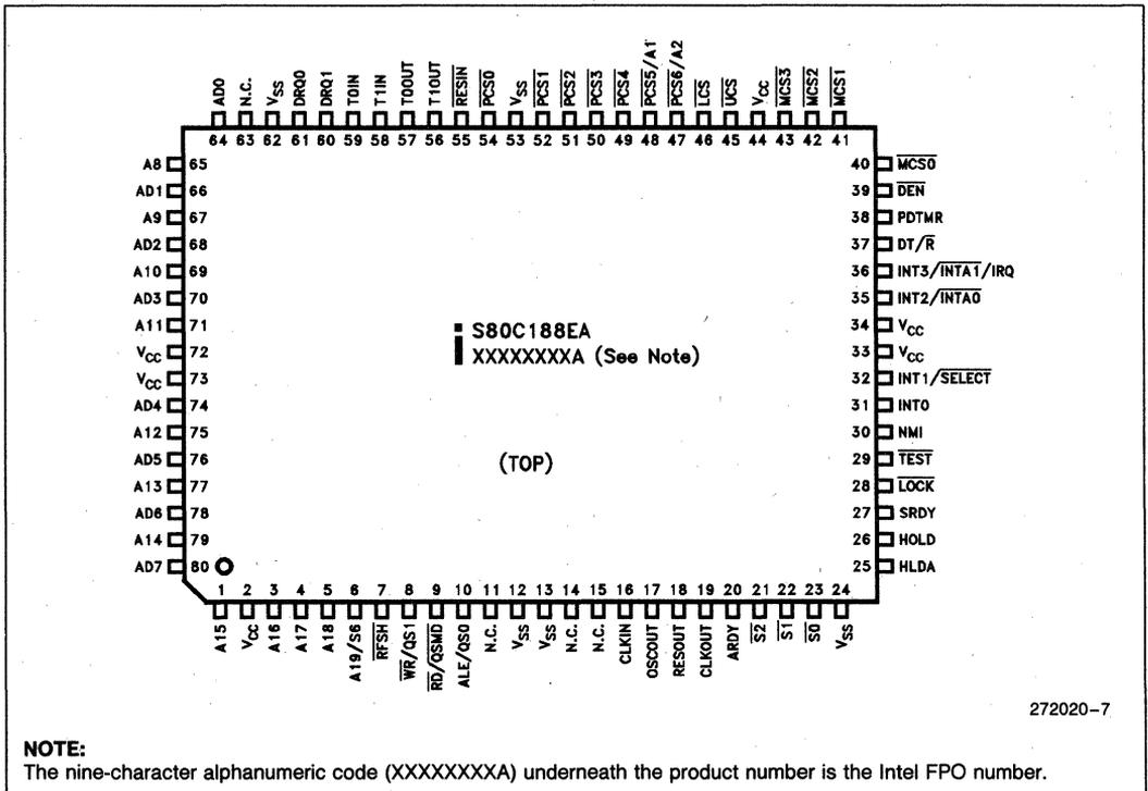
Figure 6. Quad Flat Pack (EIAJ) Pinout Diagram
