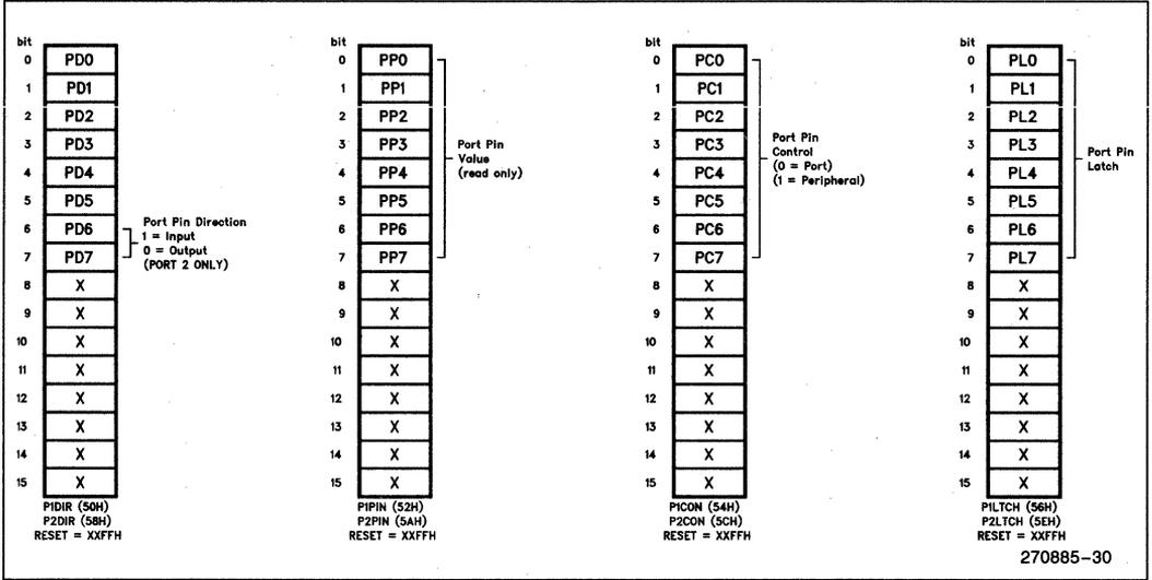
Figure 27. I/O Port Unit Registers
