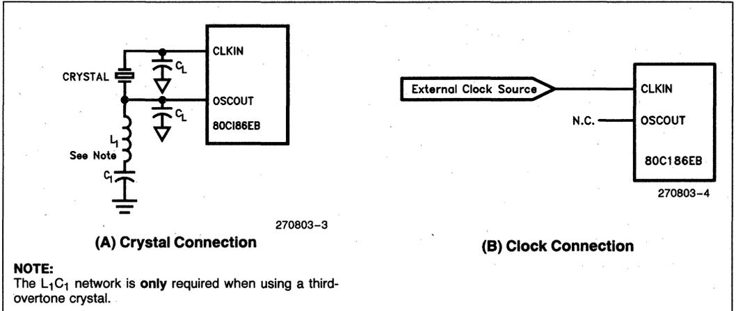
**Figure 2. 80C186EB Clock Configurations**
