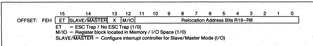
Figure 9. Relocation Register
