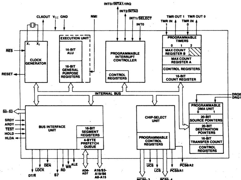
Figure 1. 80188 Block Diagram
