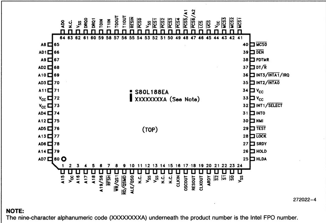
Figure 3. Quad Flat Pack (EIAJ) Pinout Diagram
