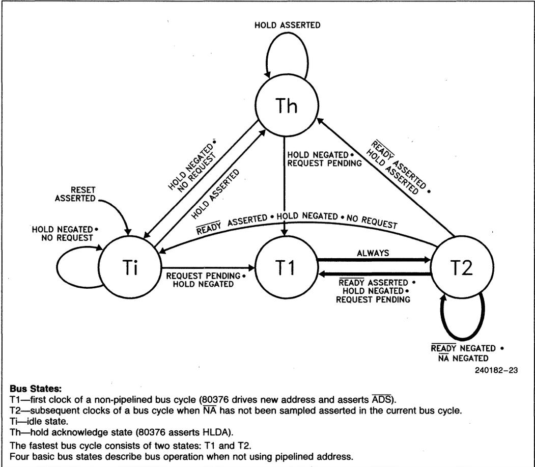
**Figure 4.8. 80376 Bus States (Not Using Pipelined Address)**
