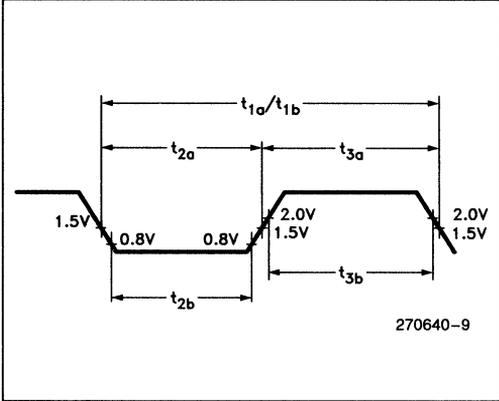
**AC SETUP, HOLD, AND DELAY TIME MEASUREMENTS—GENERAL**
