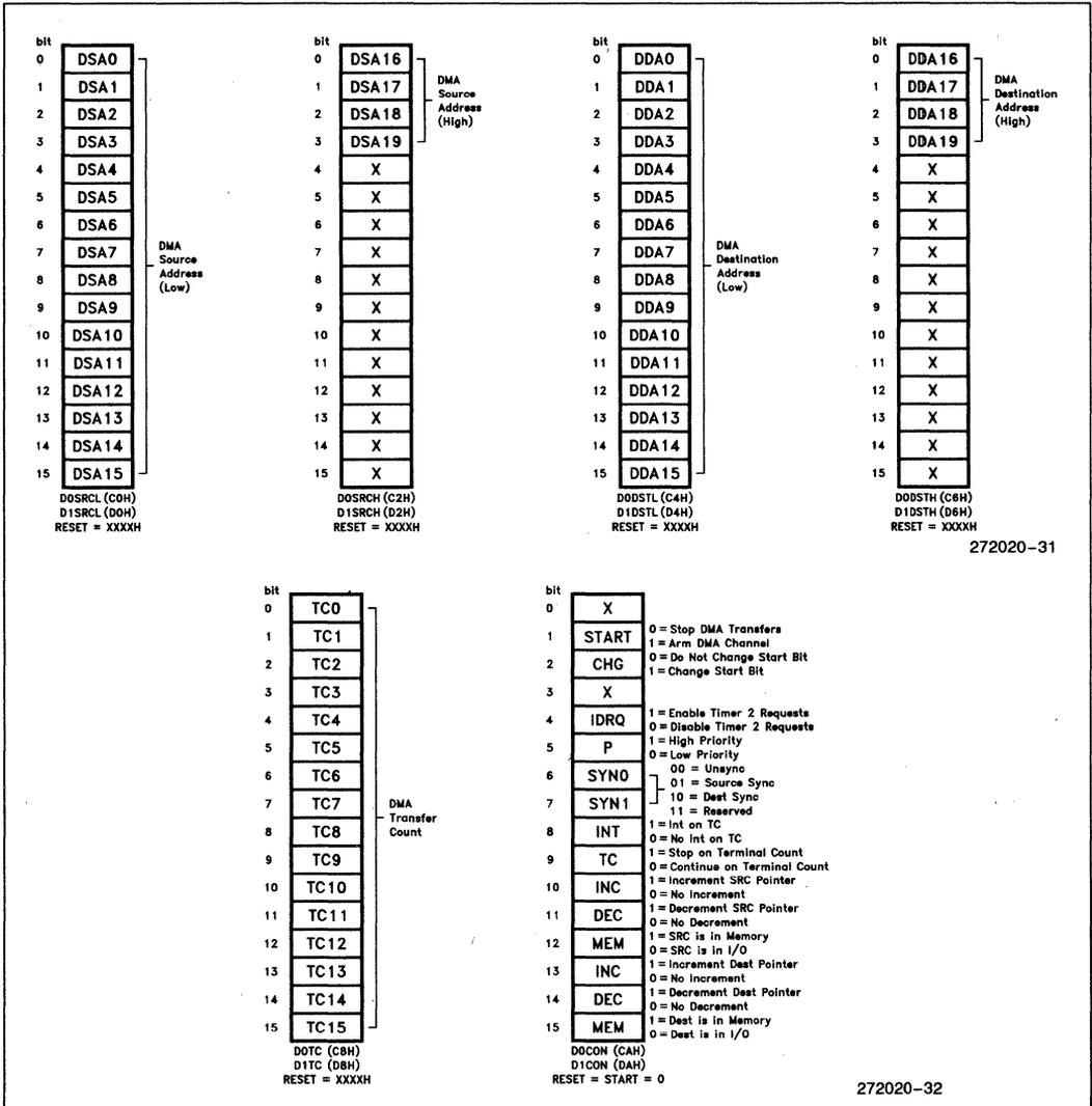
Figure 28. DMA Unit Registers
