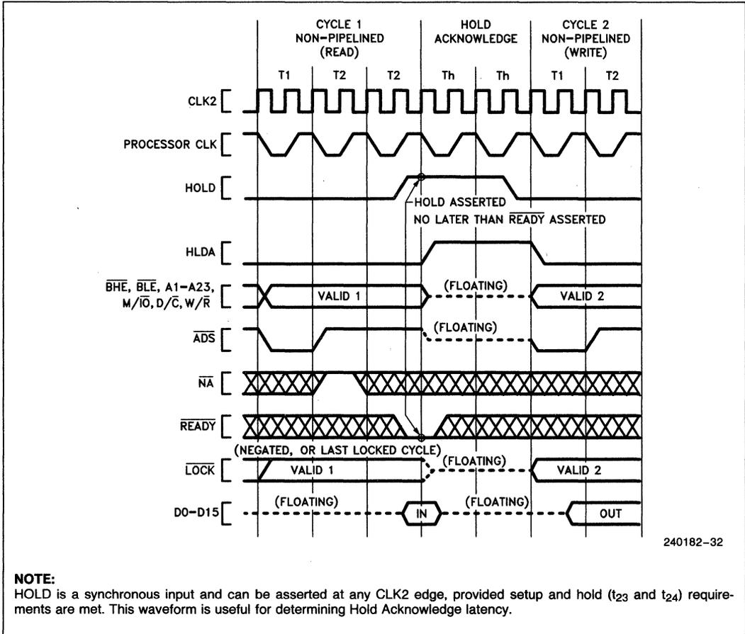
Figure 4.17. Requesting Hold from Active Bus ( $\overline{N\bar{A}}$  Inactive)
