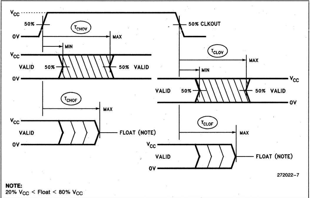
Figure 6. Output Delay and Float Waveform
