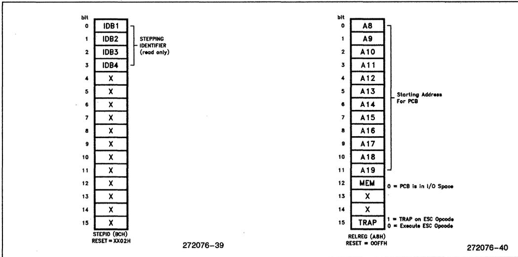
Figure 37. Relocation and Stepping Identifier Registers
