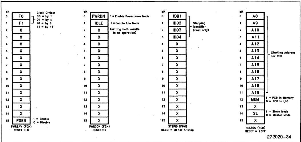
Figure 30. Power Management, Relocation and Stepping Registers
