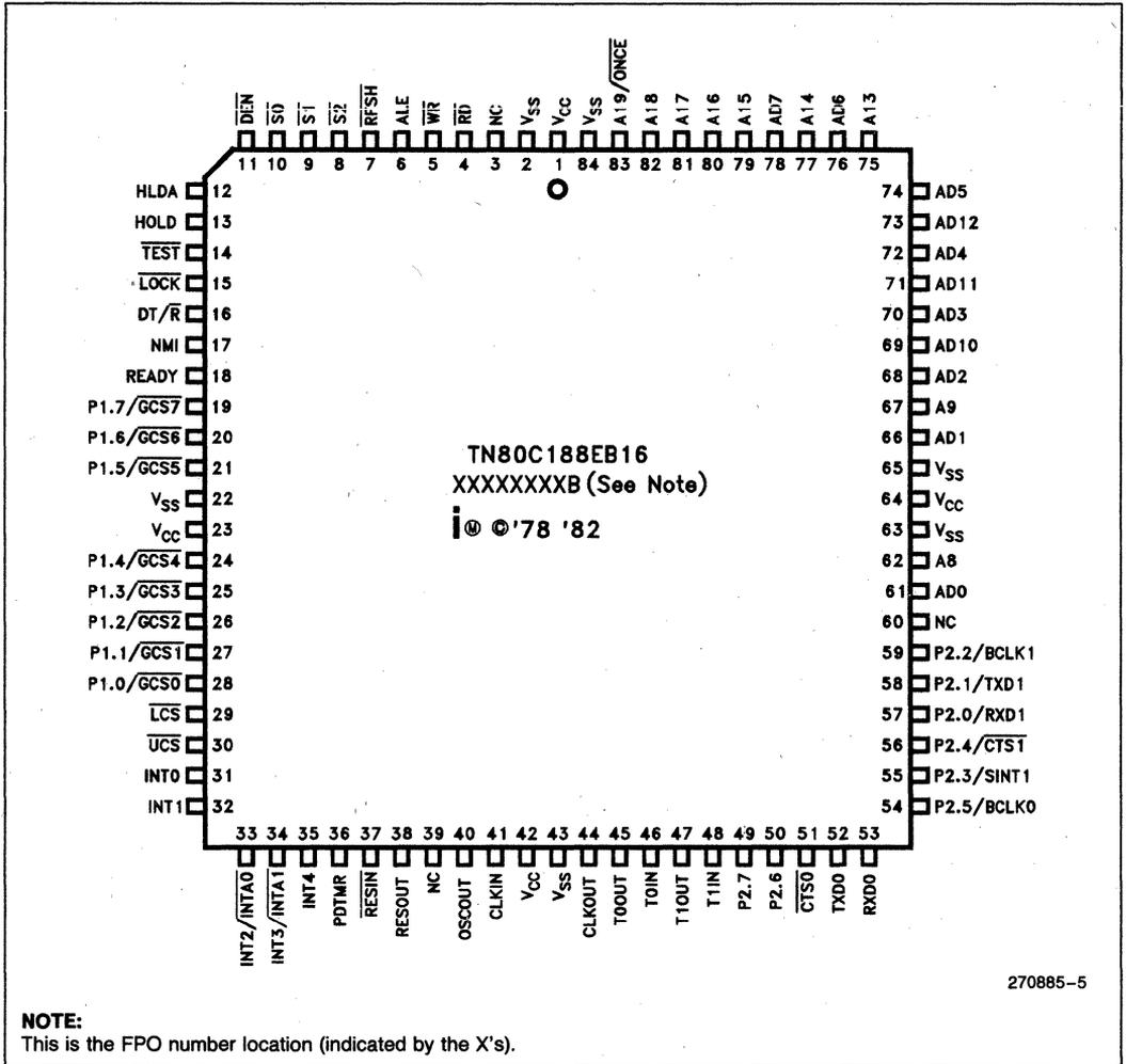
**Figure 5. 84-Pin Plastic Leaded Chip Carrier Pinout Diagram**
