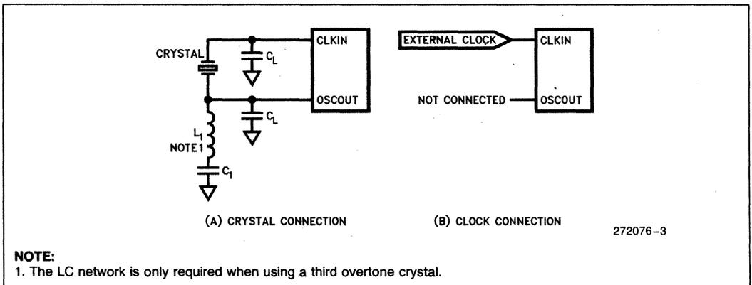
**Figure 2. 80C188EC Clock Connections**
