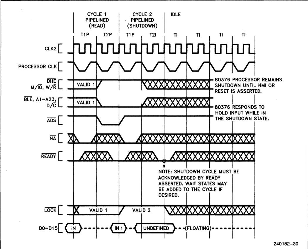
Figure 4.15. Example Shutdown Indication Cycle from Non-Pipelined Cycle
