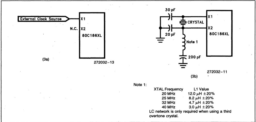
Figure 3. 80C186XL Oscillator Configurations (see text)
