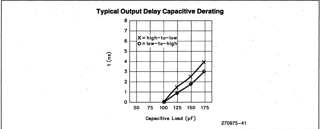
Figure 16. Capacitive Derating Curve
