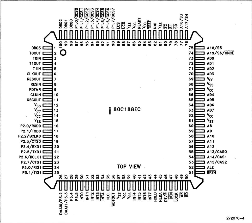
Figure 4. 100-Pin Plastic Quad Flat Pack Package (PQFP)
