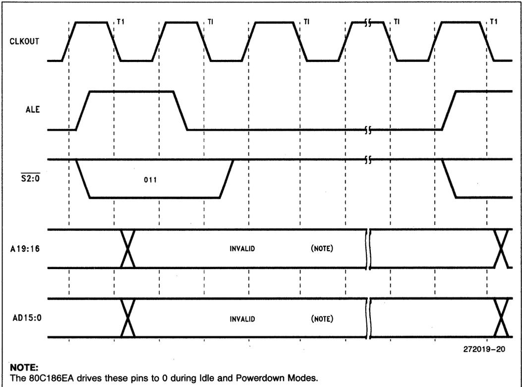
Figure 18. Halt Cycle Waveform
