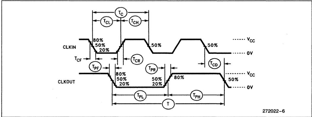
**Figure 5. Input and Output Clock Waveform**
