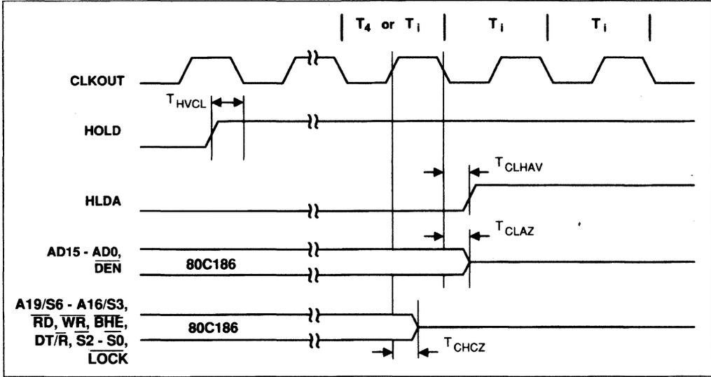
HOLD/HLDA WAVEFORMS (Leaving Hold)
