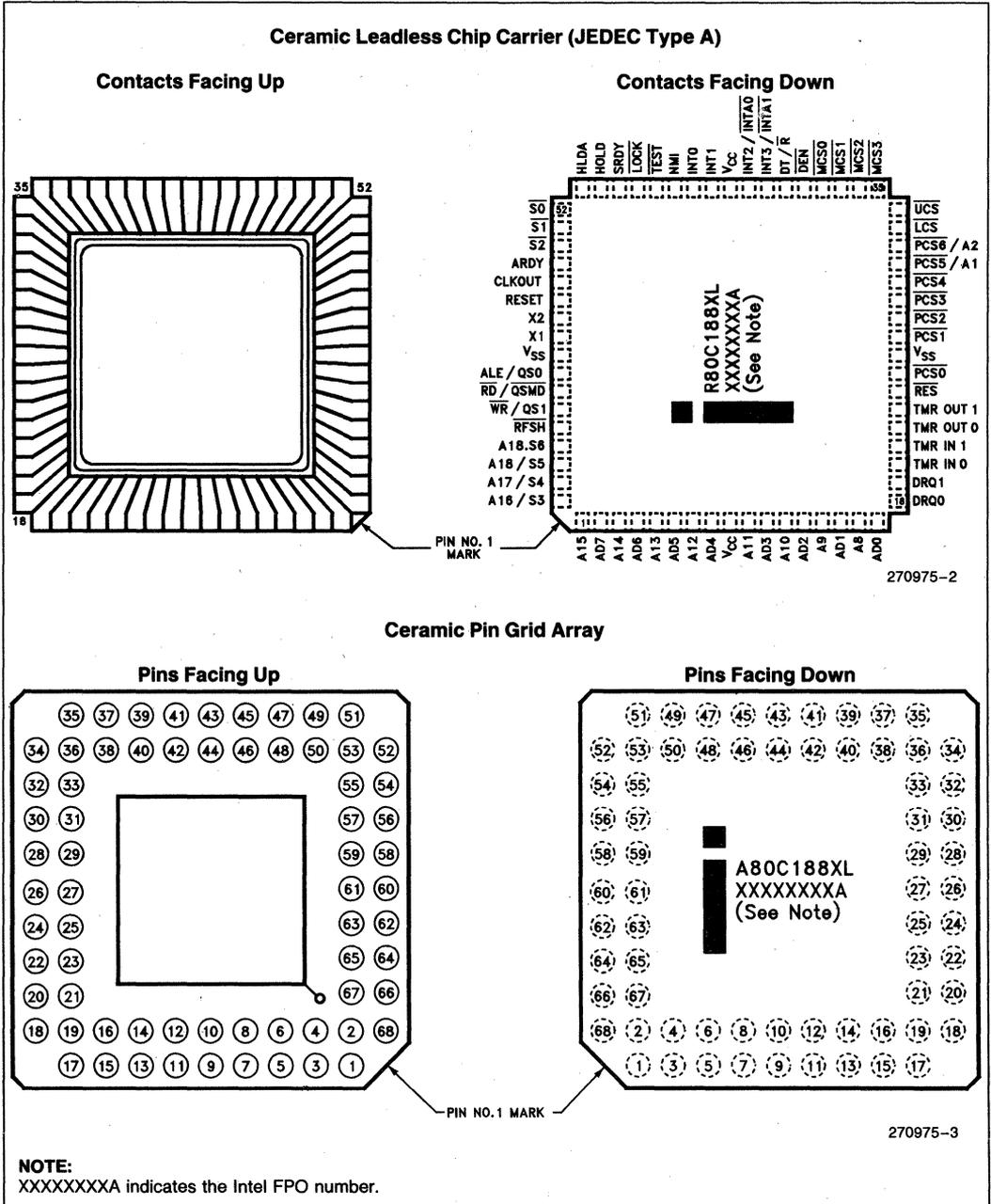
Figure 2. 80C188XL Pinout Diagrams
