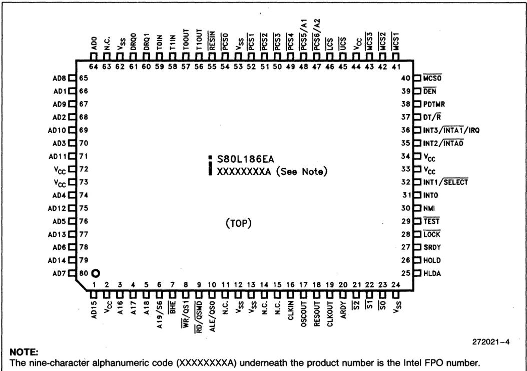
Figure 3. Quad Flat Pack (EIAJ) Pinout Diagram
