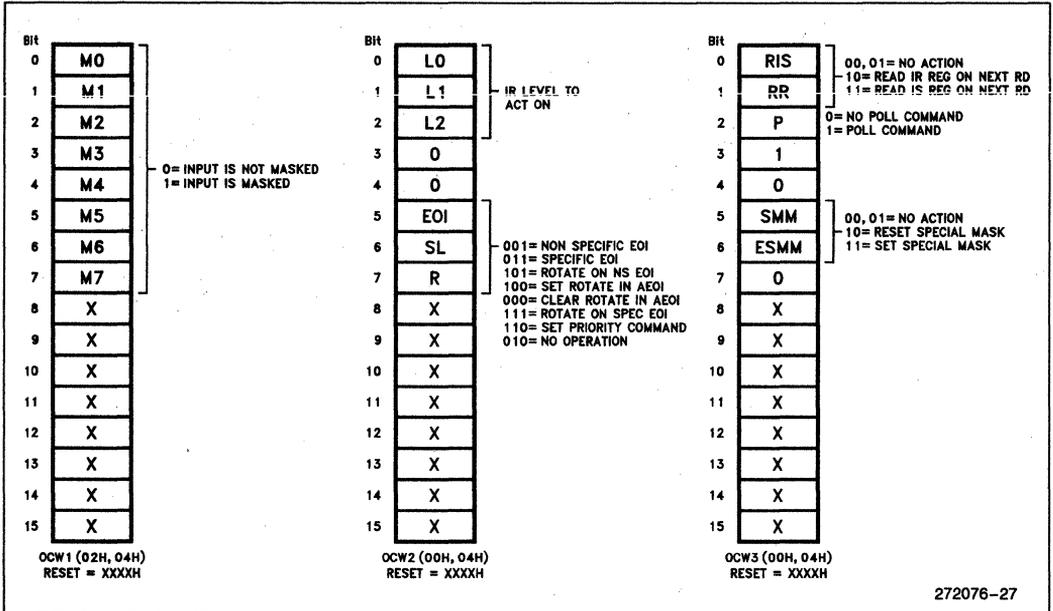
Figure 26. 8259A Module Operation Command Words
