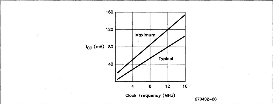
**Figure 46. I<sub>CC</sub> vs Frequency**
