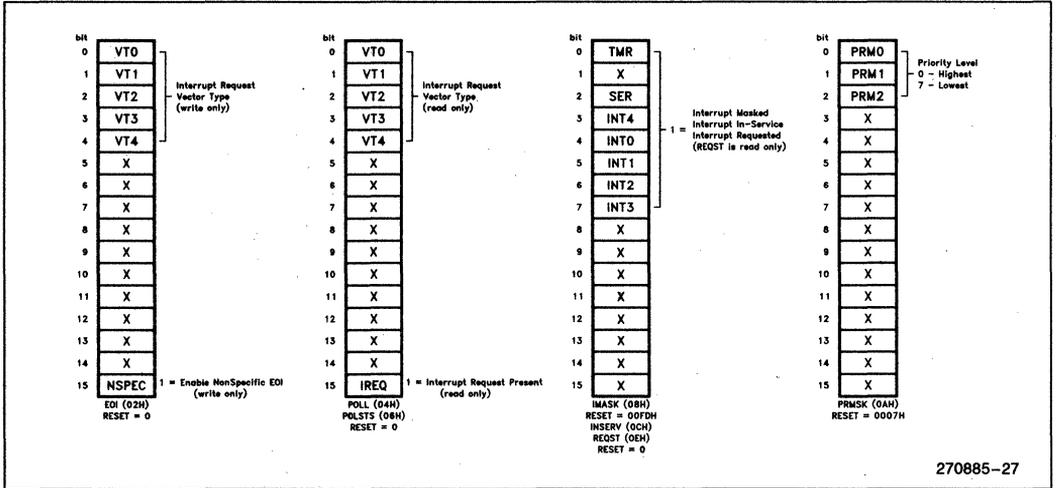
**Figure 24. Interrupt Control Unit Registers**
