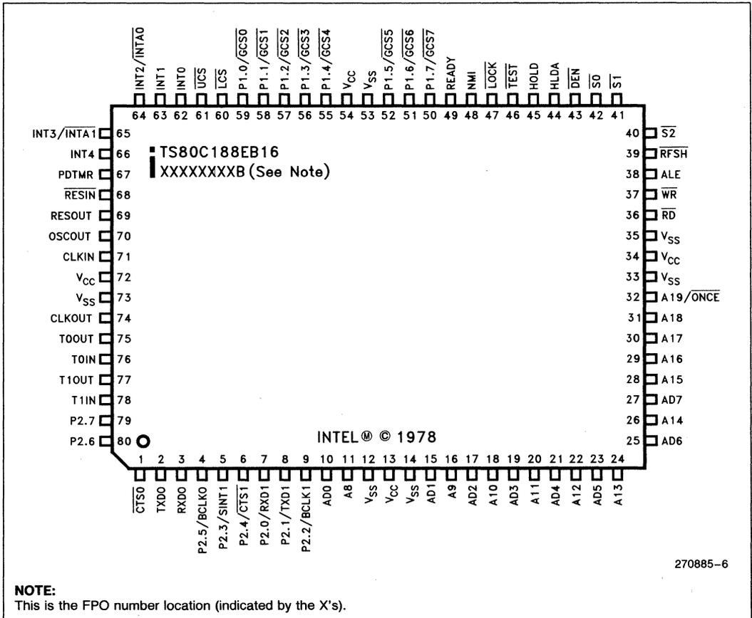
Figure 6. Quad Flat Pack Pinout Diagram
