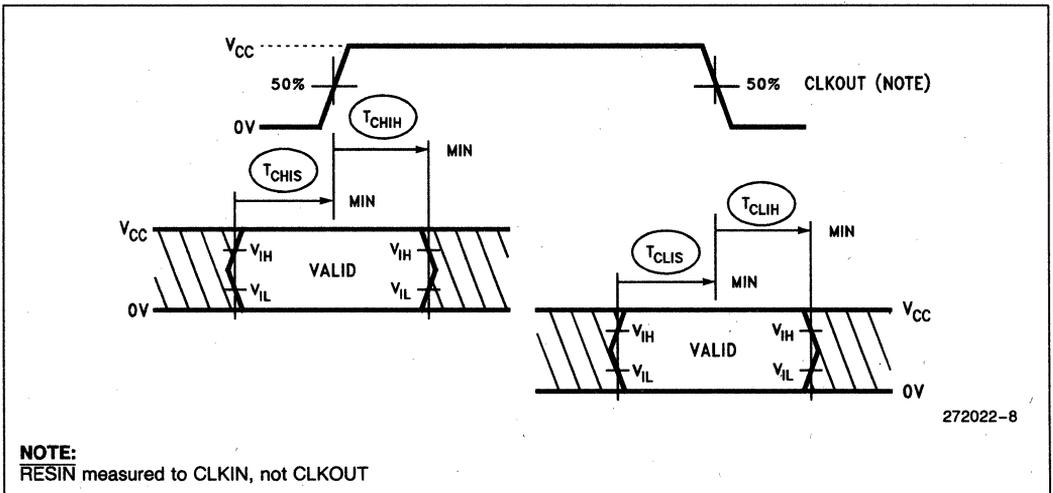
Figure 7. Input Setup and Hold
