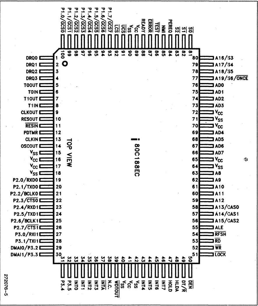
Figure 5. Quad Flat Pack (EIAJ) Pinout Diagram
