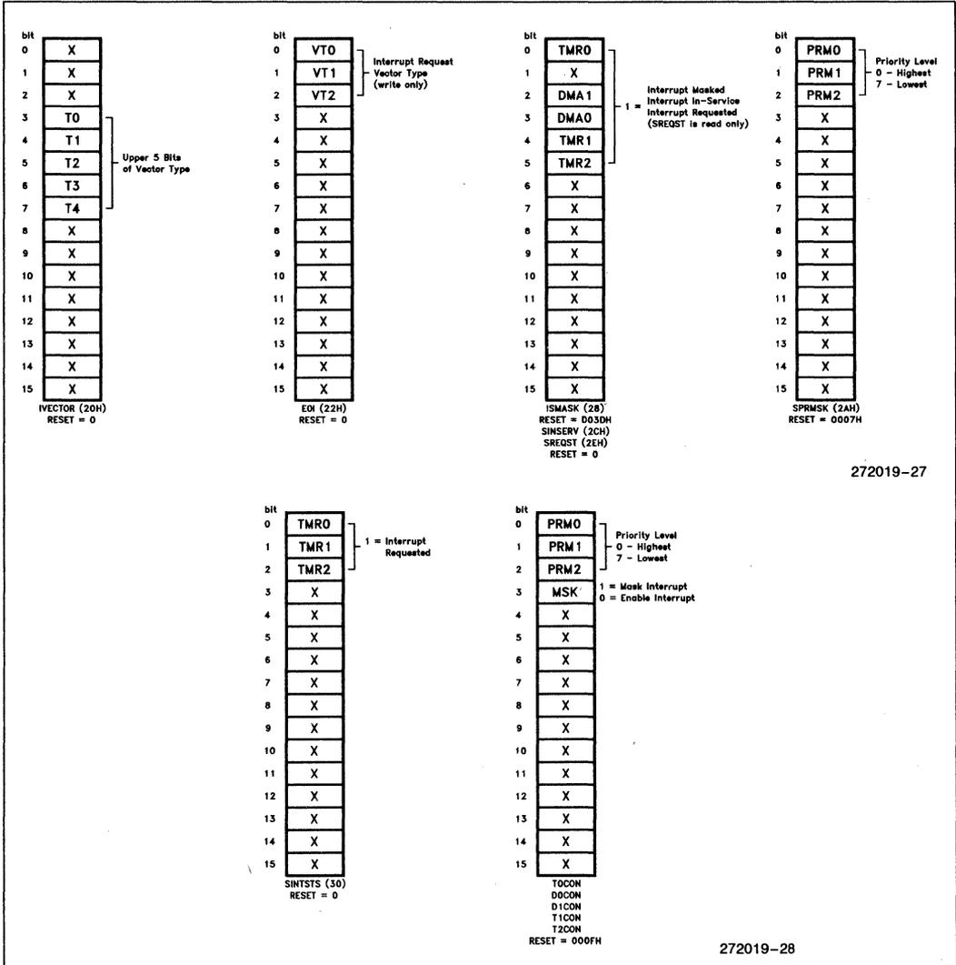
Figure 25. Interrupt Control Unit Registers (Slave Mode)
