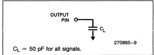
**Figure 7. AC Test Load**
