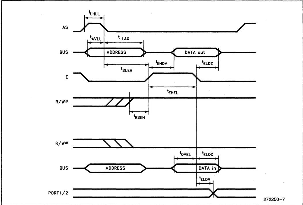
**A.C. Characteristics for 8-Bit Non-Multiplexed Asynchronous (Mode 3)**Conditions:  $V_{CC} = 5V \pm 10\%$ ,  $V_{SS} = 0V$ ,  $T_A = -40^\circ\text{C}$  to  $+125^\circ\text{C}$ ,  $C_L = 100\text{ pF}$
