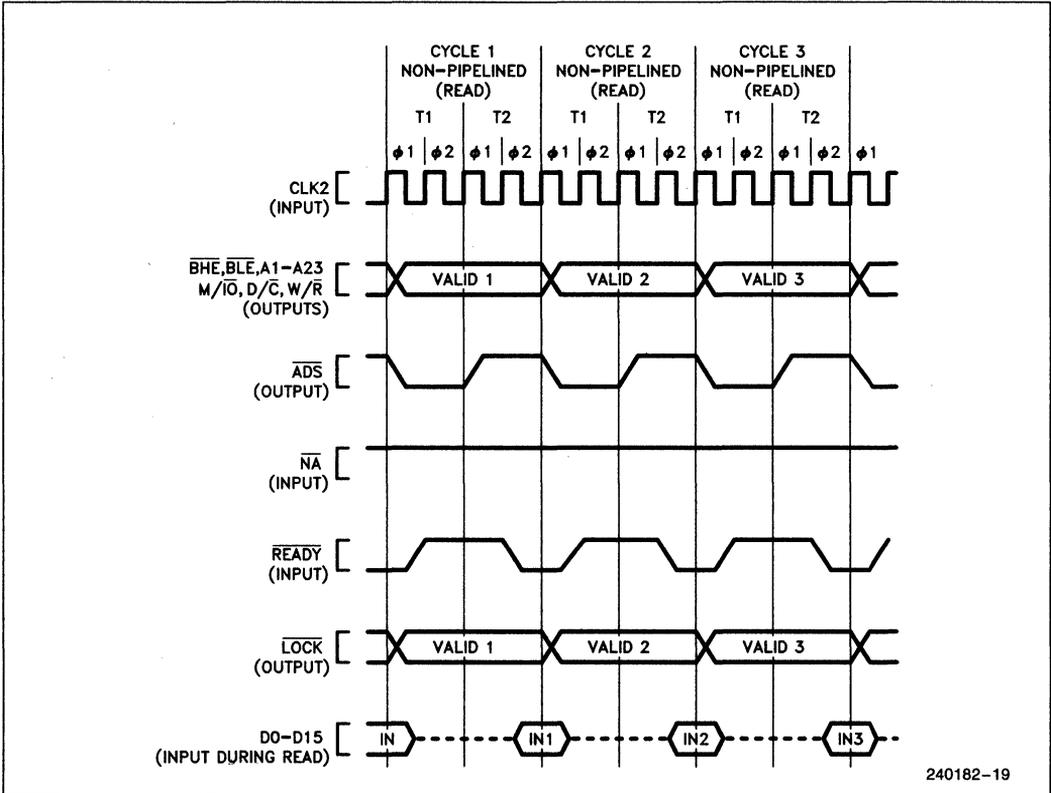
Figure 4.4. Fastest Read Cycles with Non-Pipelined Timing
