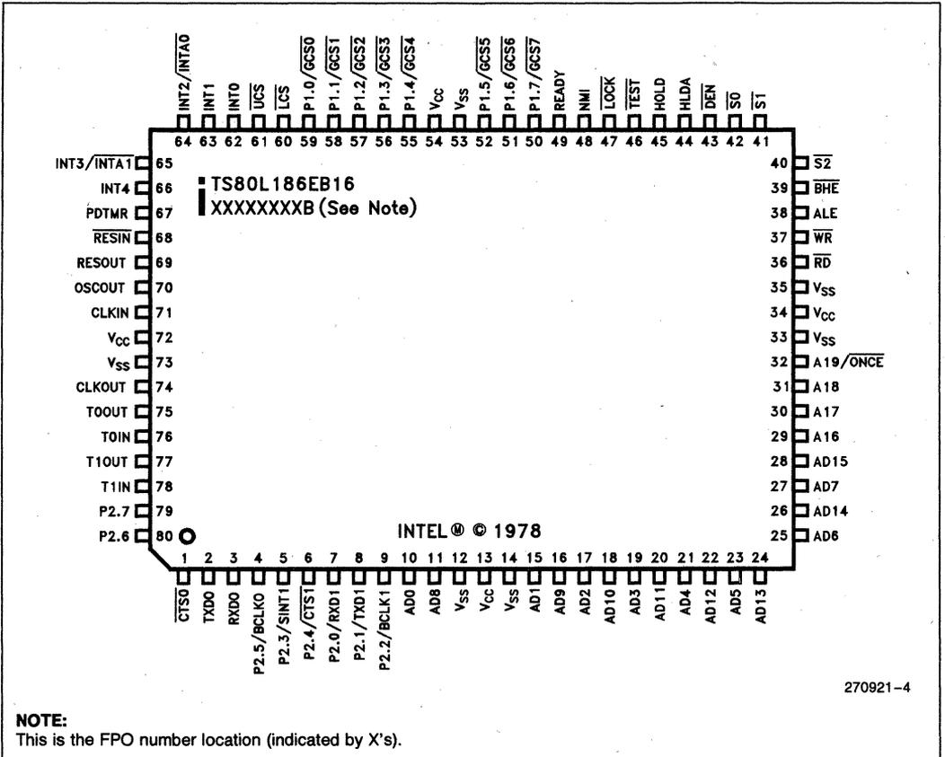
Figure 3. Quad Flat Pack Pinout Diagram
