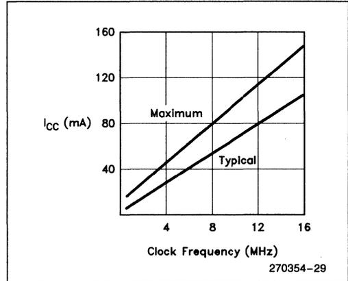
Figure 46.  $I_{CC}$  vs Frequency
