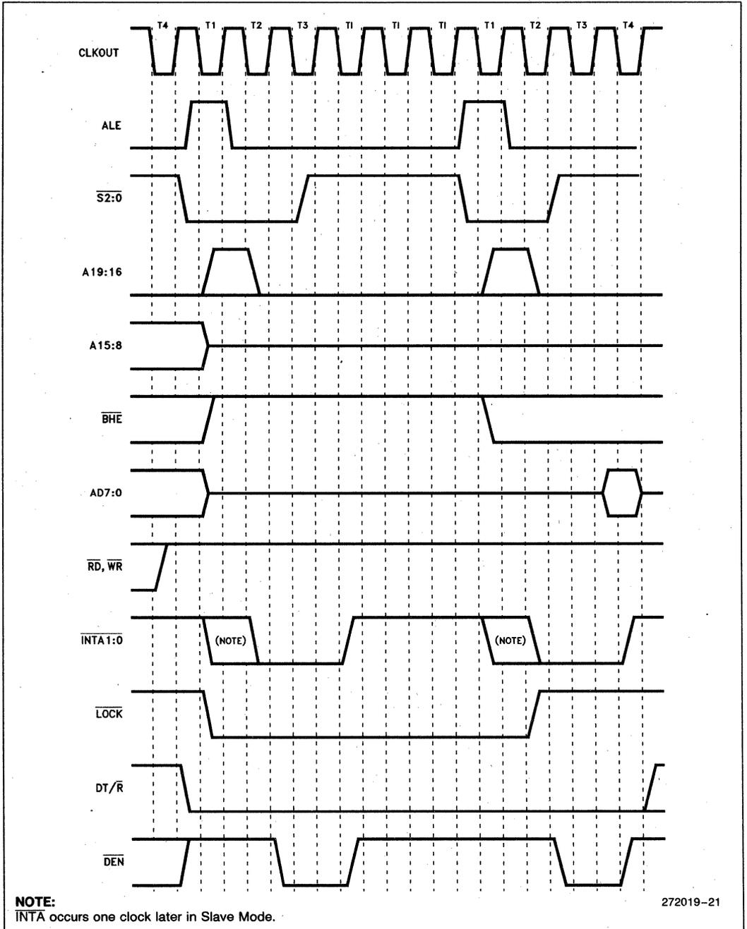
Figure 19.  $\overline{INTA}$  Cycle Waveform
