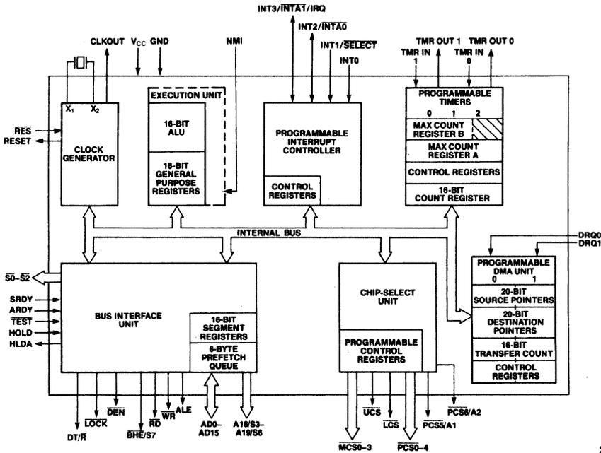
Figure 1. 80186 Block Diagram
