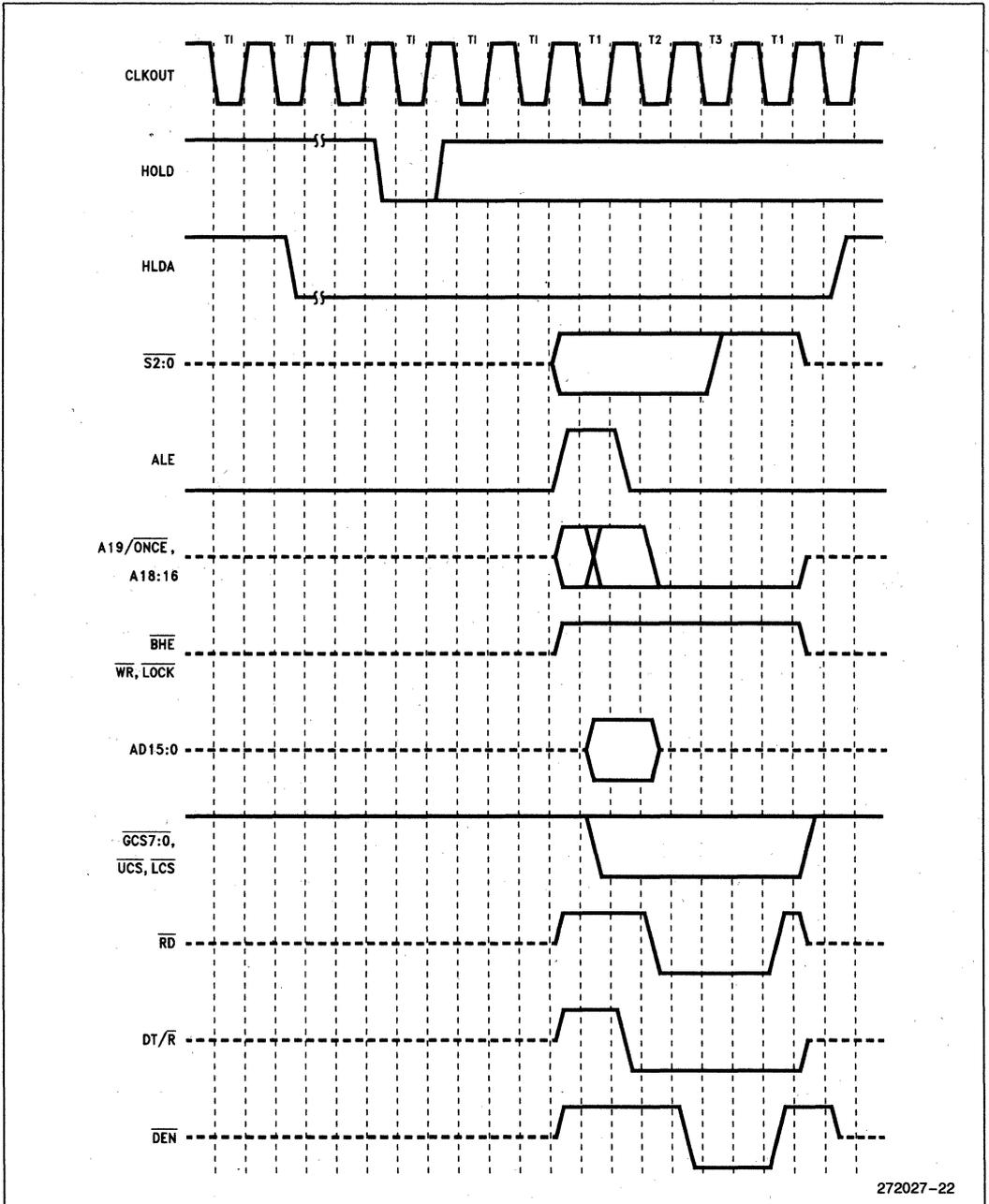
Figure 22. Refresh during HLDA Waveforms
