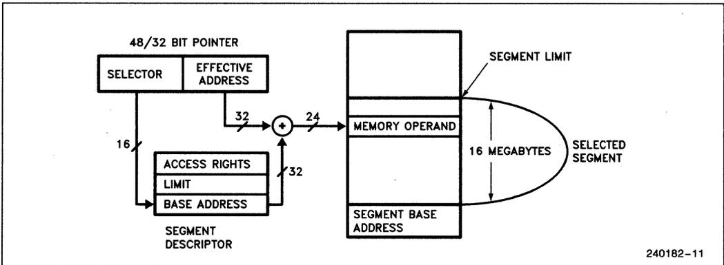
Figure 3.1. Address Calculation
