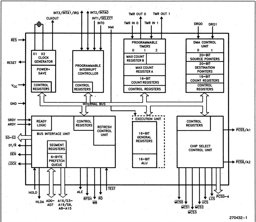
Figure 1. 80C188 Block Diagram
