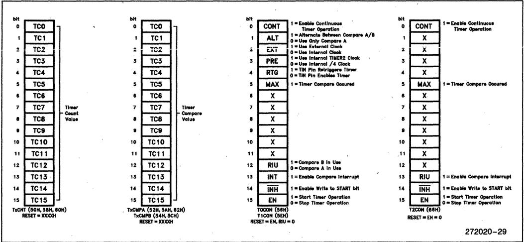
Figure 26. Timer Control Unit Registers
