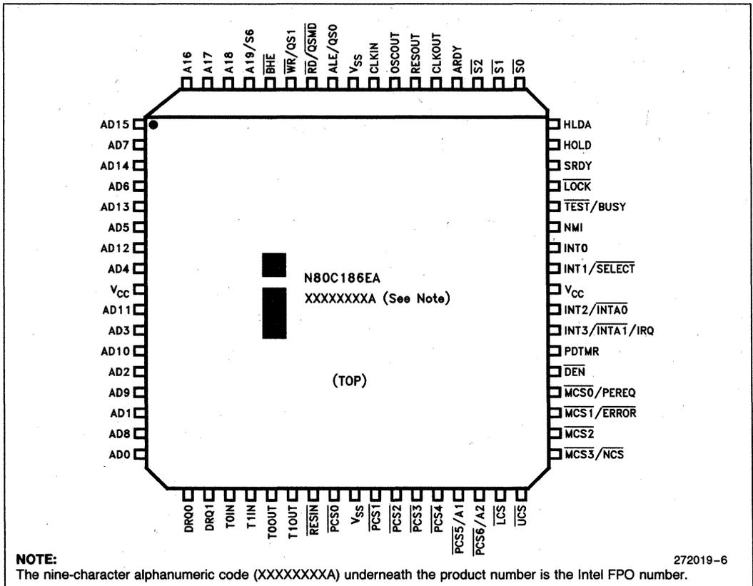
Figure 5. 68-Lead PLCC Pinout Diagram
