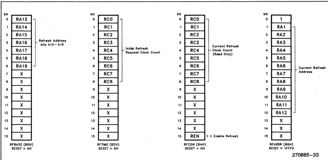
Figure 30. Refresh Control Unit Registers
