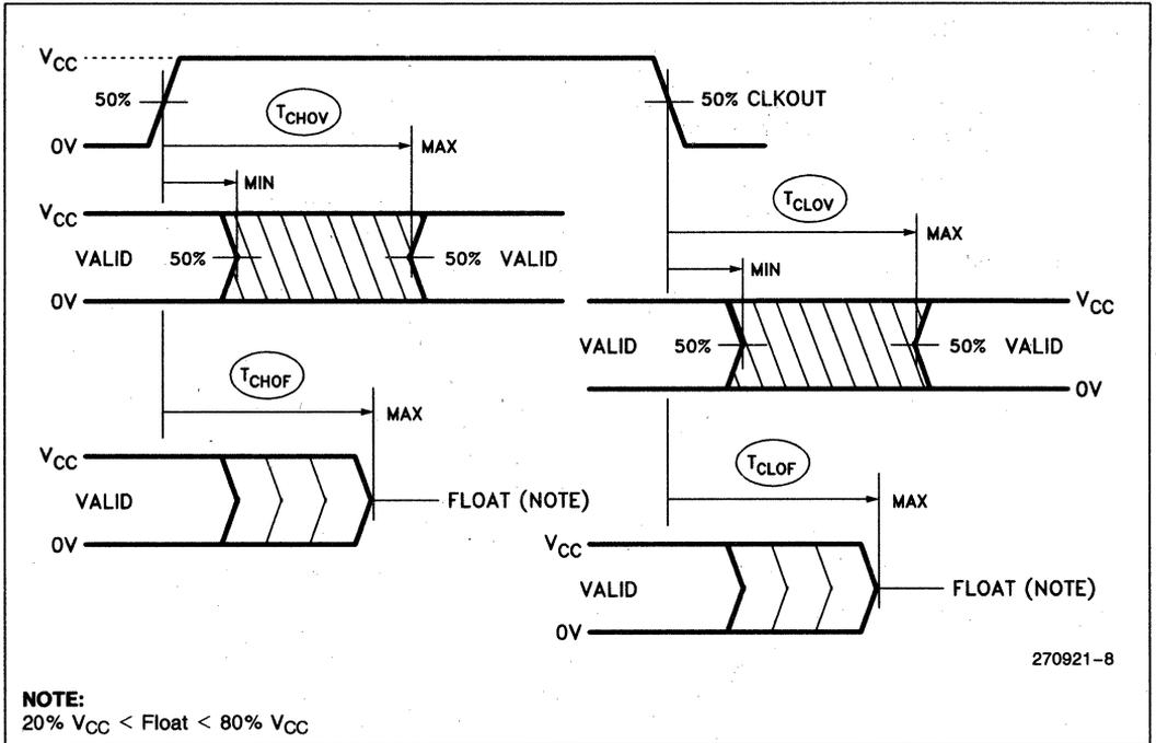
Figure 6. Output Delay and Float Waveform
