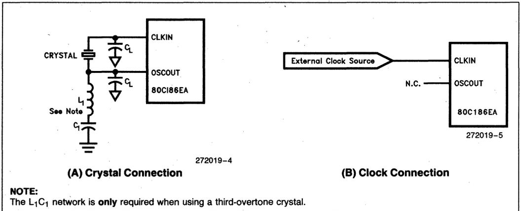
Figure 2. 80C186EA Clock Configurations
