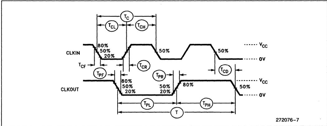
Figure 7. Input and Output Clock Waveforms
