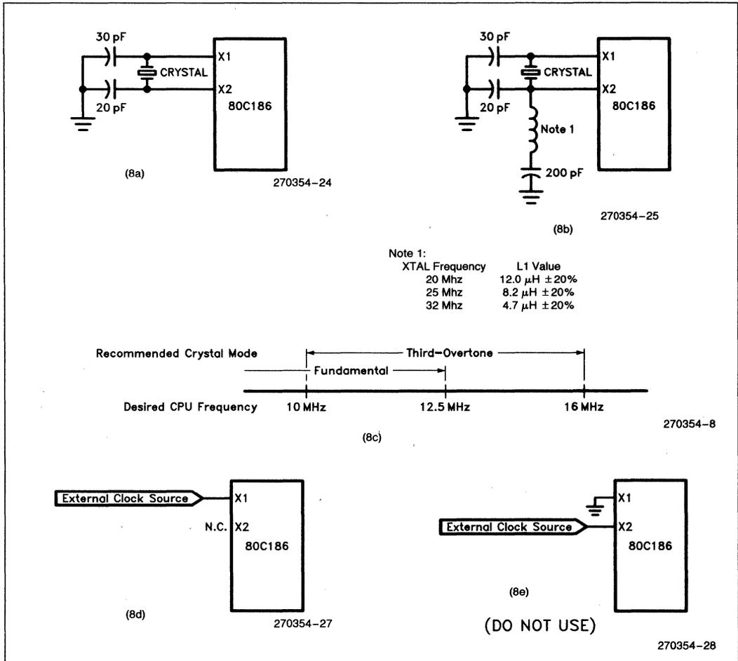
Figure 8. 80C186 Oscillator Configurations (see text)
