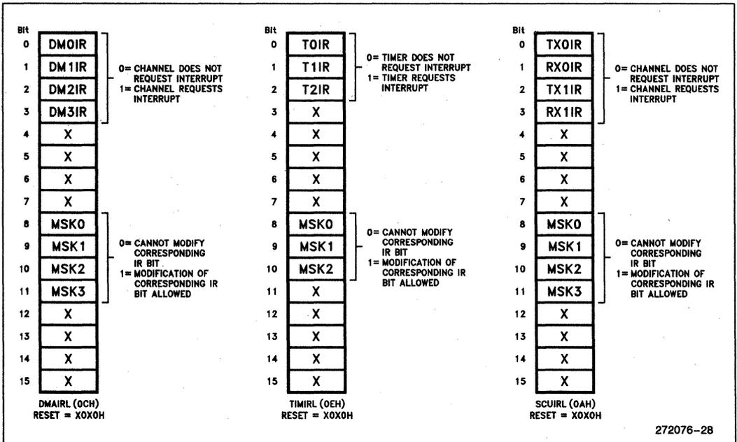
Figure 27. Interrupt Request Latch Registers
