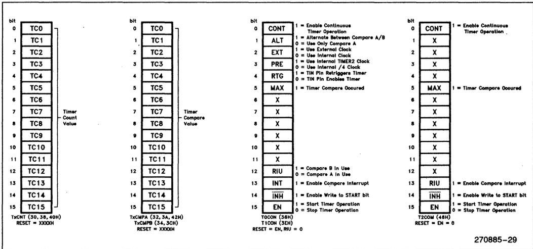
Figure 26. Timer Control Unit Registers
