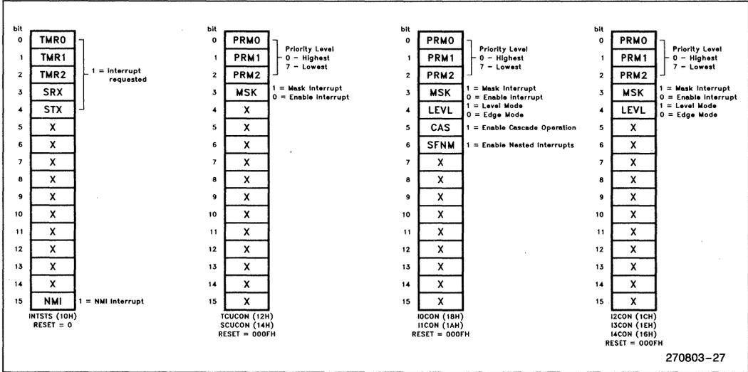
Figure 25. Interrupt Control Unit Registers
