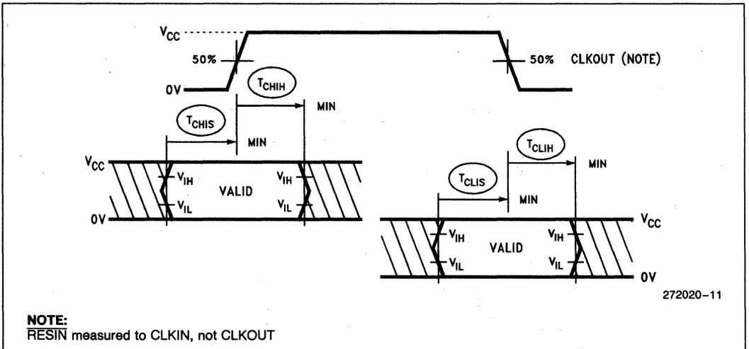
Figure 10. Input Setup and Hold
