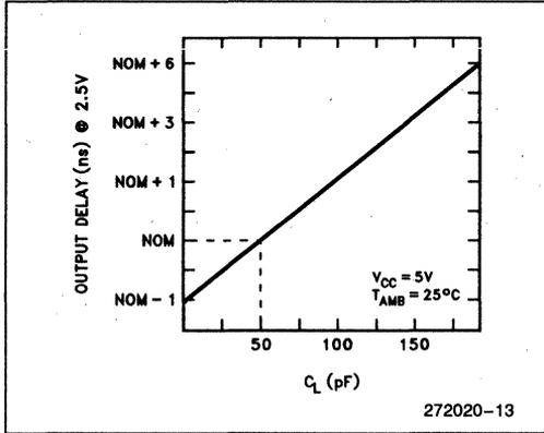
Figure 12. Typical Output Delay Variations Versus Load Capacitance
