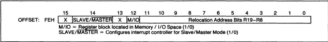
Figure 9. Relocation Register
