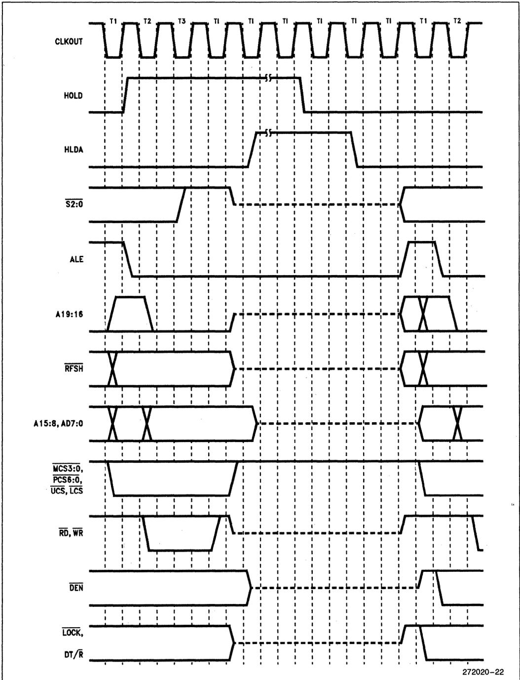
Figure 20. HOLD/HLDA Waveform
