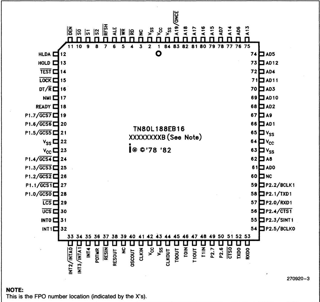
Figure 2. 84-Pin Plastic Leaded Chip Carrier Pinout Diagram
