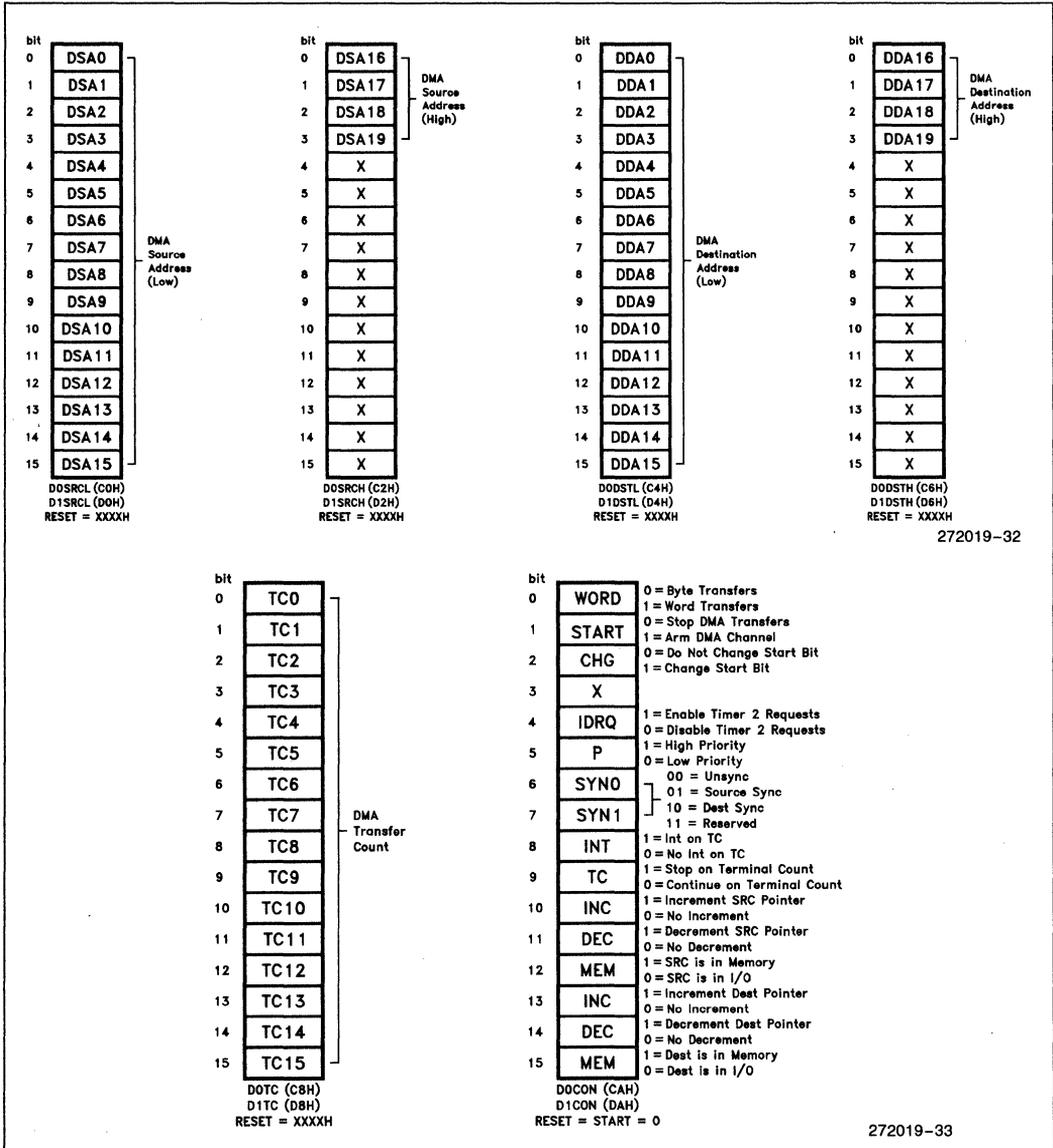
Figure 28. DMA Unit Registers
