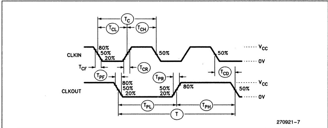
**Figure 5. Input and Output Clock Waveform**
