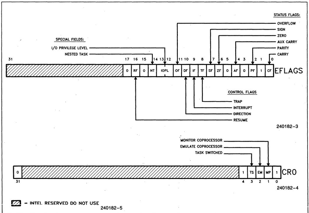
Figure 2.2. Status and Control Register Bit Functions
