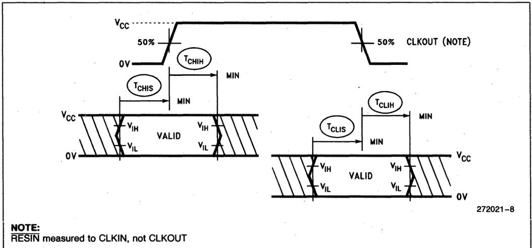
Figure 7. Input Setup and Hold
