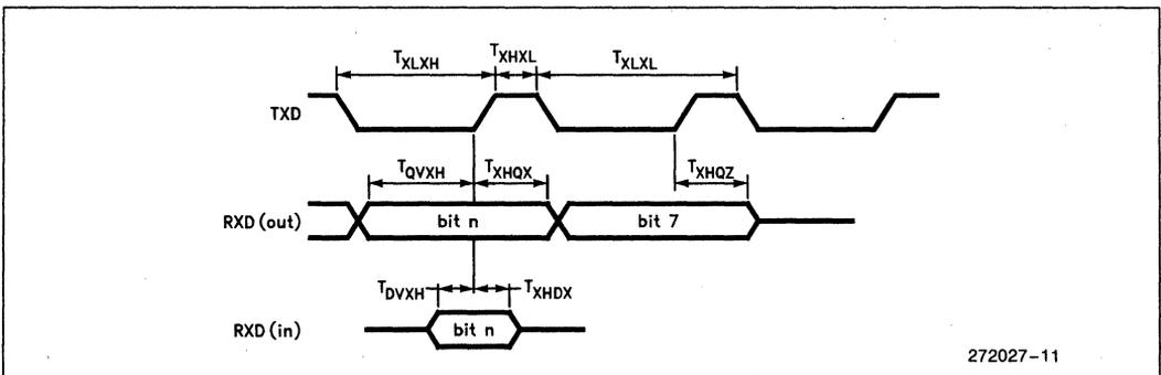
Figure 12. Serial Port Mode 0 Waveform
