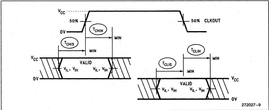
Figure 9. Input Setup and Hold
