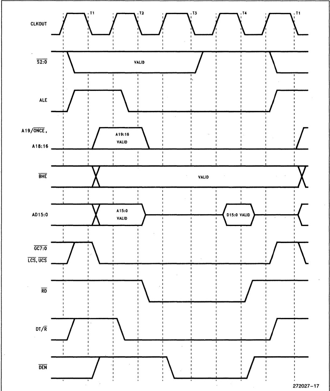
**Figure 17. Memory Read, I/O Read, Instruction Fetch and Refresh Waveform**
