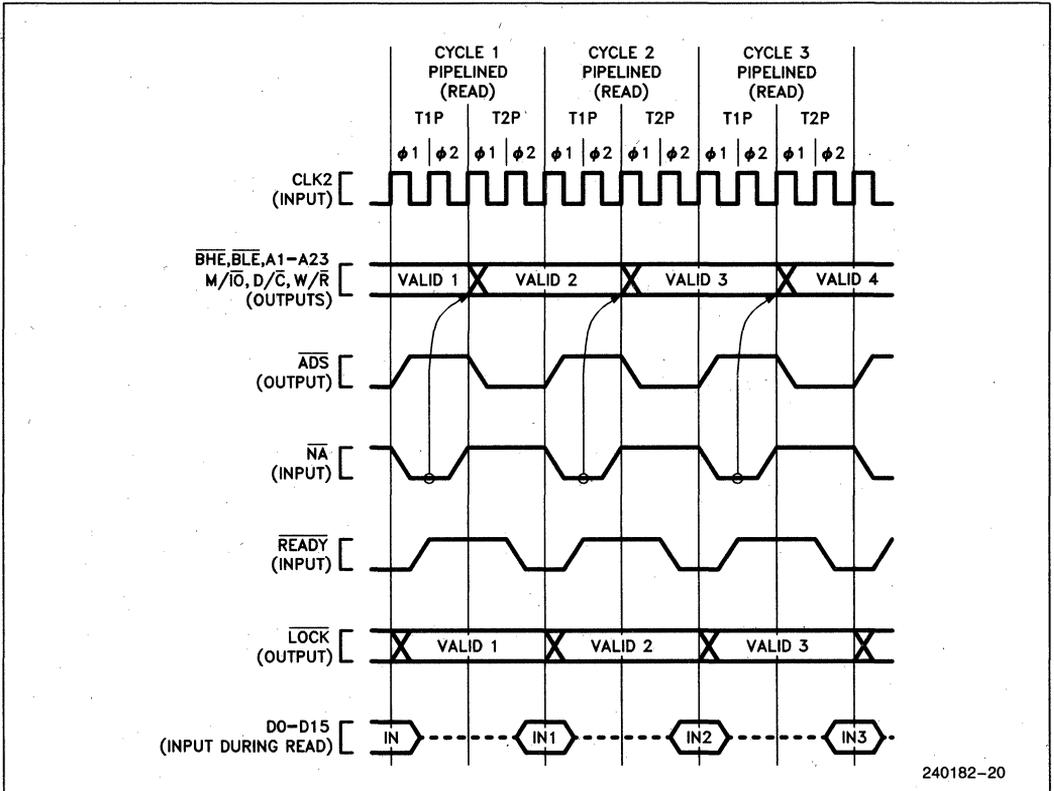
Figure 4.5. Fastest Read Cycles with Pipelined Timing
