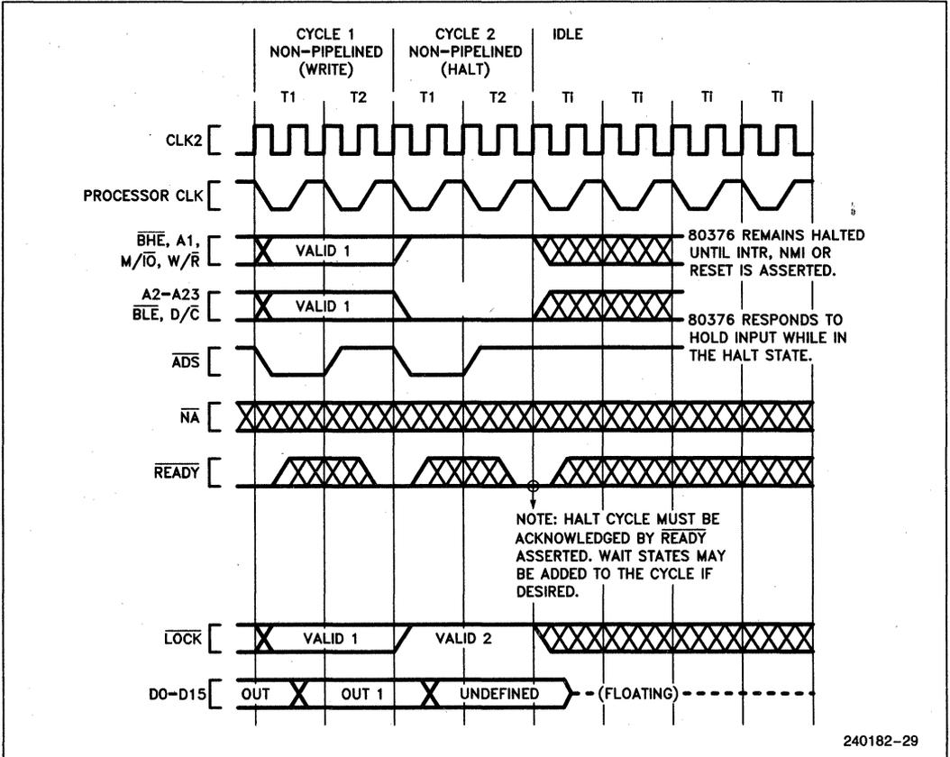
Figure 4.14. Example Halt Indication Cycle from Non-Pipelined Cycle
