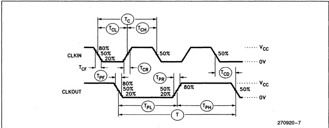
**Figure 5. Input and Output Clock Waveform**
