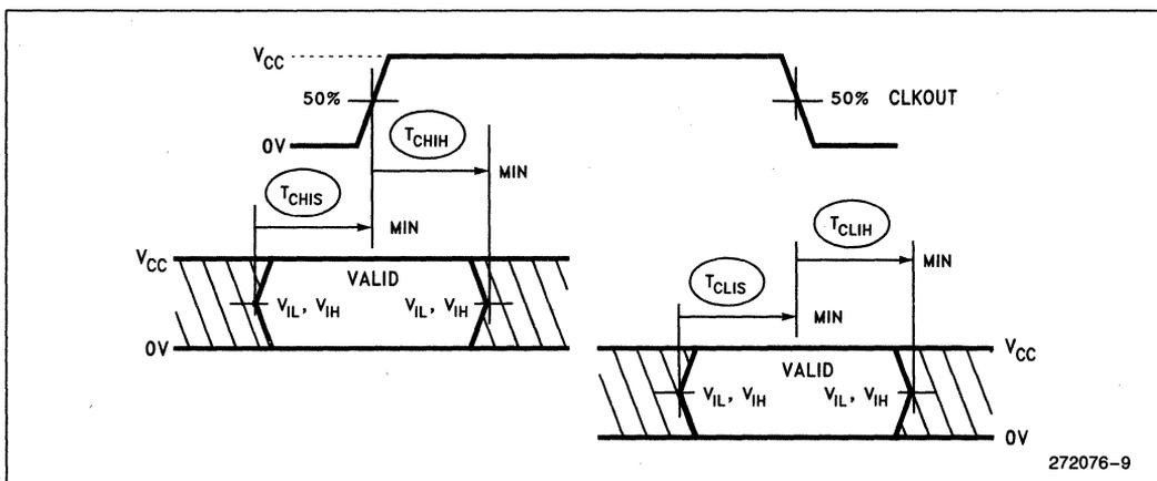
Figure 9. Input Setup and Hold
