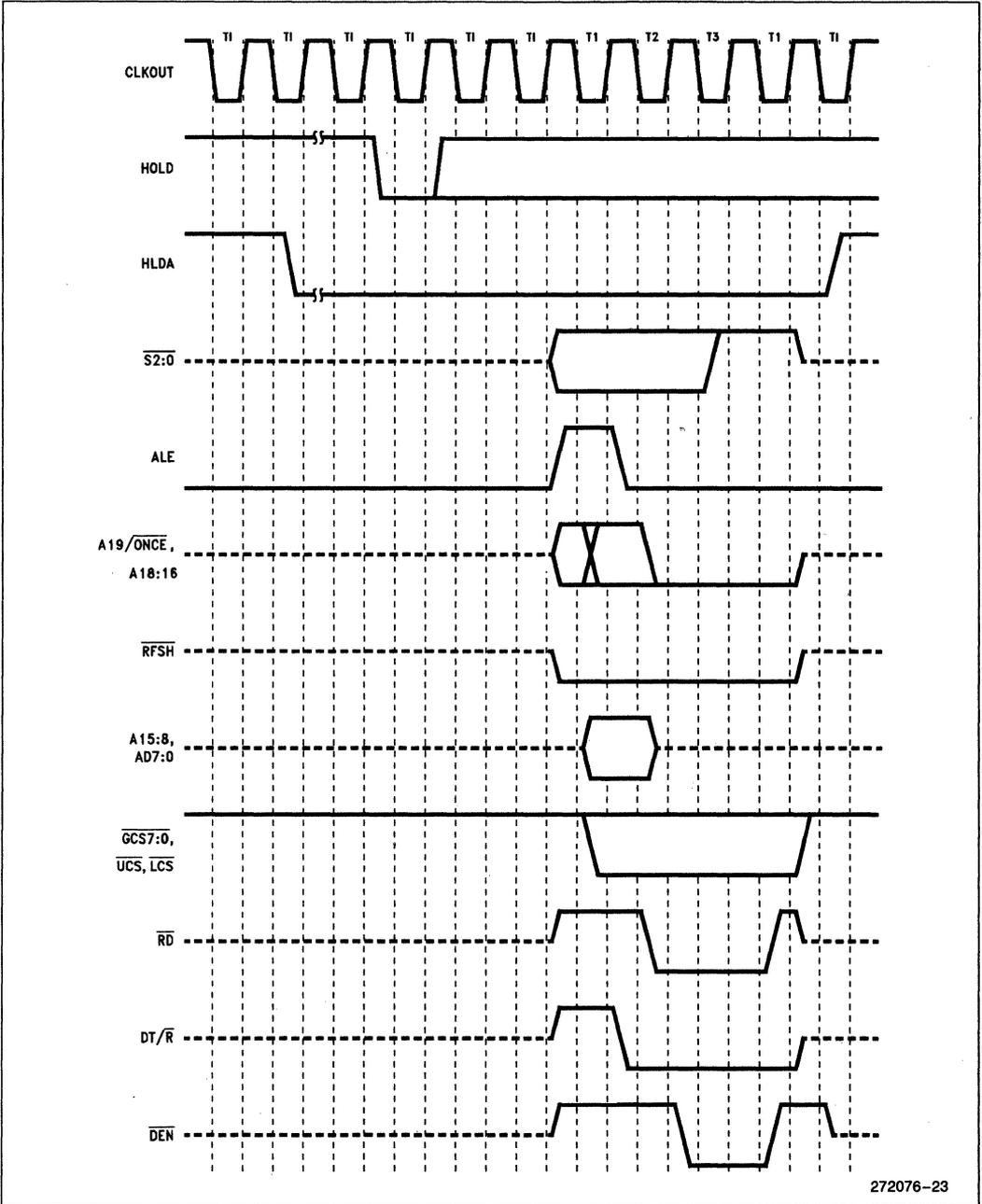
Figure 22. Refresh during HLDA Waveforms
