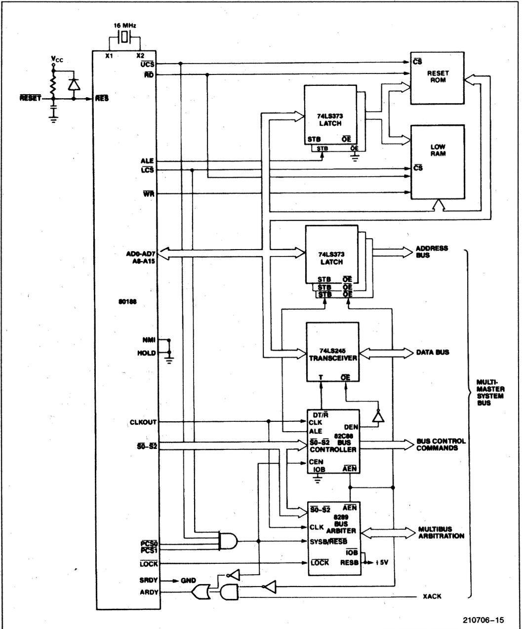
Figure 41. Typical 80188 Multi-Master Bus Interface
