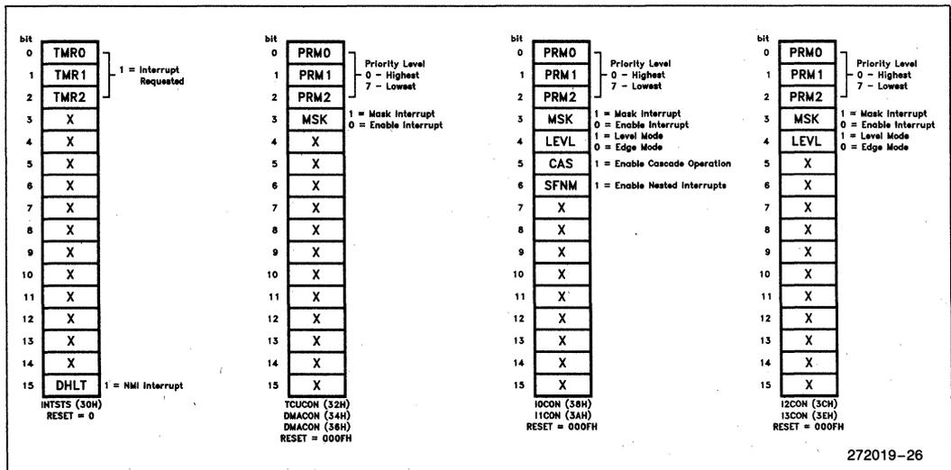
**Figure 24. Interrupt Control Unit Registers (Master Mode)**
