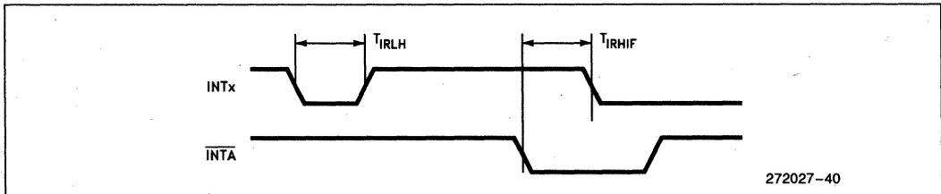
Figure 10. Relative Interrupt Signal Timings
