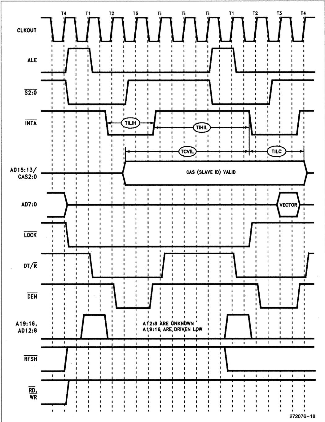
Figure 20. Interrupt Acknowledge Cycle Waveform
