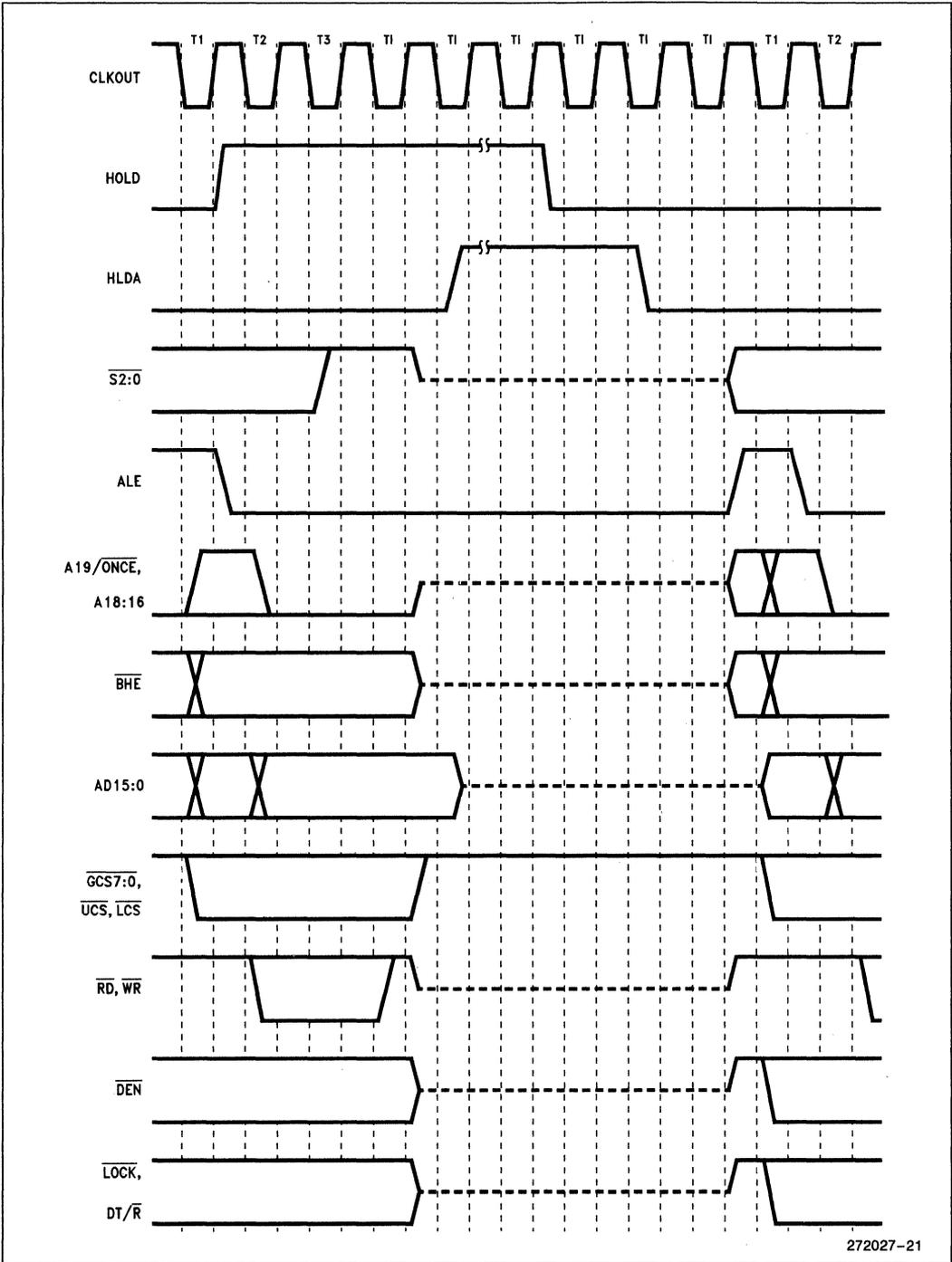
Figure 21. HOLD/HLDA Cycle Waveforms
