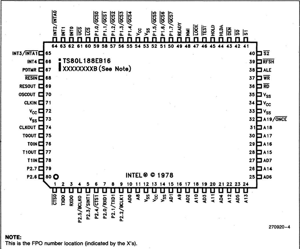
Figure 3. Quad Flat Pack Pinout Diagram
