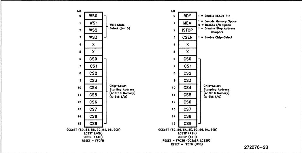
**Figure 32. Chip-Select Unit Registers**
