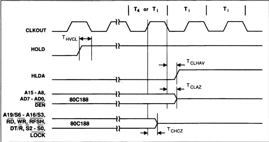
HOLD/HLDA WAVEFORMS (Leaving Hold)
