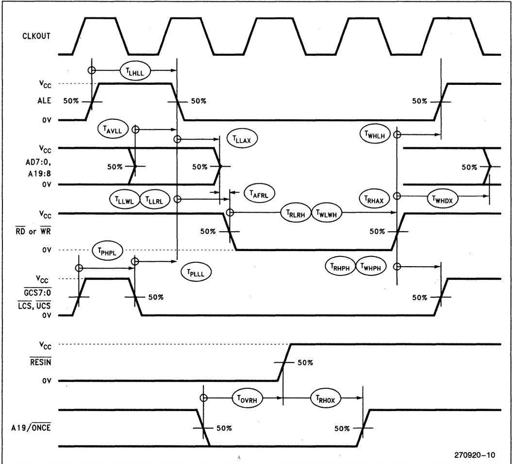
Figure 8. Relative Signal Waveform
