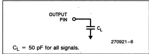
**Figure 4. AC Test Load**
