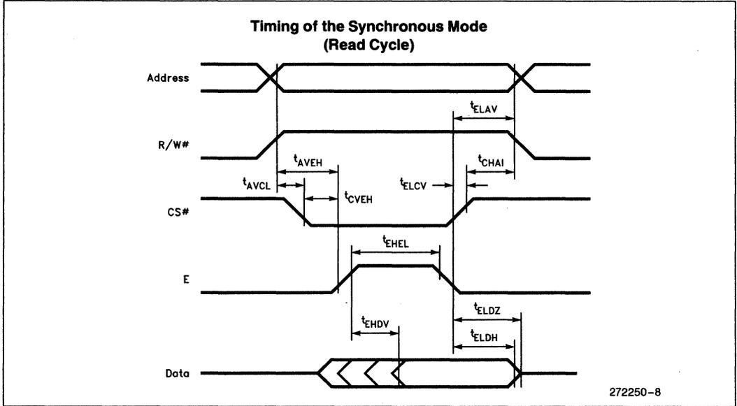
**A.C. Characteristics for 8-Bit Non-Multiplexed Synchronous Mode (Mode 3)**
