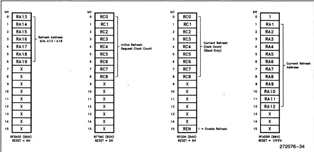
**Figure 33. Refresh Control Unit Registers**
