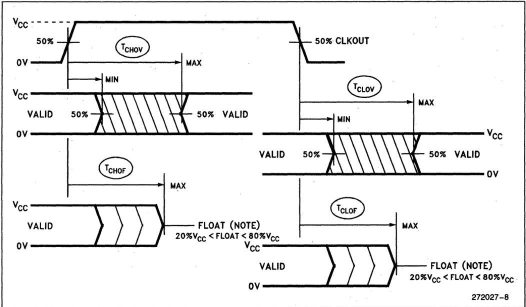
Figure 8. Output Delay and Float Waveforms
