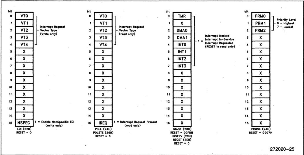
**Figure 23. Interrupt Control Unit Registers (Master Mode)**
