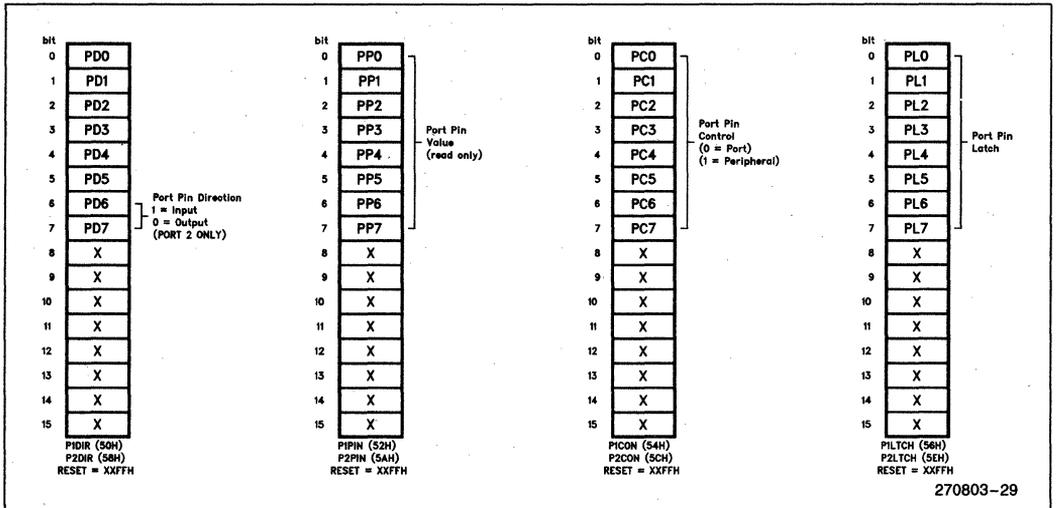
Figure 27. I/O Port Unit Registers
