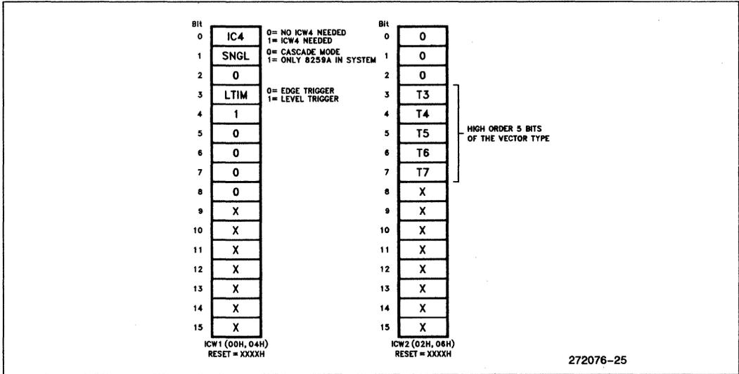
**Figure 24. 8259A Module Initialization Command Words (ICWs)**
