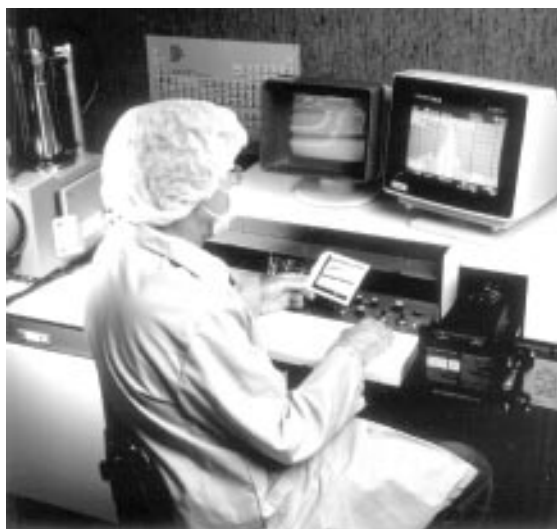
Scanning Electron Microscope with X-RAY Dispersive Analysis
