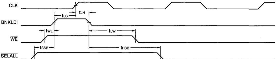
**SWITCHING WAVEFORMS: COEFFICIENT/CONTROL SIGNAL LOADING (METHOD II)**
