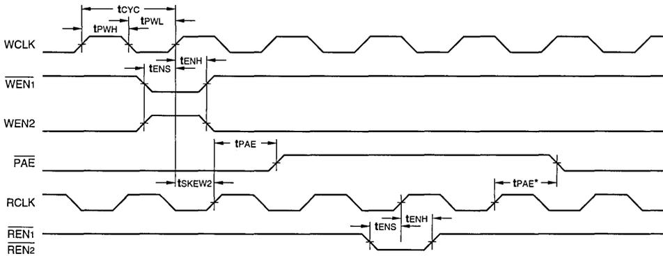
\*PAE is synchronized to the rising edge of RCLK, but in this case the PAE transition takes place in the next clock cycle.
