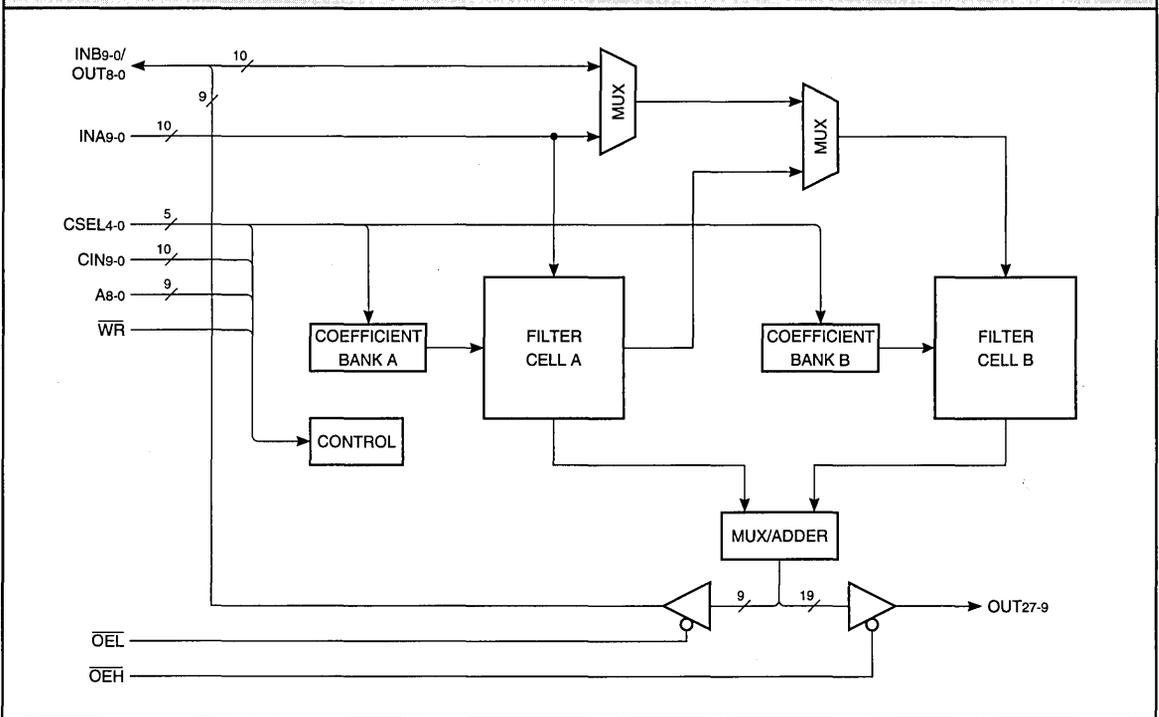
**FIGURE 1. LF43168 FUNCTIONAL BLOCK DIAGRAM**
