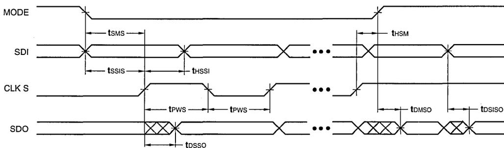
**SWITCHING CHARACTERISTICS — PIPELINE LOAD FROM SHADOW**
