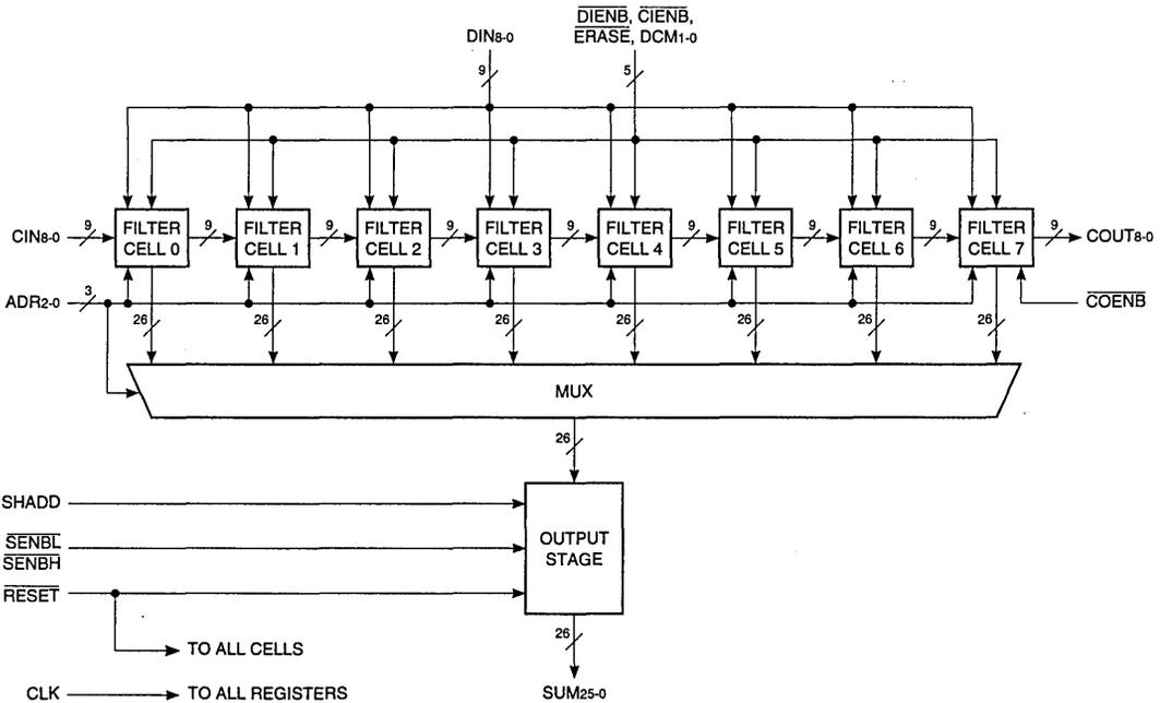
**FIGURE 1. FILTER CELL DIAGRAM**
