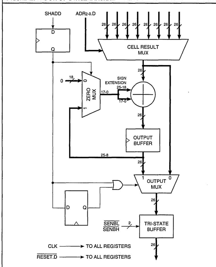
M REG0 and M REG1. The output of the multiplier is sign extended and is used as one of the inputs to the 26-bit adder. The output of the 26-bit accumulator provides the second input to the adder. Both the accumulator and T register are loaded simultaneously with the output of the adder.
