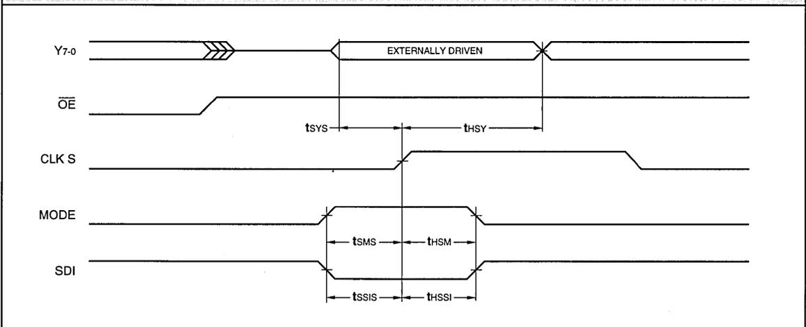
**SWITCHING CHARACTERISTICS — SHADOW READ VIA D PORT**
