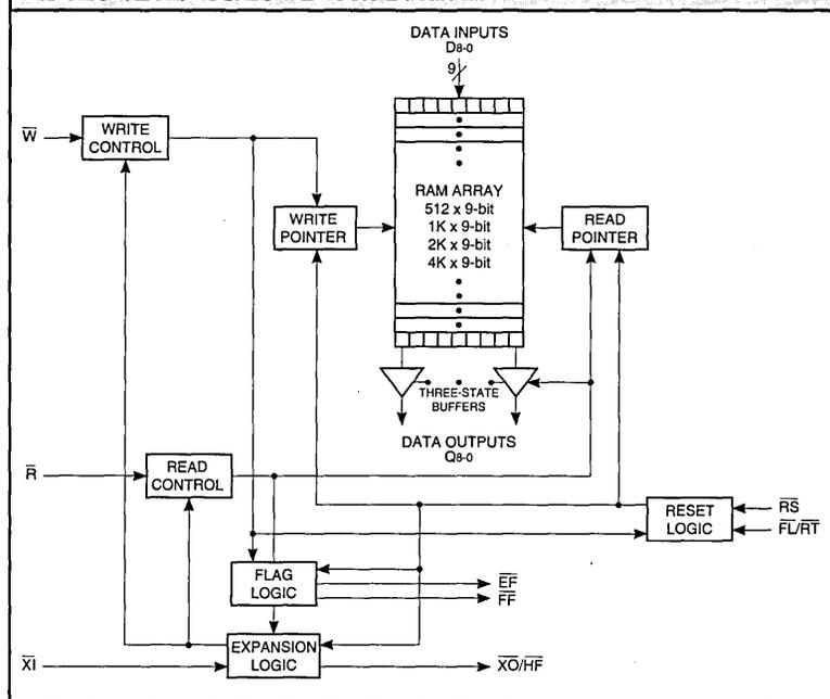
These FIFOs are designed to have the fastest data access possible. Even in lower cycle time applications, faster access time can eliminate timing bottlenecks as well as leave enough margin to allow the use of the devices without external bus drivers.
