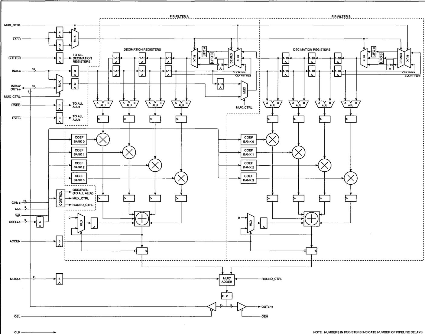
NOTE: NUMBERS IN REGISTERS INDICATE NUMBER OF PIPELINE DELAYS.
