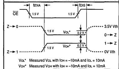
Vol\* Measured VOL with IOH = -10mA and IOL = 10mA
