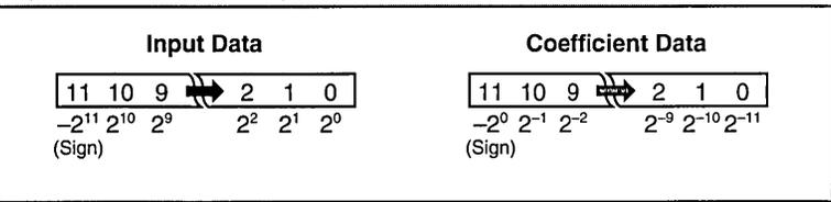
**FIGURE 3. ACCUMULATOR OUTPUT FORMATS**
