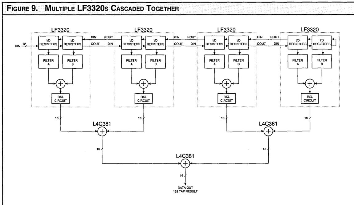
**FIGURE 9. MULTIPLE LF3320S CASCADED TOGETHER**
