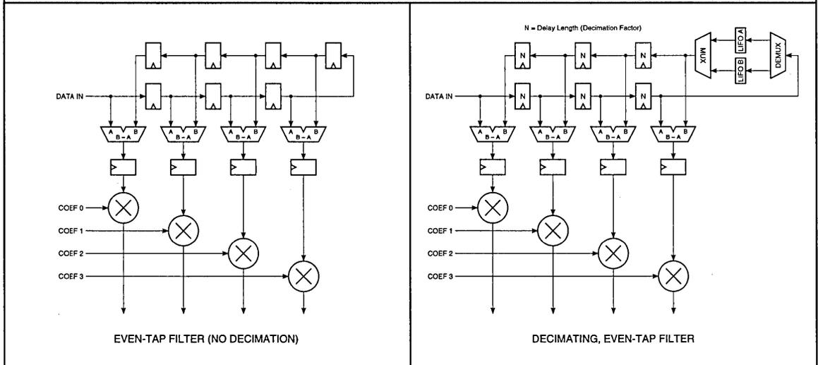
Figure 5 shows the two possible configurations when the device is programmed as a decimating, even-symmetric coefficient filter. The delay length of the decimation registers will be equal to the decimation factor that the device is programmed for. Since only four coefficients (effectively eight) can be sent to the filter multipliers
