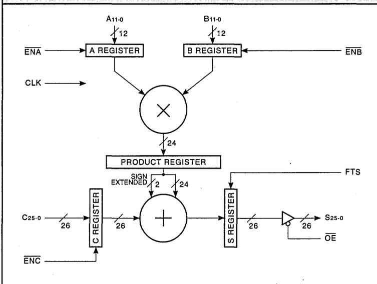
**FIGURE 1. FLOW DIAGRAM FOR 5-TAP FIR FILTER**
