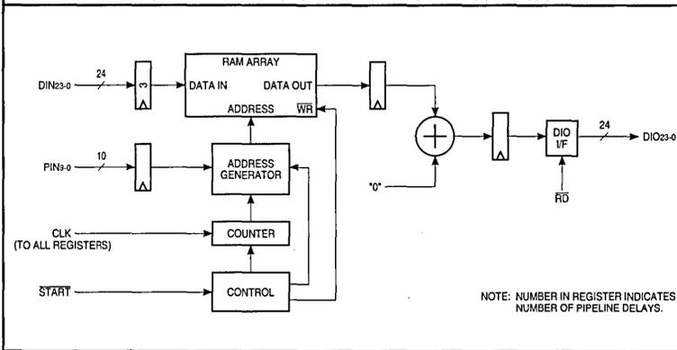
DIO23-0 (if  $\overline{RD}$  is LOW). If Look Up Table Write Mode was used to load the memory array, it is important to wait until the third clock cycle after  $\overline{START}$  goes HIGH to input data on PIN9-0 to insure that all data is written into the memory array before any reading is done.
