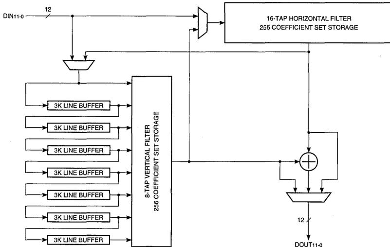
**FIGURE 1. LF3310 FUNCTIONAL BLOCK DIAGRAM**
