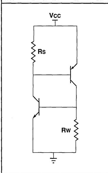
the die, reducing the values of  $R_S$  and  $R_W$ . This makes it more difficult to develop the base drive necessary to regenerate the latchup condition.
