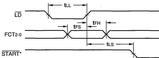
\*there must be at least one rising edge of CLK between the rising edge of LD and the falling edge of START.
