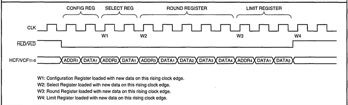
vertical filter. Each register is 32 bits wide. HRSL3-0 and VRSL3-0 determine which horizontal and vertical round registers respectively are used for rounding.
