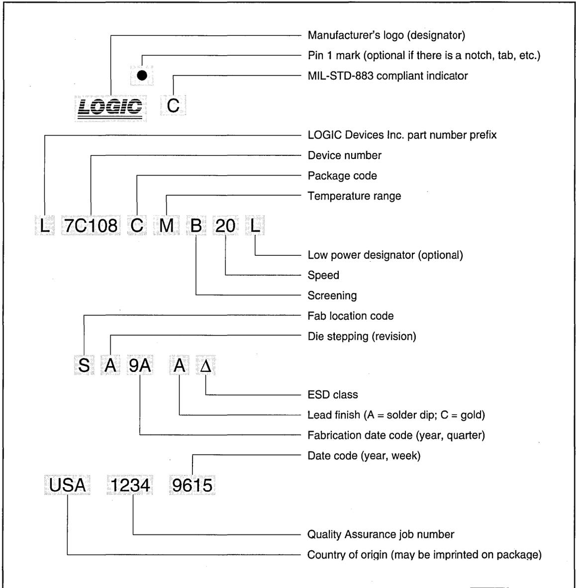
NOTE: Package marking may occur on top and bottom of package due to space limitations
