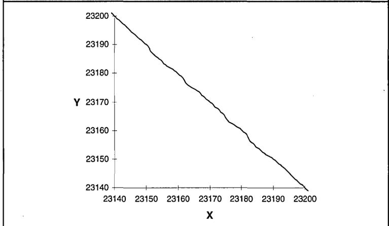
**FIGURE 3. CIRCLE TEST RESULT NEAR 45° (24-BIT INTERNAL PROCESSOR)**
