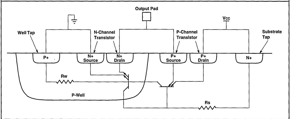
**FIGURE 2. EQUIVALENT CIRCUIT FOR LATCHUP PATH**
