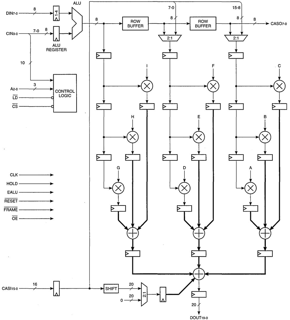
NOTE: NUMBERS IN REGISTER INDICATE NUMBER OF PIPELINE DELAYS.
