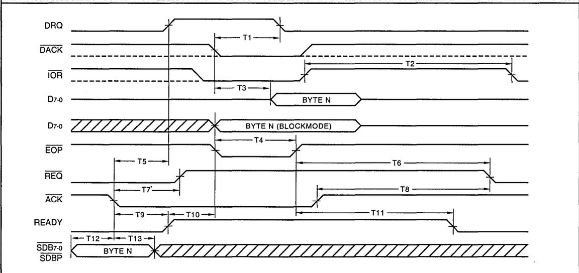
\*Data must be held on the SCSI bus until  $\overline{\text{REQ}}$  becomes False
