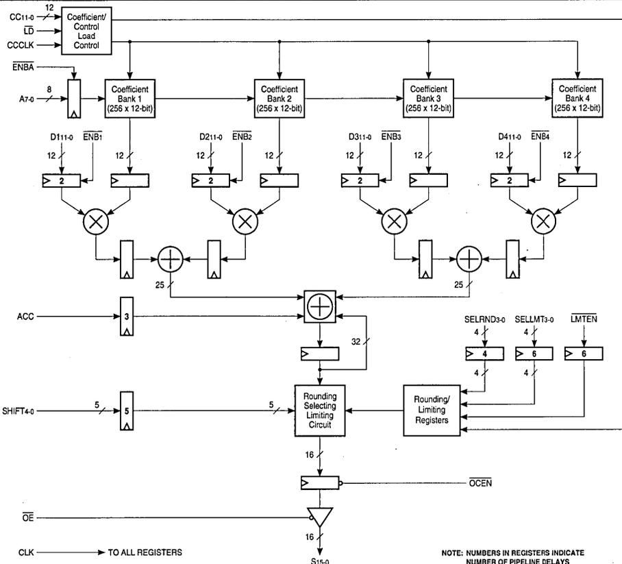
NOTE: NUMBERS IN REGISTERS INDICATE NUMBER OF PIPELINE DELAYS
