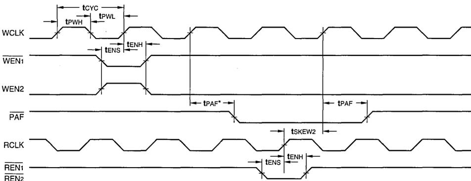
\*PAF is synchronized to the rising edge of WCLK, but in this case the PAF transition takes place in the next clock cycle.
