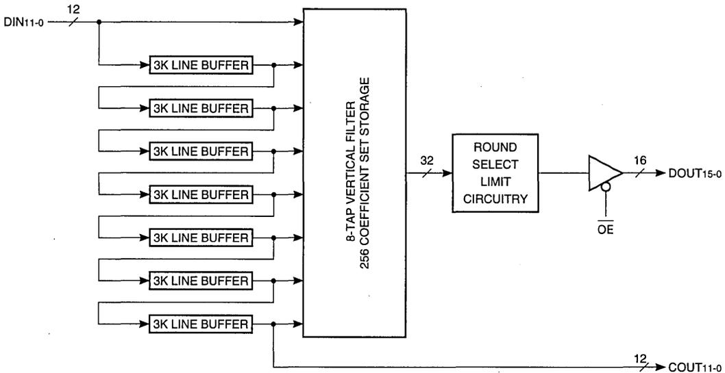
**FIGURE 1. LF3330 FUNCTIONAL BLOCK DIAGRAM**
