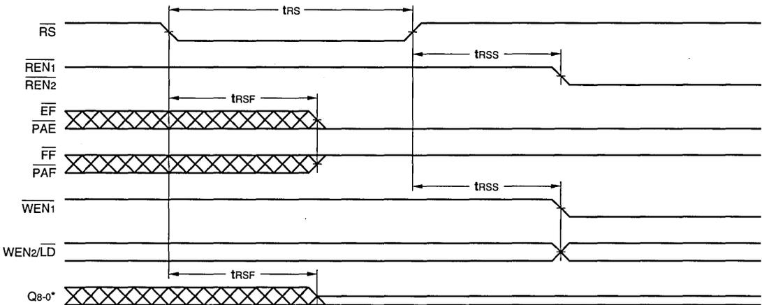
\*after reset, Q8-0 will be LOW if  $\overline{OE} = 0$  and in HIGH IMPEDANCE if  $\overline{OE} = 1$ .
