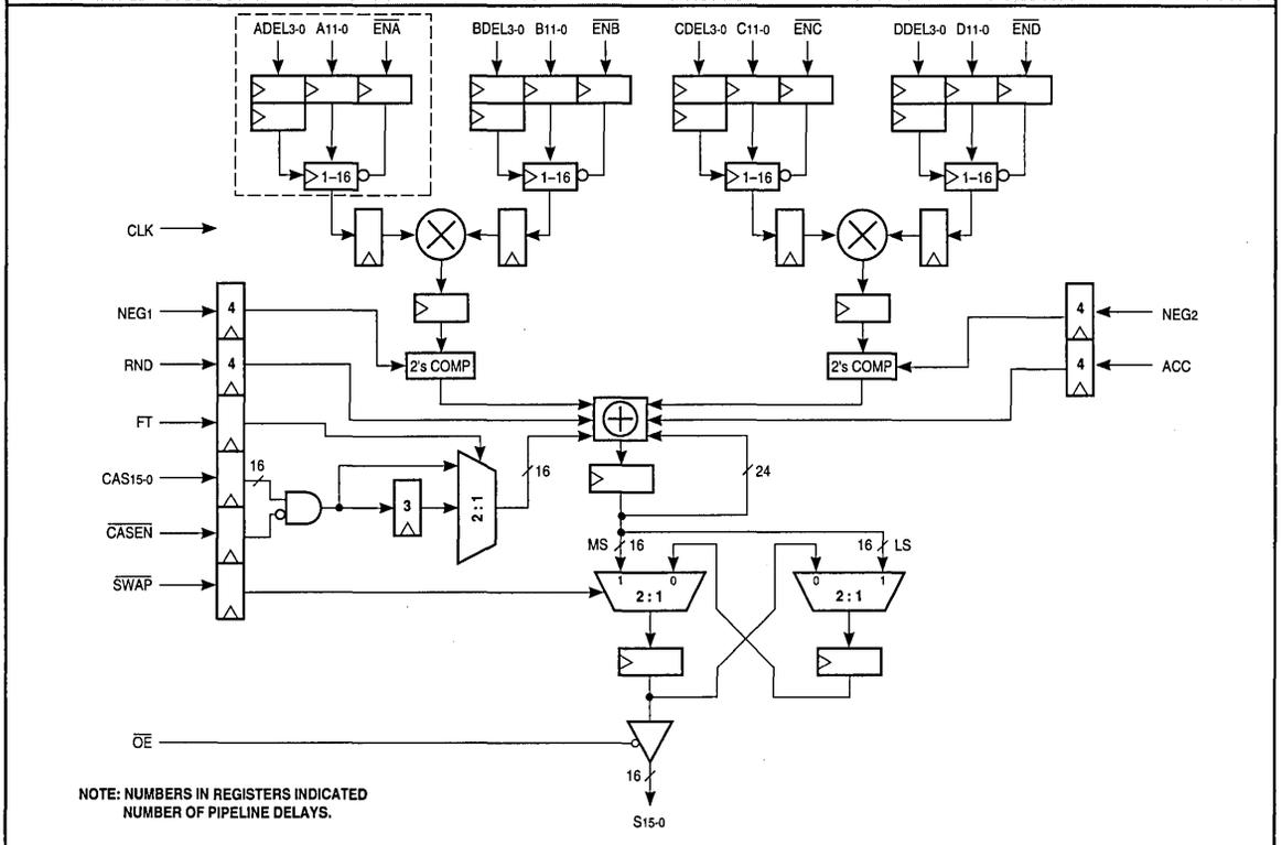
synchronous operation between the incoming data and all available control functions. The LF2249 operates at a clock rate of 40 MHz over the full commercial temperature and supply voltage ranges.
