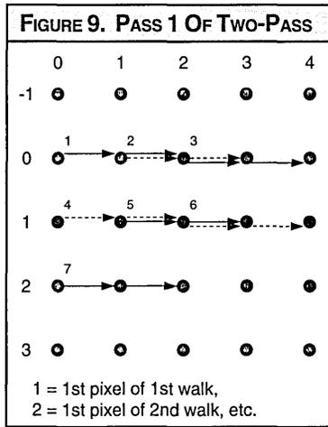
pixel address of the second line is determined by adding  $dx/dv$  to  $x_0$  and by adding  $dy/dv$  to  $y_0$ . Since the first pixel of the first pixel walk on the second line should be (0,1),  $dx/dv$  is selected to be 0 and  $dy/dv$  is selected to be 1. Second order differential terms are not used in this filter and are therefore set to 0.
