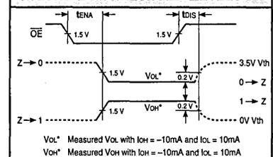
Vol\* Measured Vol with IOH =  $-10\text{ mA}$  and IOL =  $10\text{ mA}$
