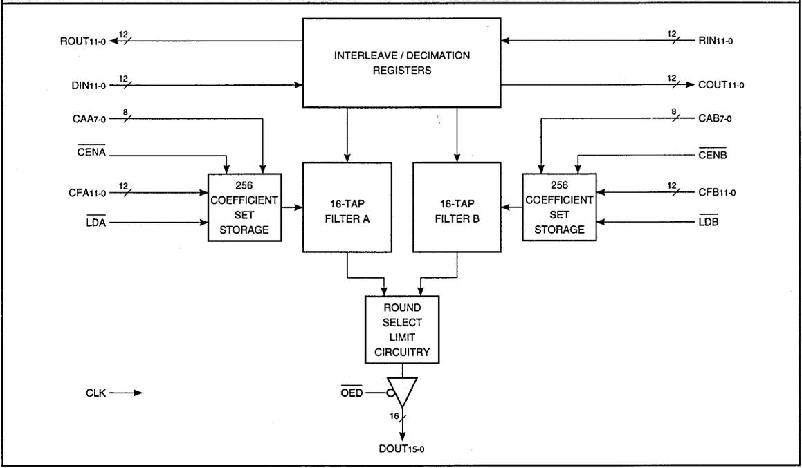
**FIGURE 1. LF3320 FUNCTIONAL BLOCK DIAGRAM**
