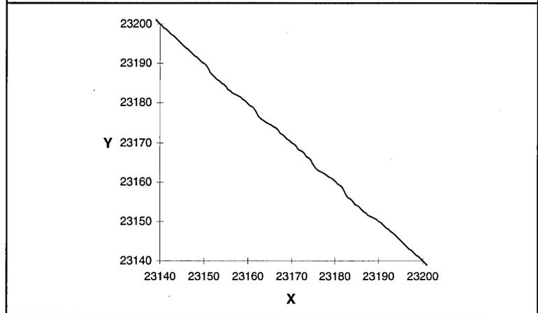
**FIGURE 4. CIRCLE TEST RESULT NEAR 45° (24-BIT INTERNAL PROCESSOR)**
