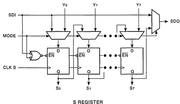
CLK P. In diagnostic applications, this allows a data value input via serial scan to be loaded into the active data path of the machine.
