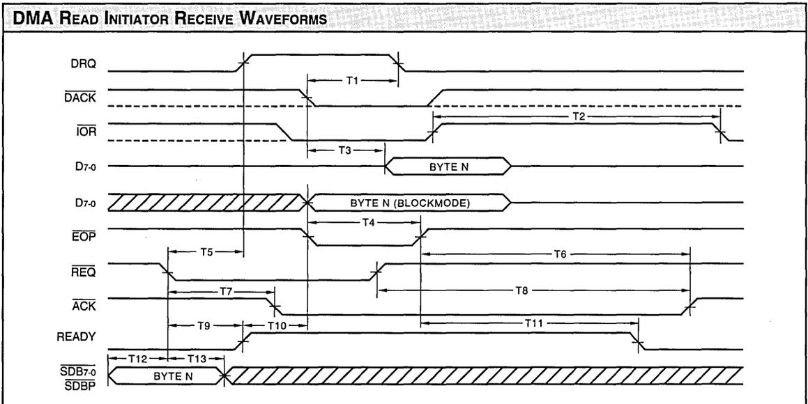
\*Data must be held on the SCSI bus until  $\overline{\text{ACK}}$  becomes True
