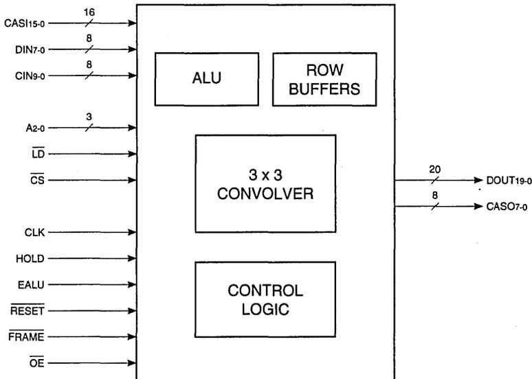
**FIGURE 2. LF48908 FUNCTIONAL BLOCK DIAGRAM**
