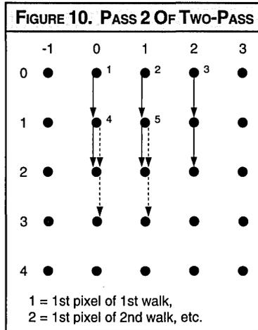
selected, the first pixel address of the second line is determined by adding  $dx/dv$  to  $x_0$  and by adding  $dy/dv$  to  $y_0$ . Since the first pixel of the first pixel walk on the second line should be (0,1),  $dx/dv$  is selected to be 0 and  $dy/dv$  is selected to be 1. Second order differential terms are not used in this filter and are therefore set to 0.
