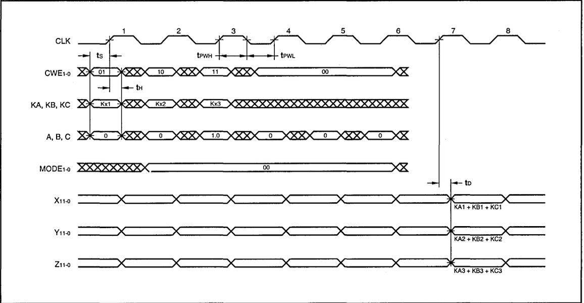
**SWITCHING WAVEFORMS: 9-TAP FIR FILTER — MODE 01**
