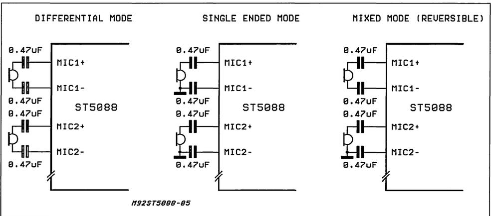
The 4 connection modes (since the MIXED MODE is symmetrical with respect to MIC1 and MIC2) allow one microphone at a time to be selected via the  $V_s$  bit (bit 7 of Control Register CR4).
