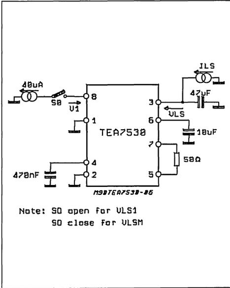
Figure 6: Loudspeaker Amplifier: Gain/Distortion/Output Offset
