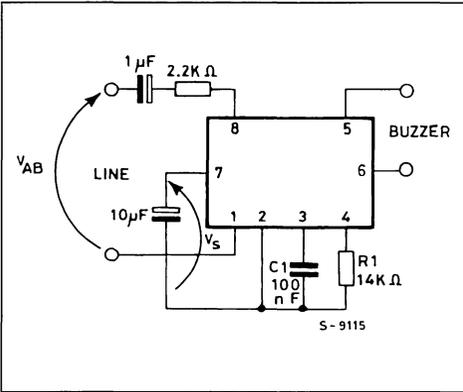
**Figure 2** : Typical Application with Balanced Output.
