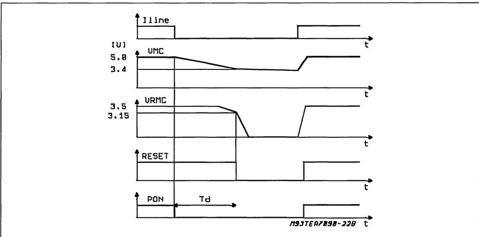
$T_D$  is fixed by the VMC value, C10 on VMC, and the ST6 current consumption.
