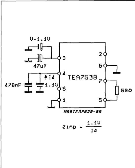
Figure 8: Anti-loading Feedback System at G = GATT
