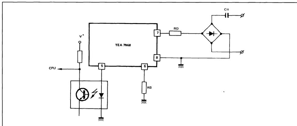
Three external components affect the characteristic of the ring detection circuit. The capacitor  $C_R$  provides the DC isolation from the line.
