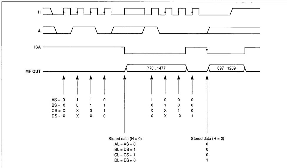
Notes : 1. With ISA at logic 0, H, A, B, C and D signals cannot modify the generated DTMF pair. As a result, in serial operating mode, it is possible to enter AS, BS, CS and DS data while another DTMF pair is being generated.
