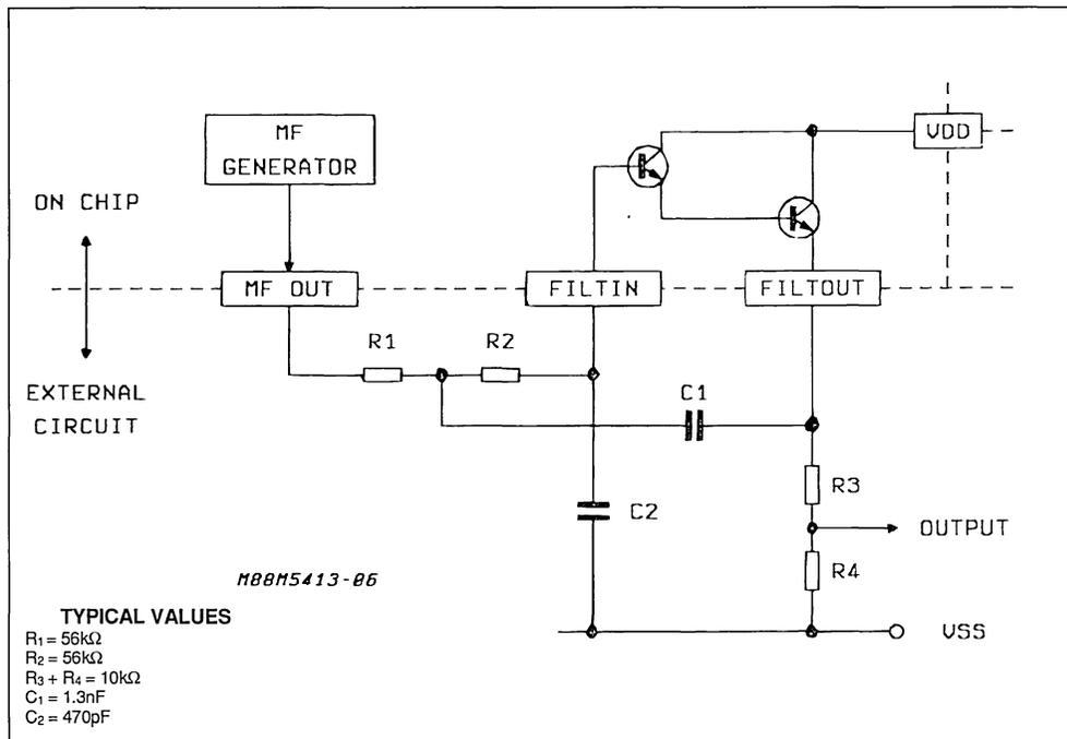
The filter components shown have been chosen to give a second order Butterworth response with a cut-off frequency of about 3.5kHz. The pass-band insertion loss is nominally 0.5dB.
