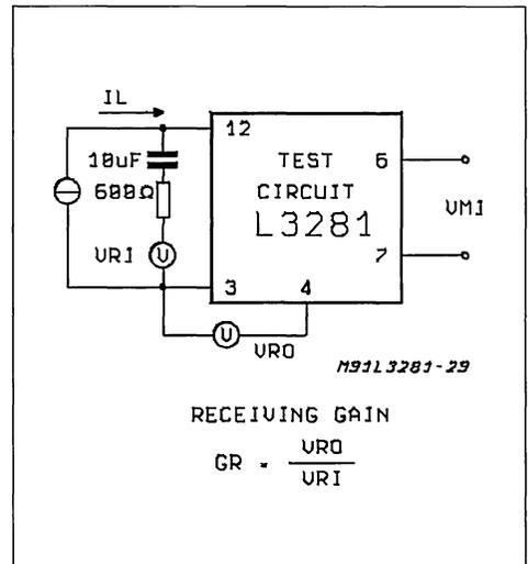
**ELECTRICAL CHARACTERISTICS**  $I_L = 20$  to  $100\text{mA}$ ;  $R_4 = (51\Omega // \text{diode}) + 33\Omega$ ;
