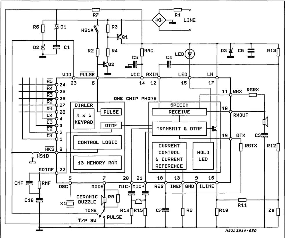
When mated with a tone ringer, a complete telephone can be produced with just two ICs.
