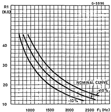
$$R_1 \approx \frac{3.56 \times 10^4}{F_1 \text{ (HZ)}} \times (1 - 0.12 \times \ln \frac{F_1}{2543})$$
