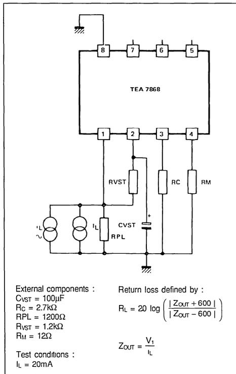
Figure 3 : Ring Detection Level and Impedance.
