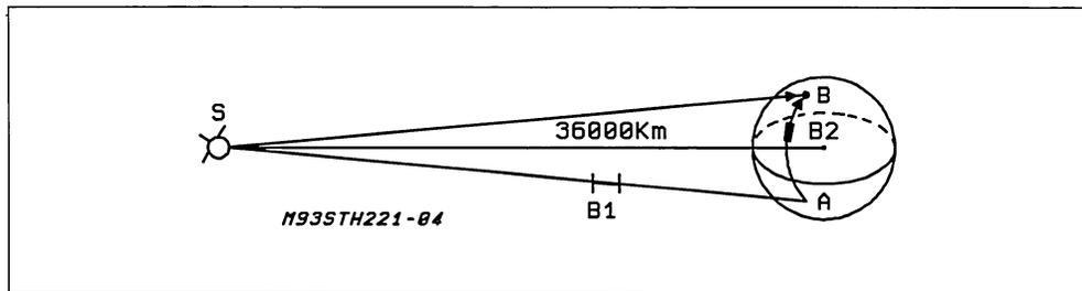
B1 channel path ASB 300000Km/s Delay  $\frac{3600 \cdot 2}{300000} = 0.240s$ .
