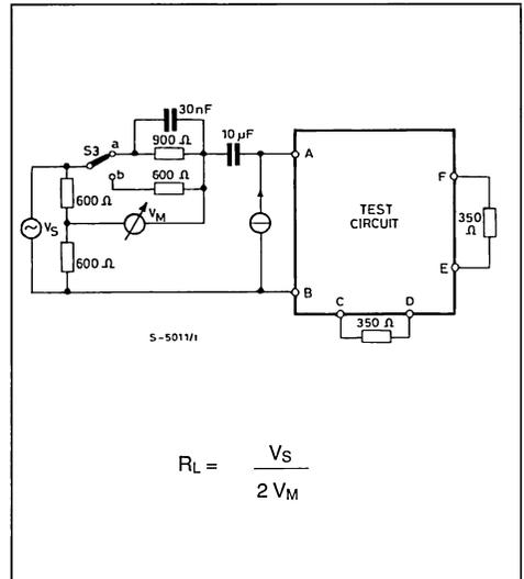
**ELECTRICAL CHARACTERISTIC**(refer to the test circuit,  $T_{amb} = 25^{\circ}\text{C}$ ,  $f = 300\text{Hz}$  to  $3400\text{Hz}$ , S1, S2 in "a" unless otherwise specified)
