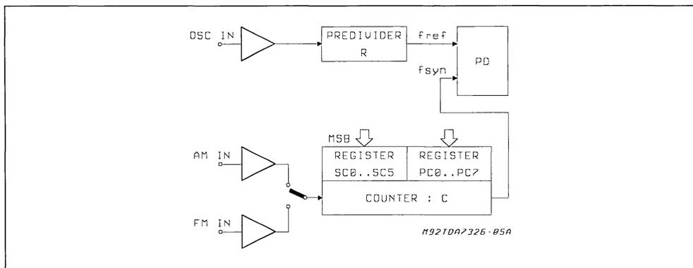
The AM signal is directly applied to the 14 bit static divider 'C'. This divider is controlled by both SC and PC registers.
