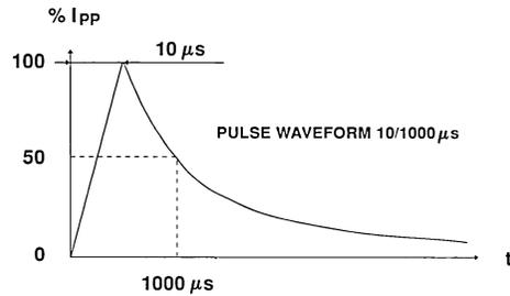
Note 1 : For surges greater than the maximum values, the diode will present a short-circuit Anode - Cathode
