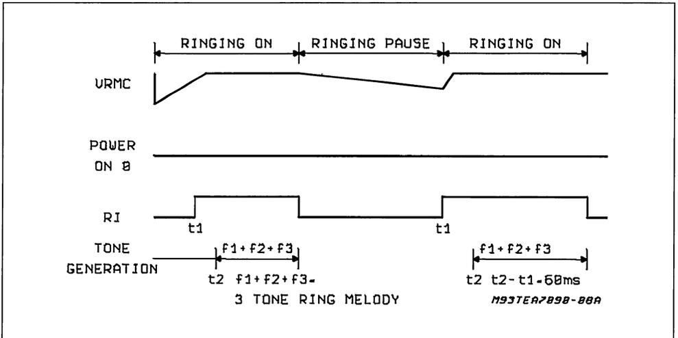
During the delay  $t_2 - t_1$ , the microcontroller can analyse the line ring frequency and then sends to the serial data input the code corresponding to the chosen ringing output level.
