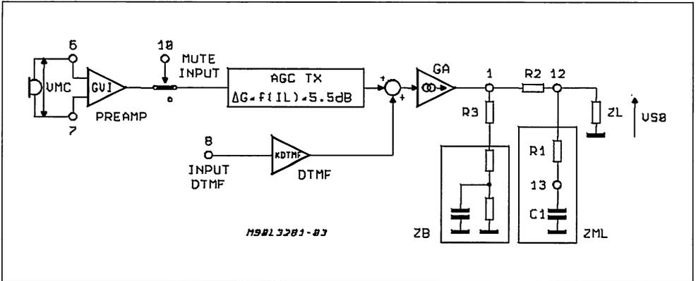
**Figure 9:** Equivalent Receiving Circuit.
