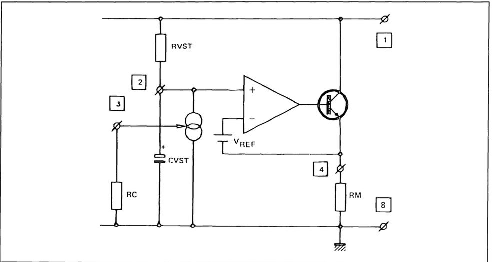
The DC characteristic is a zener characteristic which slope is fixed by  $R_M$  (see Figure 8). The voltage over the circuit (pin 1) is fixed via a current source driven through  $R_{VST}$ . The value of this current source is fixed by the external resistor  $R_C$  with the formula :
