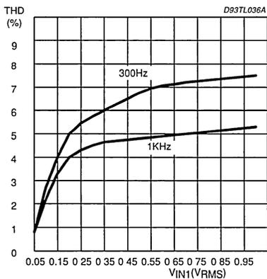
Figure 4: IN3 and IN2 Channels – Distortion
