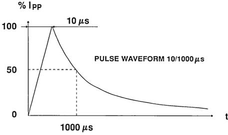
**Note 1 :** For surges greater than the maximum values, the diode will present a short-circuit Anode - Cathode.
