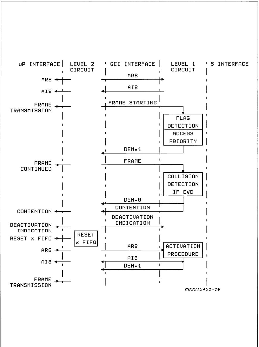
Figure 12: HDCL Frame Transmission Procedure in D Channel
