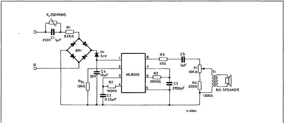
**Figure 11 : ML8204 Test Circuit (power supply transient).**
