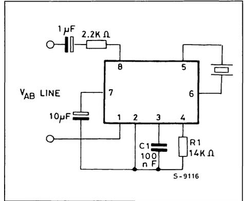
**Figure 3** : Application Compatible with LS1240 (single ended output).
