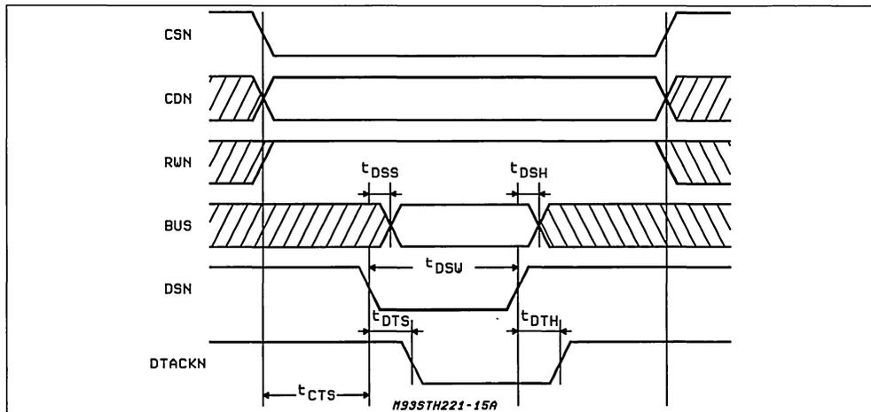
Figure 15: Transmitter Start Timing.
