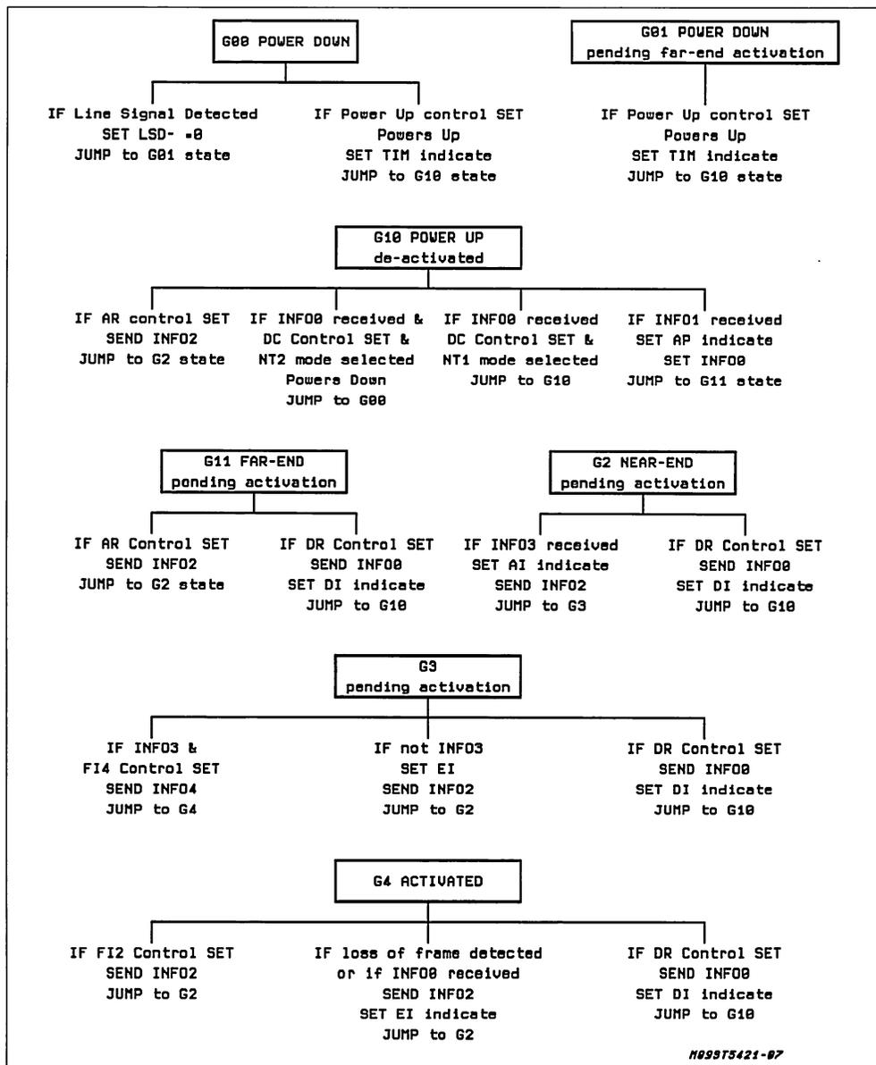
FSa, BCLK and MCLK must be present at this time. When activation is initiated by the far-end, SID-GCI being in the Power Down state, a Line Signal Detector circuit pulls low LSD- pin, which can be used to wake up the system. A power Up procedure must be then be issued allowing identification of received signal ie, INFO1 or INFO2. The appropriate procedure is then followed according to I.430.
