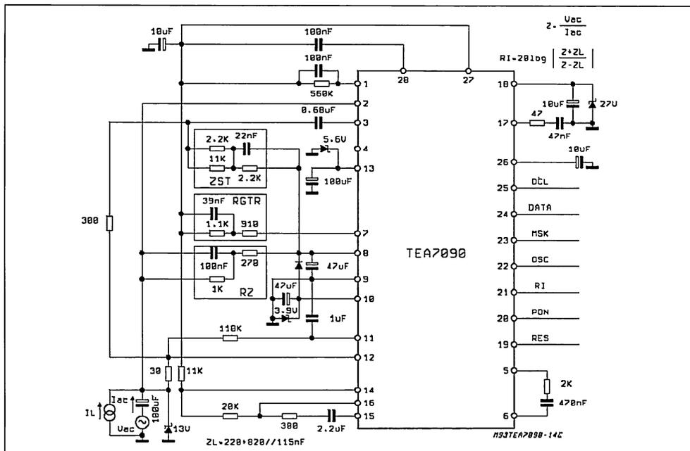
Figure 19: Test 8a Circuit Vthri
