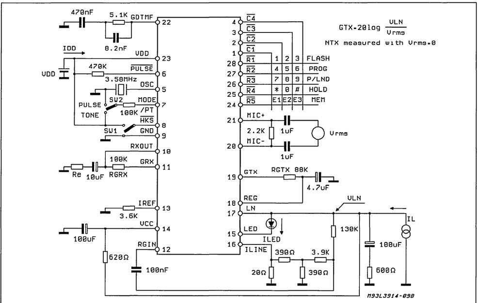
Figure 9: Typical Application Circuit.
