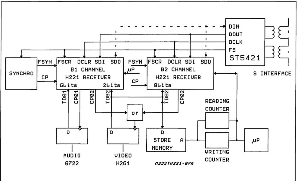
Figure 8: Application Interface Configuration can change every 20ms.
