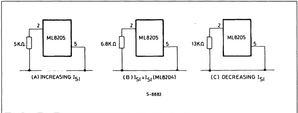
Figure 9a : I-V Slope Change Due to  $R_{SL}$ .
