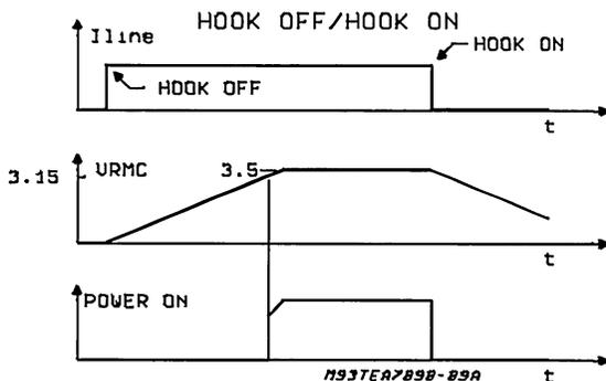
**Figure 7:** Timing PULSE/FLASH MODE
