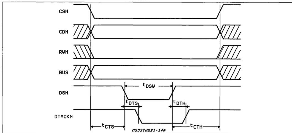
**Figure 14: CPU Read Cycle**
