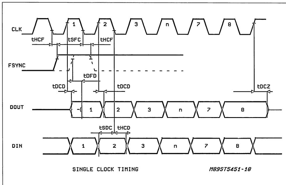
Figure 16: Non-multiplexed  $\mu$ P bus timing
