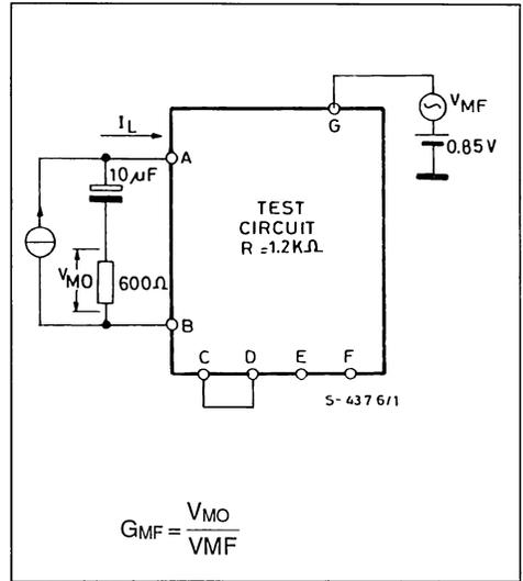
**ELECTRICAL CHARACTERISTICS** (refer to the test circuits, S1, S2 in (a),
