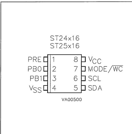
The ST25x16 operates with a power supply value as low as 2.5V. Both Plastic Dual-in-Line and Plastic Small Outline packages are available.
