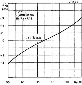
**Figure 8 :** Sending Gain Variation vs. Rx Value (see note for R6 and R6').
