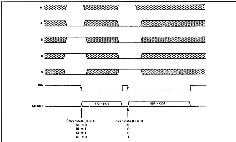
Note : If the circuit operates permanently in parallel mode, then the H input may be left floating (internally pulled-up to V<sup>+</sup>) or tied to logic 1. With ISA at logic 0, H, A, B, C, and D inputs cannot modify the generated DTMF pair.
