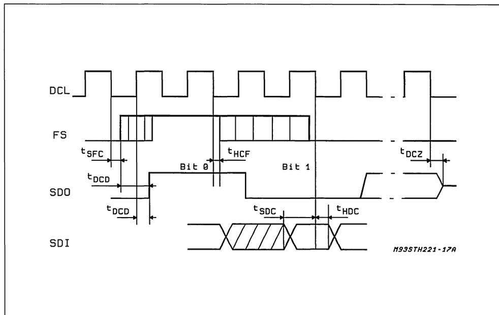
Figure 17: Application Side Signals.
