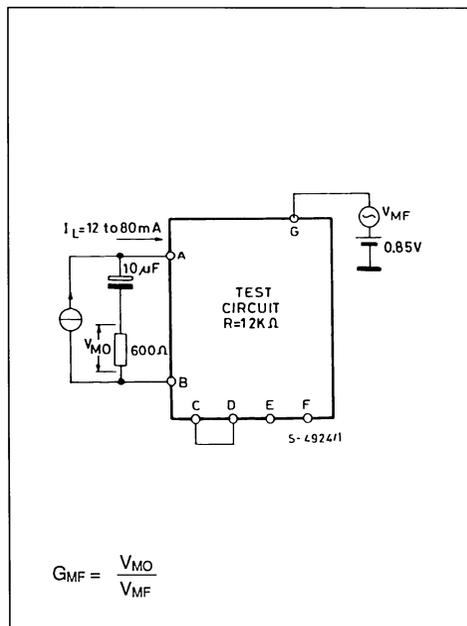
**ELECTRICAL CHARACTERISTICS** (refer to the test circuits,  $V_G = 1$  to 2V,  $I_L = 12$  to 80mA, S1, S2 and S3 in (a),  $T_{amb} = -25$  to  $+50^\circ\text{C}$ ,  $f = 200$  to 3400Hz, unless otherwise specified)
