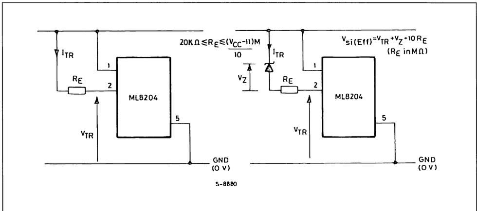
Oscillation of the ML8204 may be inhibited for voltages in the range  $V_{si} < V_s \leq V_{s(max)}$  by sinking the current from D<sub>1</sub>, starving Q<sub>1</sub> of base current. This is achieved by either a) grounding pin 2 (fig. 6a), or b) applying a voltage  $V_{INH}$  via a resistor  $R_1$  to pin 2 (fig. 6b) to ensure that :
