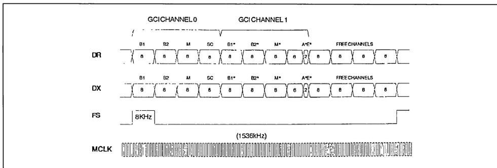
appropriate. During the assigned time slot, Dx output shifts data out from the voice data register on the rising edges of MCLK. Serial voice data is shifted into DR input during the same time slot on the falling edges of MCLK.
