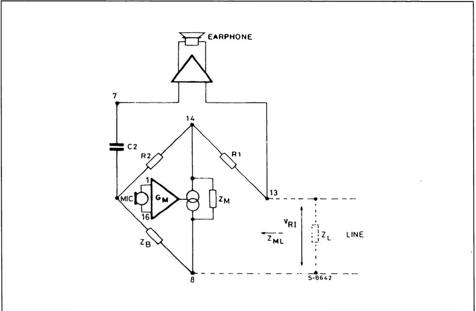
Figure 11 : Anticlippping Application.
