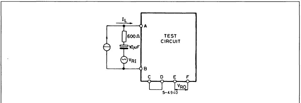
**ELECTRICAL CHARACTERISTICS** (Refer to test circuits,  $T_{amb} = -25$  to  $+50^{\circ}\text{C}$ ,  $f = 200$  to  $3400\text{Hz}$ ,  $I_L = 15$  to  $100\text{mA}$ ,  $R_7 = 17.3\text{k}\Omega$ ,  $R_8 = 17.1\text{k}\Omega$ ,  $S_1$  in A,  $S_2$  in A, unless otherwise specified)
