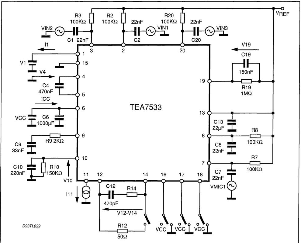
Figure 1: IN1 Channel - AGC Gain (Typical)
