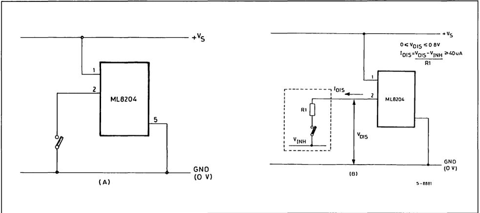
Figure 7a : Gating the ML8204 from CMOS.
