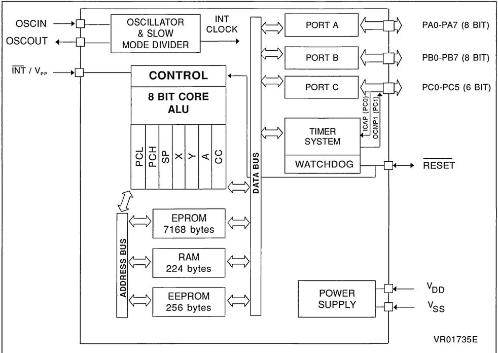
The EPROM ST72E94 may be used for the prototyping and the pre-production phases of development, can be configured as either a standalone microcontroller with 7K bytes of on-chip ROM, either as a microcontroller able to manage external memory.
