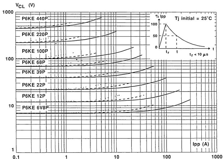
**Note :** The curves of the figure 3 are specified for a junction temperature of 25 °C before surge.
