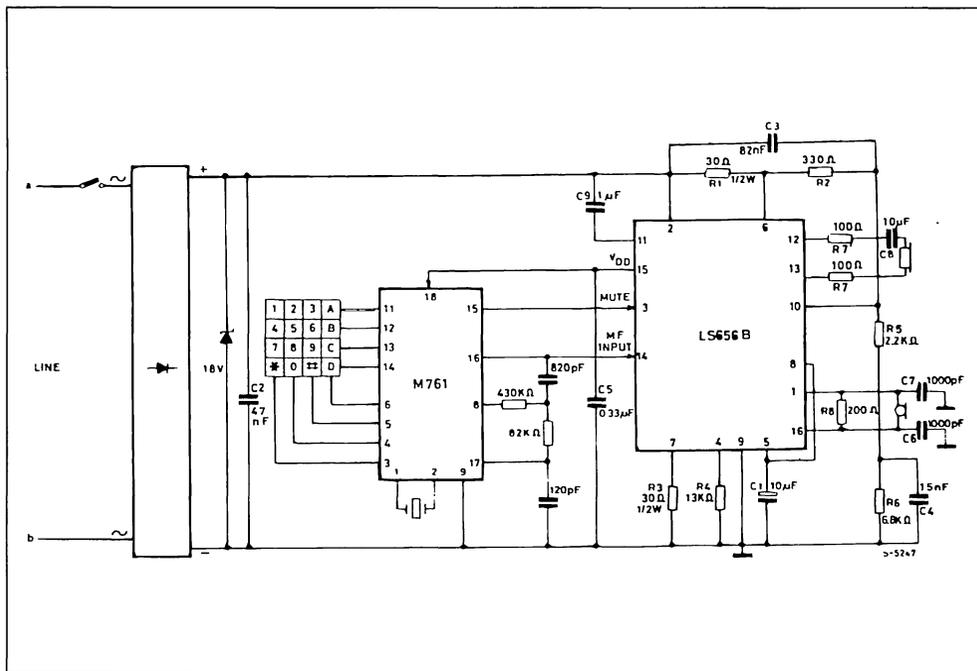
Figure 11 : Application Circuit with Multifrequency (Europe I STD).
