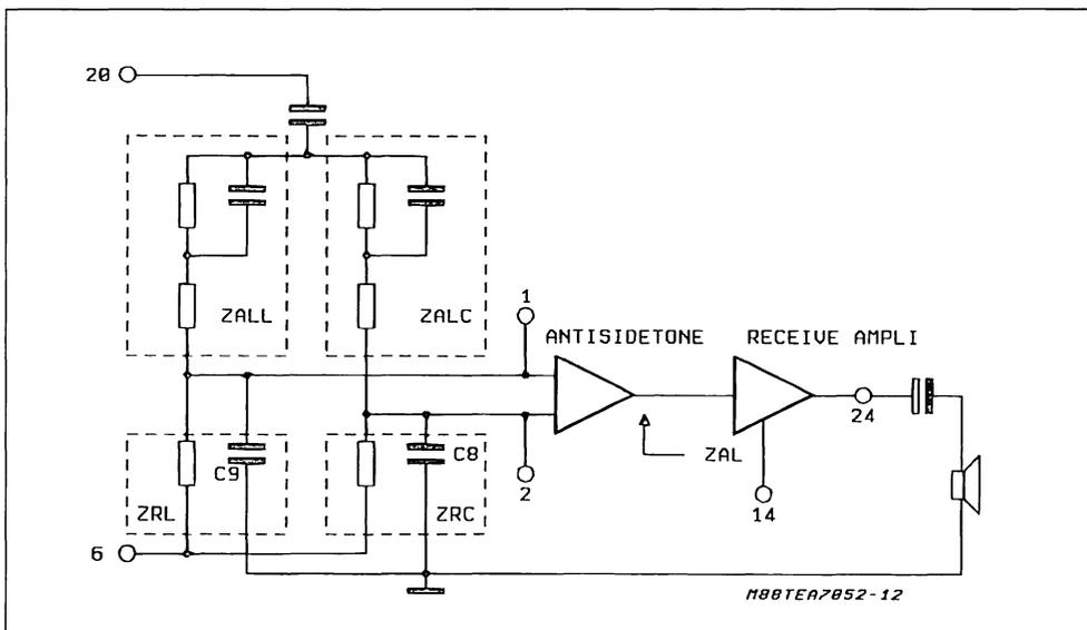
3.1. A.G.C. IN RECEIVE. As described for the transmission chain, also the receiving gains  $G_r$ , from pins 1 and 2 to pin 24, have a reduction of 6dB when  $I_{line}$  moves from 27mA to 42mA.
