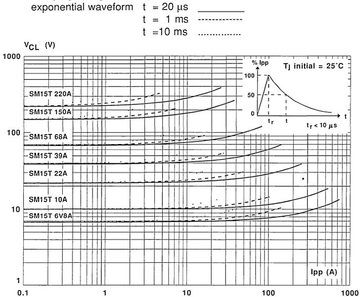
**Note :** The curves of the figure 3 are specified for a junction temperature of  $25^\circ\text{C}$  before surge. The given results may be extrapolated for other junction temperatures by using the following formula :  $\Delta V \text{ (BR)} = \alpha T \text{ (V(BR))} \cdot [T_a - 25] \cdot V \text{ (BR)}$ . For intermediate voltages, extrapolate the given results
