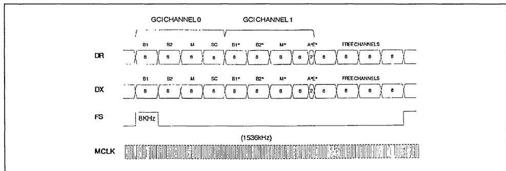
appropriate. During the assigned time slot, Dx output shifts data out from the voice data register on the rising edges of MCLK. Serial voice data is shifted into DR input during the same time slot on the falling edges of MCLK. Dx is in the high impedance Tristate condition when in the non selected time slots.
