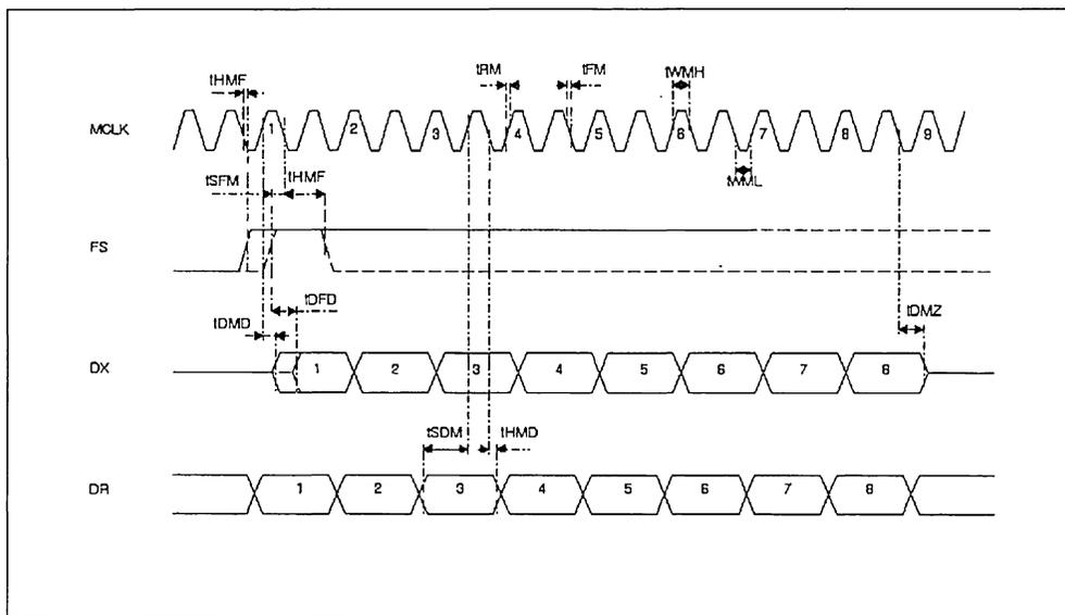
Serial Control Timing (MICROWIRE MODE)
