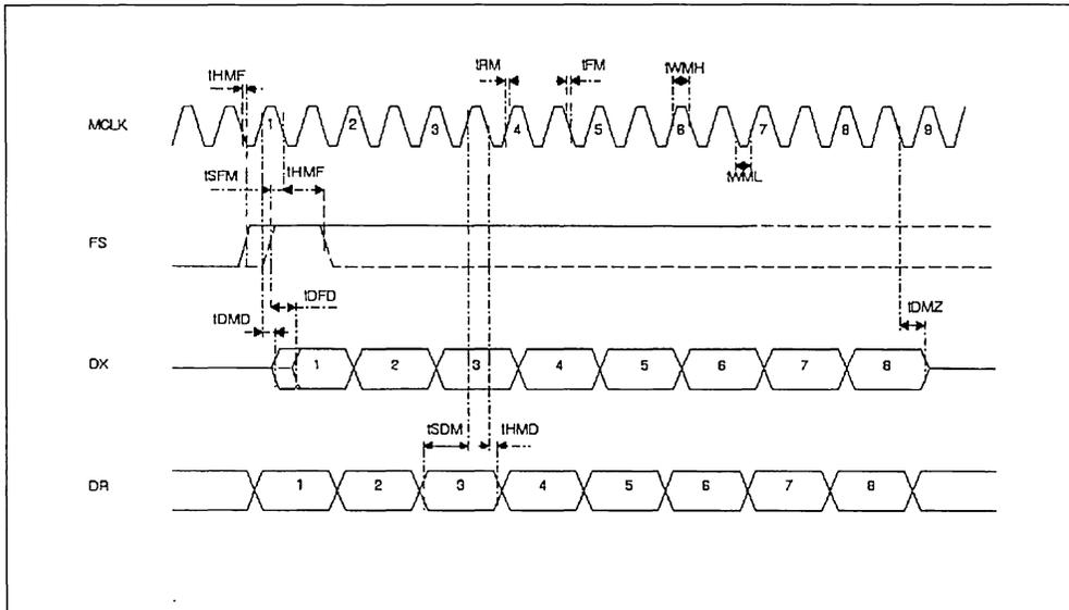
Serial Control Timing (MICROWIRE MODE)
