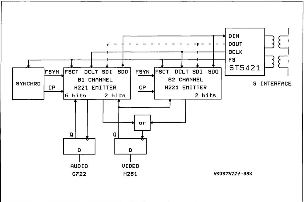
Figure 7: B1 channel is slower than B2 channel.
