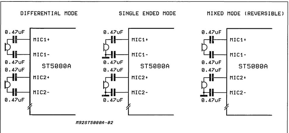
The 4 connection modes (since the MIXED MODE is symmetrical with respect to MIC1 and MIC2) allow one microphone at a time to be selected via the V<sub>S</sub> bit (bit 7 of Control Register CR4).
