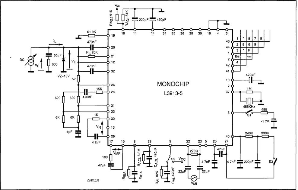
Figure 6: DTMF Distortion French Specification.
