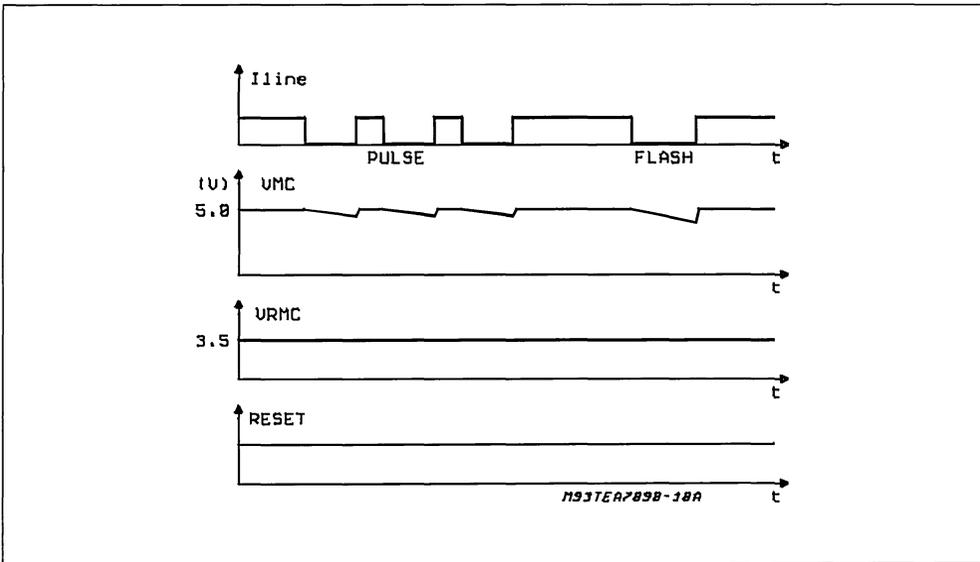
**Figure 9: Timing Without Use Microcontroller Reset Code Control**
