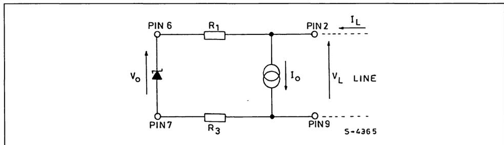
Figure 6 : Circuit Configuration of the Shunt Regulator.
