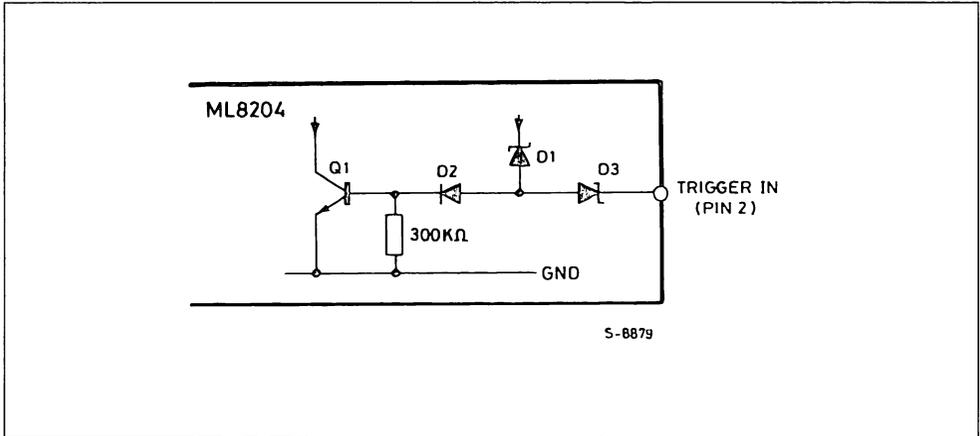
Figure 5a : Enabling Oscillation of the ML8204 for Supply Voltages less than  $V_{SI}$ .Figure 5b : Reducing the Effective Value of  $V_{SI}$  for the ML8204
