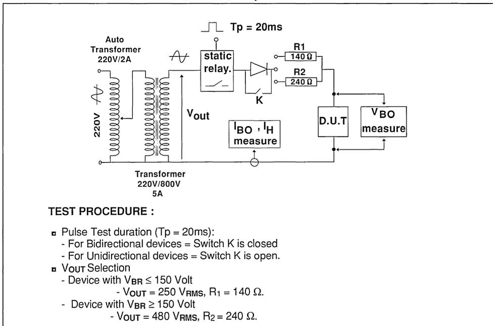
FUNCTIONAL HOLDING CURRENT ( $I_H$ ) TEST CIRCUIT = GO - NOGO TEST
