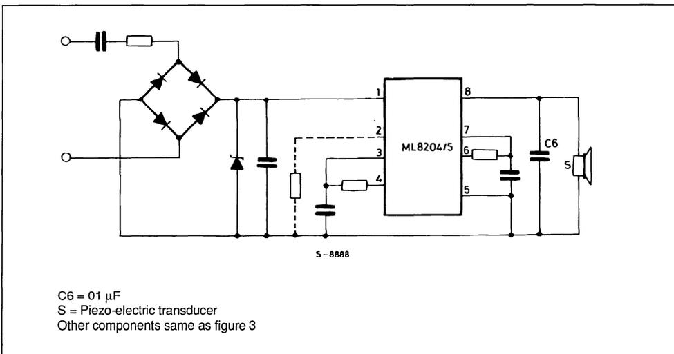
Figure 15 : ML 8204 Circuit to Eliminate Tail-off.
