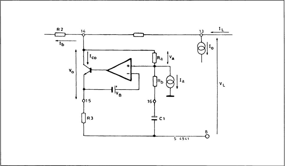
Figure 7 : Two to four Wires Conversion.
