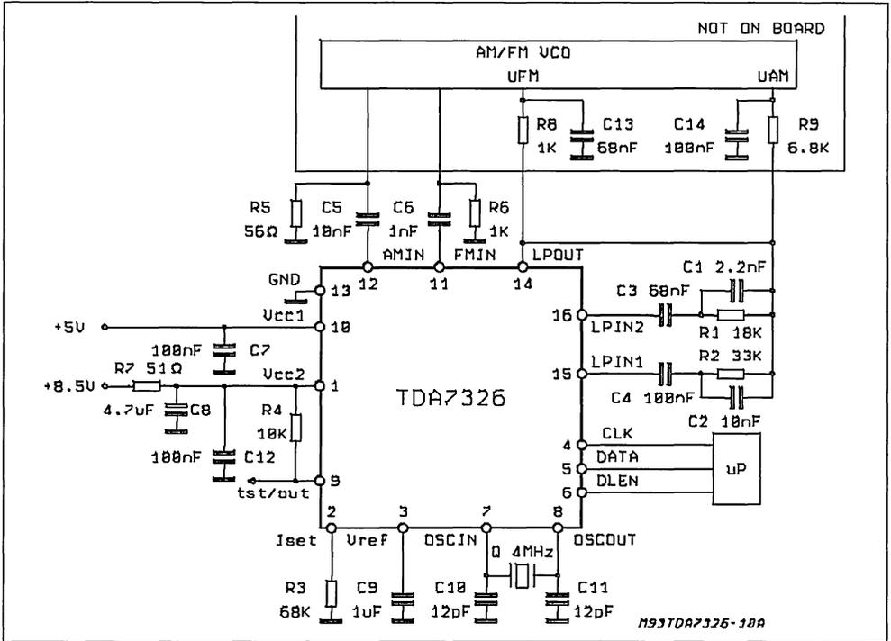
\*) C7 must be connected as closed as possible between pin 10 and pin 13
