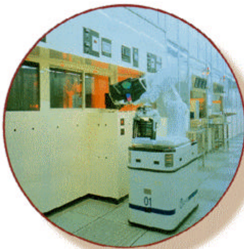
To ensure future foundry capacity, in October 1995, Xilinx entered into a joint venture with UMC, a wafer fabrication facility in Taiwan. At left, UMC uses robots to automatically transport 8" wafers, thereby reducing manual intervention.
