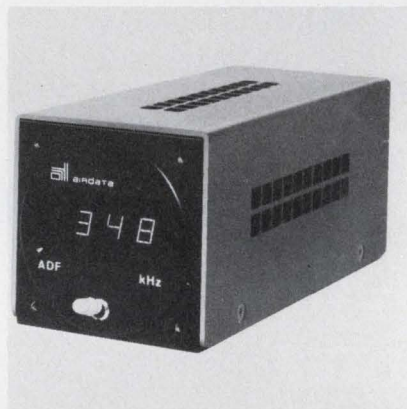
This independent display unit substitutes for the tuning dial of a standard aircraft ADF receiver.
