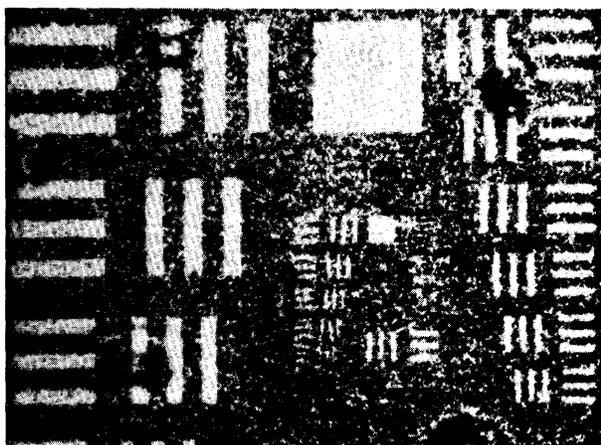
Figure 4. Photograph in reflected coherent light.
